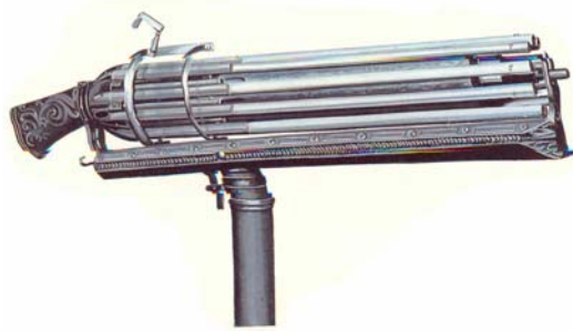
Figure 23: 17th Century Gun with 9 barrels
