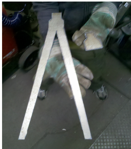
Figure 38: Finalized knuckle guard cutouts.
