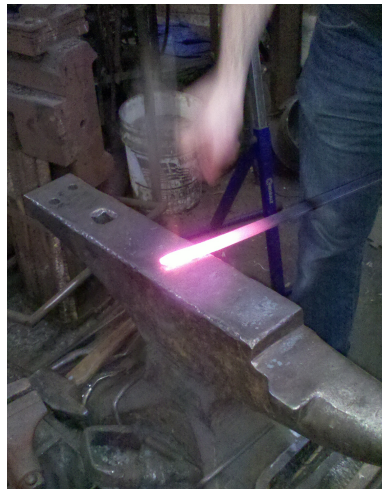
Figure 23: Peening the blade.
