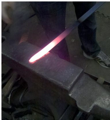
Figure 22: Furnace heated steel on the anvil.
