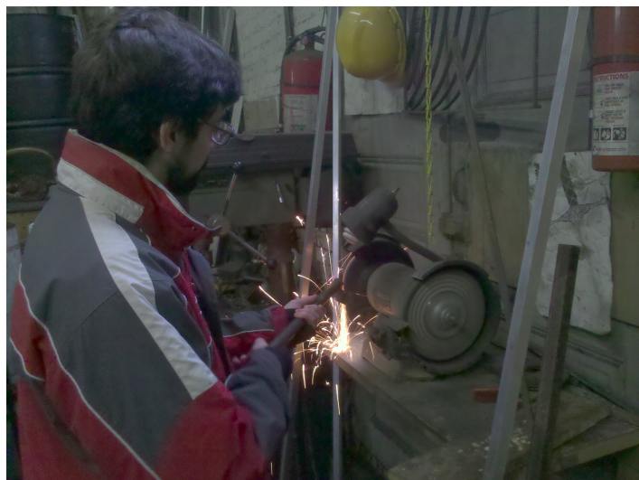
Figure 40: Preparing the pommel for forging.
