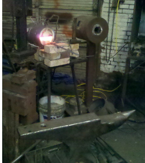
Figure 21: Blacksmith's work area with the blade heating in propane furnace.
