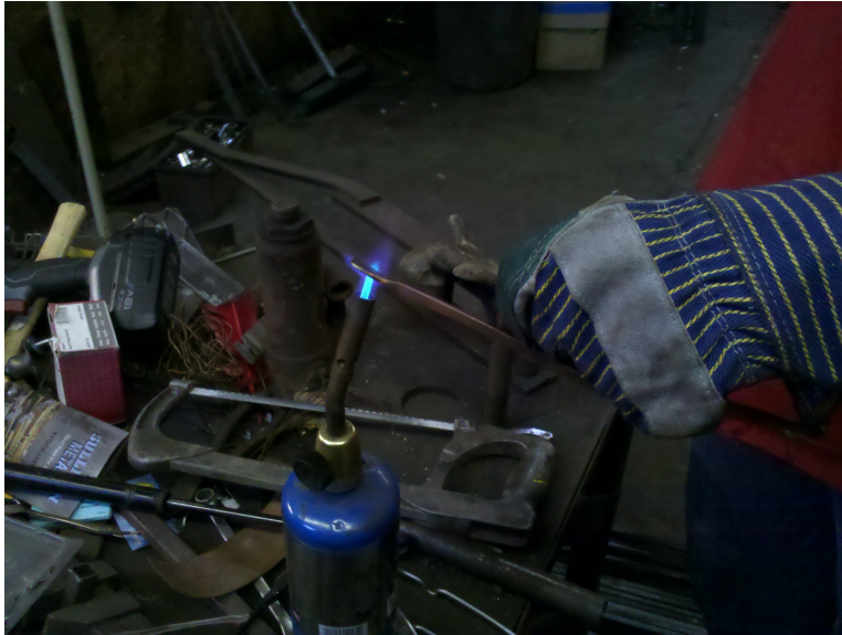
Figure 32: Annealing of the crossguard.
