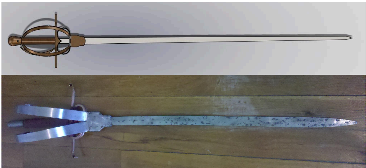
Figure 38: Comparison of the CAD model rapier (top) and the hand manufactured rapier (bottom).
