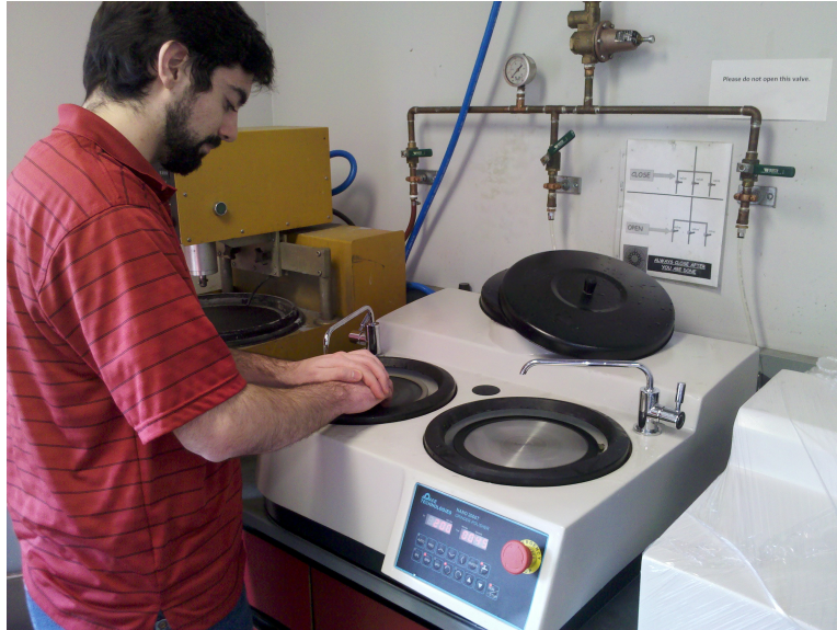
Figure 39: Preparing the sample surfaces to be viewed under the microscope.
