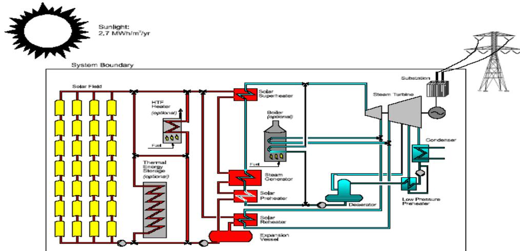
Figure 1. Solar/Rankine parabolic trough system schematic [1].
