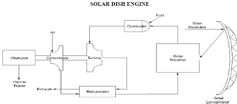
**Figure 44: Solar Dish Engine**
