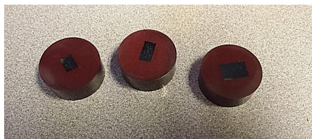
Figure 32. Sample Pieces After Mounting and Polishing.
