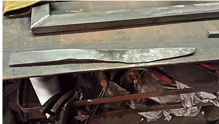
Figure 24. Rough Blade Portion Finished, Tang Next to be Worked on.
