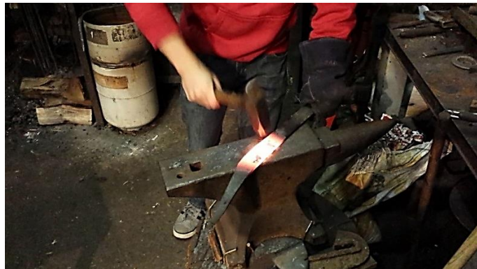
Figure 23. Connor Hammering the Blade Edge of the Steel Replica.
