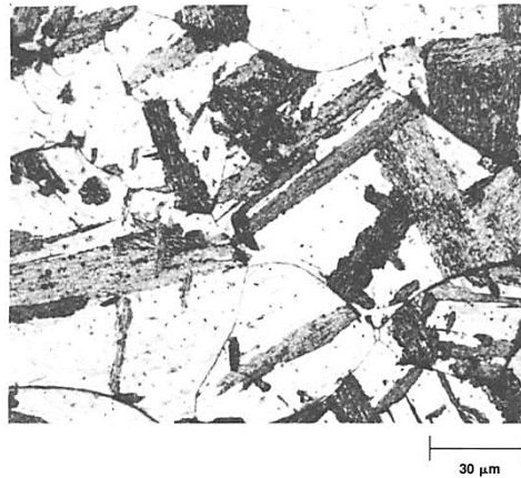
Figure 35. Light Micrograph Showing Upper Bainite (Dark) Formed in 4150 steel. [33].
