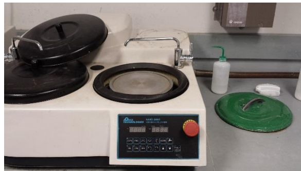
Figure 30. Grinding Machine Used in Polishing of Samples.
