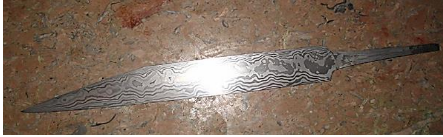
Figure 10. Varying Steel Compositions within Blade.
