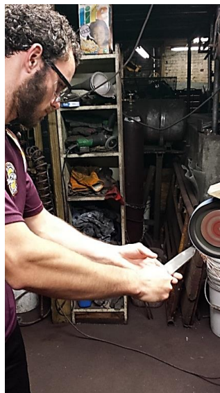
Figure 22. Grinding the First Replica into the Rough Shape.
