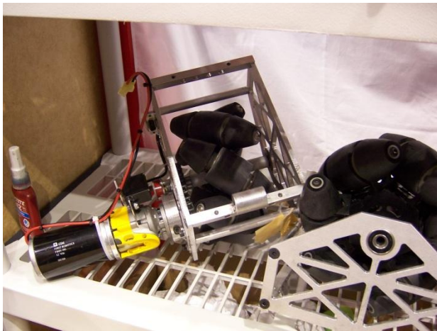
Figure 44 – Mecanum Wheel Pod
