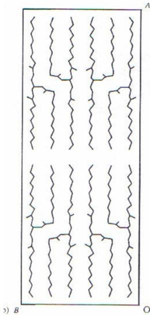
**Figure 4: Crystal Packing for  $\beta'$  structure perpendicular to ab-plane<sup>8</sup>**
