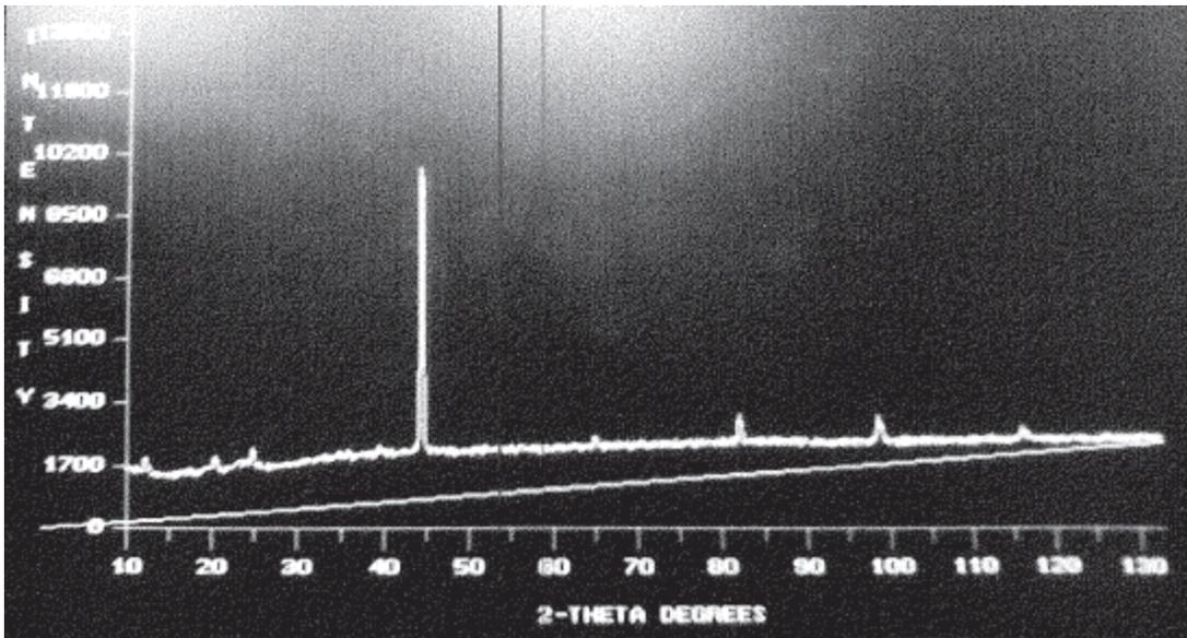
Figure 50: X-Ray Diffraction of Chocolate Sheared at  $50.3s^{-1}$
