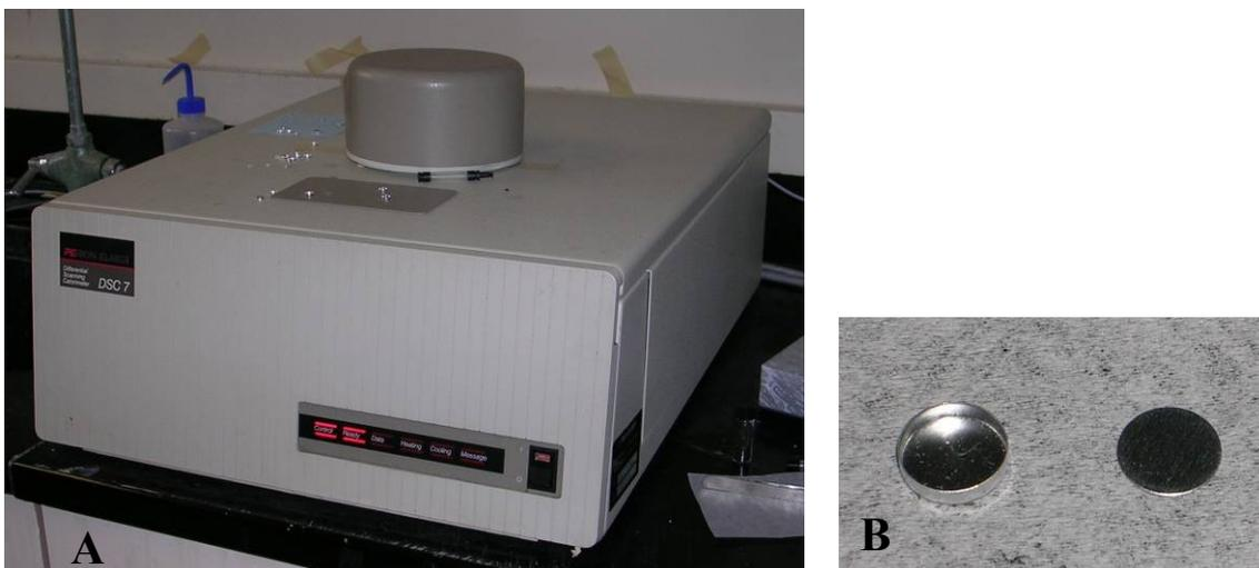
**Figure 21: A) Perkin-Elmer DSC 7 B) Aluminum cup**
