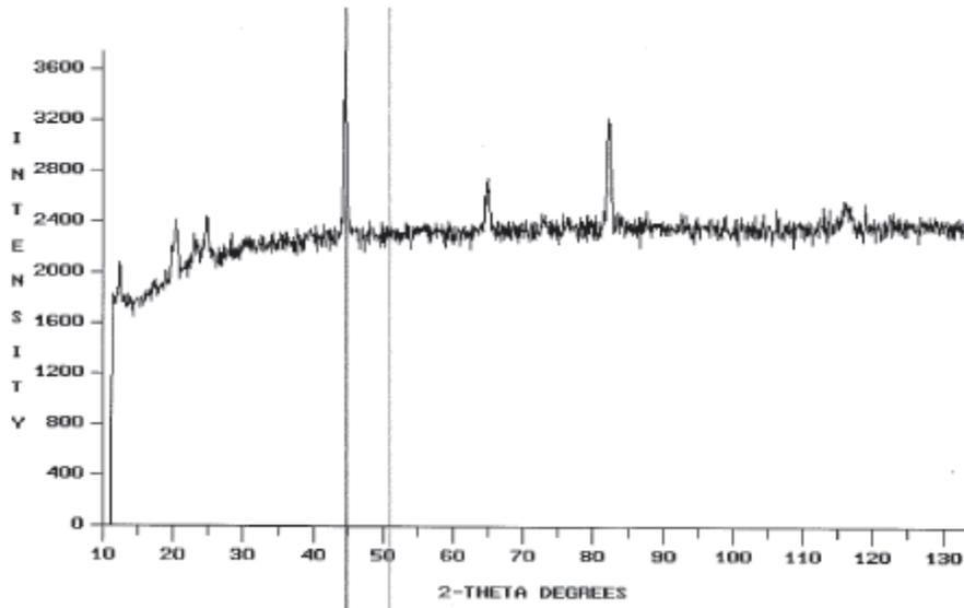
Figure 48: X-Ray Diffraction of Chocolate Sheared at  $29.2\text{s}^{-1}$
