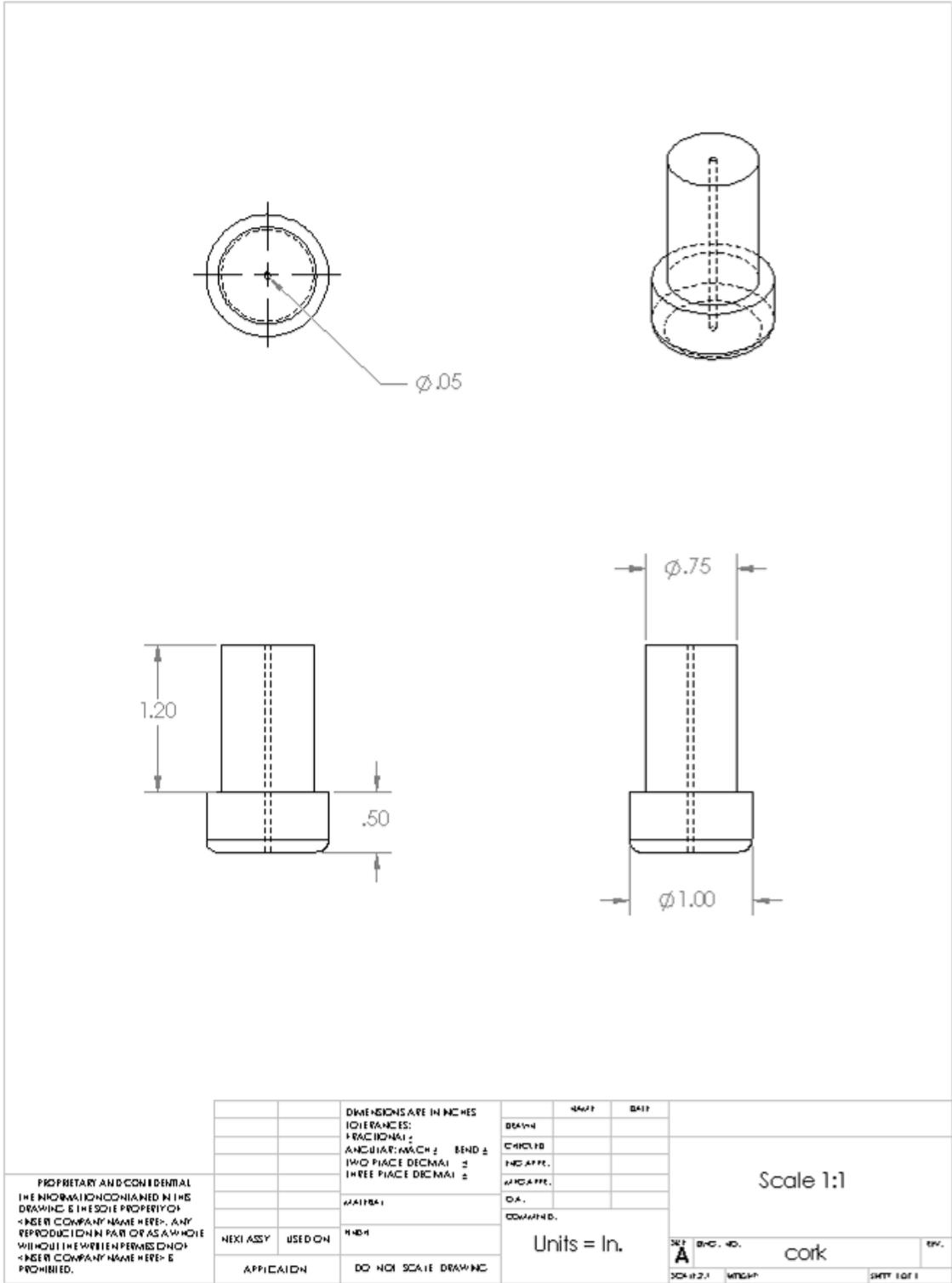
Figure 17: CAD Drawing of cork top
