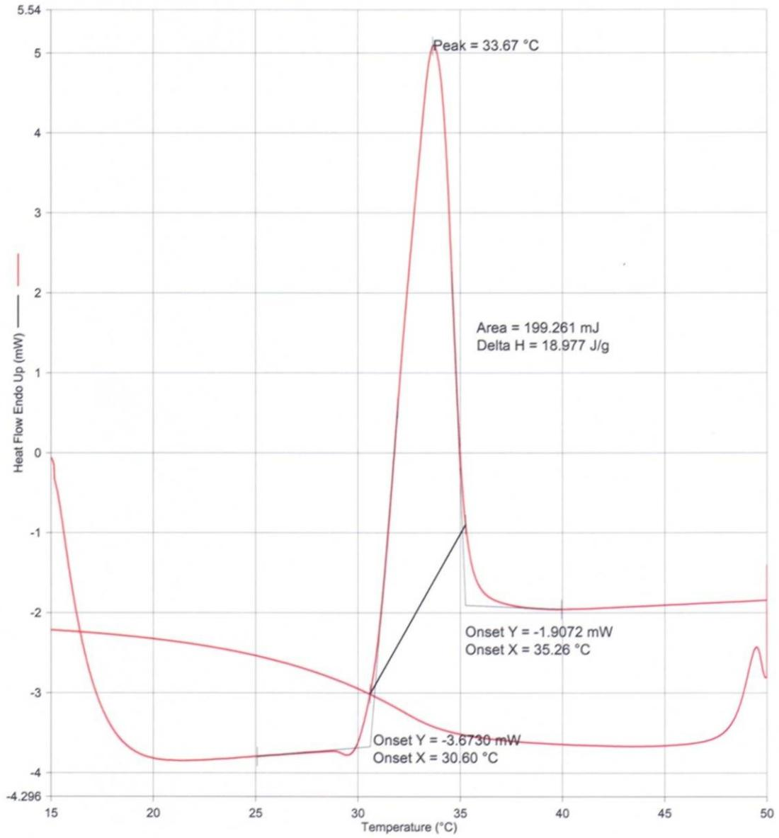
Figure 36: DSC data for shear rate  $10.5s^{-1}$  (Heating rate of  $5^{\circ}C/min$ )
