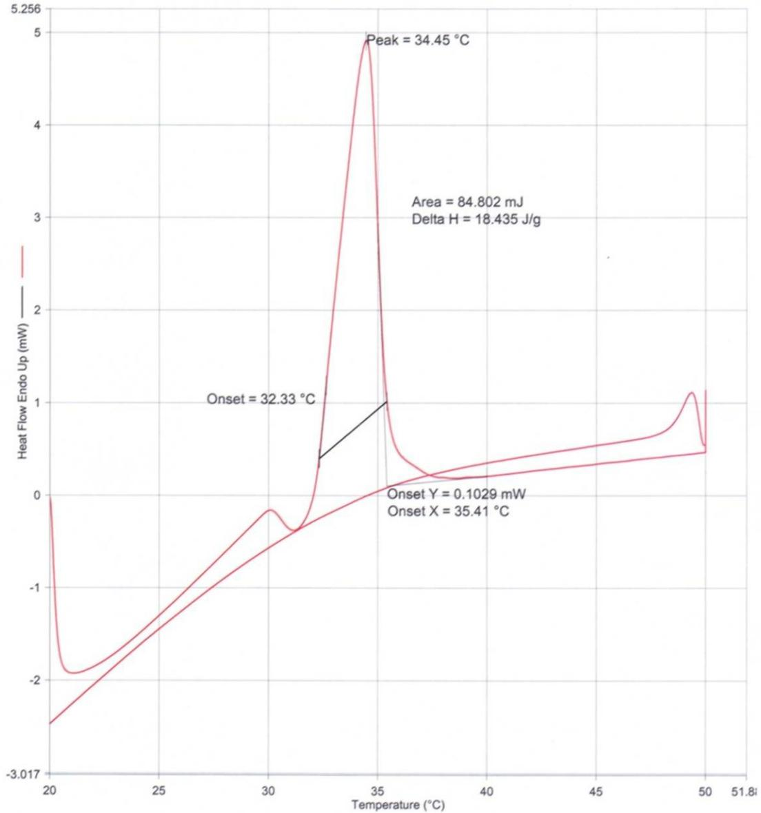
Figure 35: DSC data for unsheared chocolate (Heating rate of 5°C/min)
