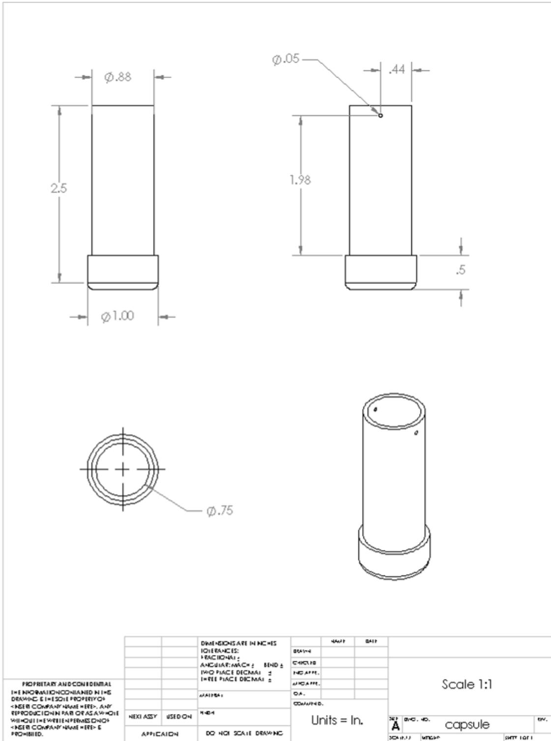
Figure 16: CAD drawing of copper capsule
