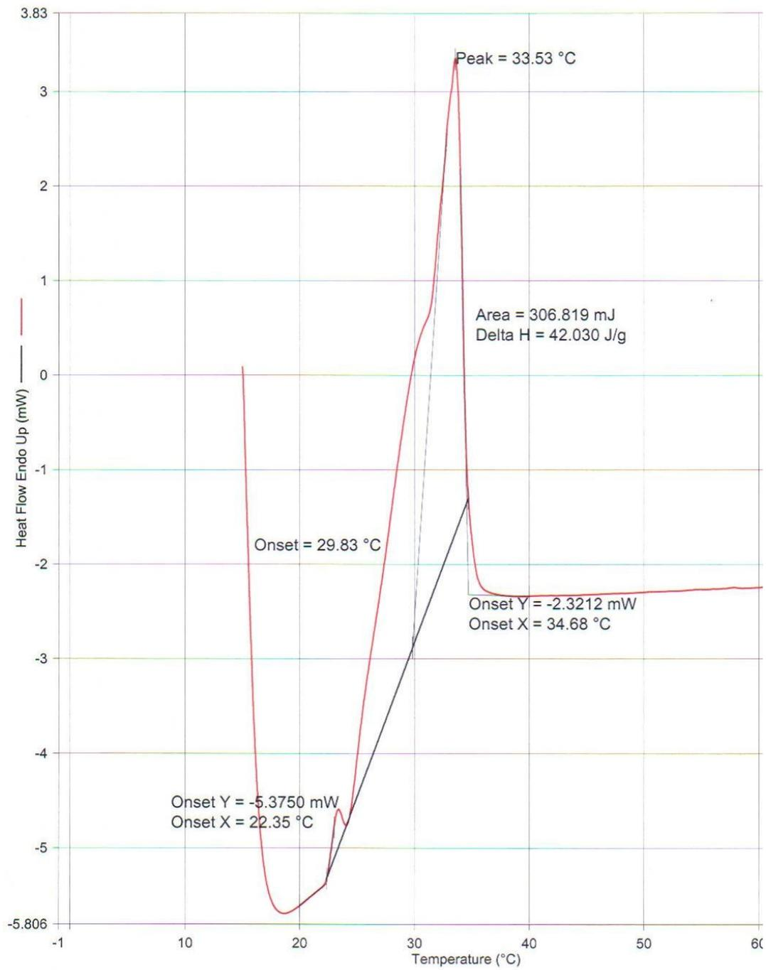
Figure 38: DSC data for shear rate  $29.2s^{-1}$  (Heating rate of  $5^{\circ}C/min$ )
