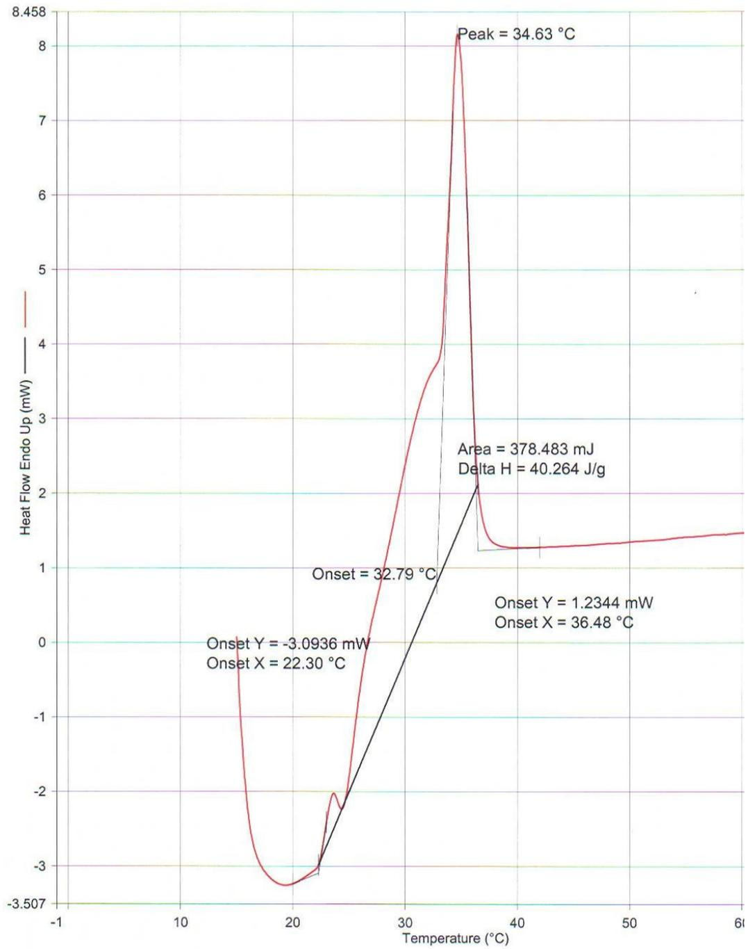
Figure 39: DSC data for shear rate  $40.5s^{-1}$  (Heating rate of  $5^{\circ}C/min$ )
