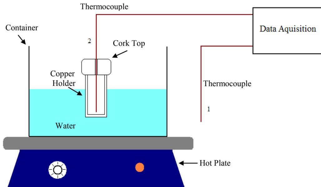
**Figure 20: Set up for Thermocouple Procedure**
