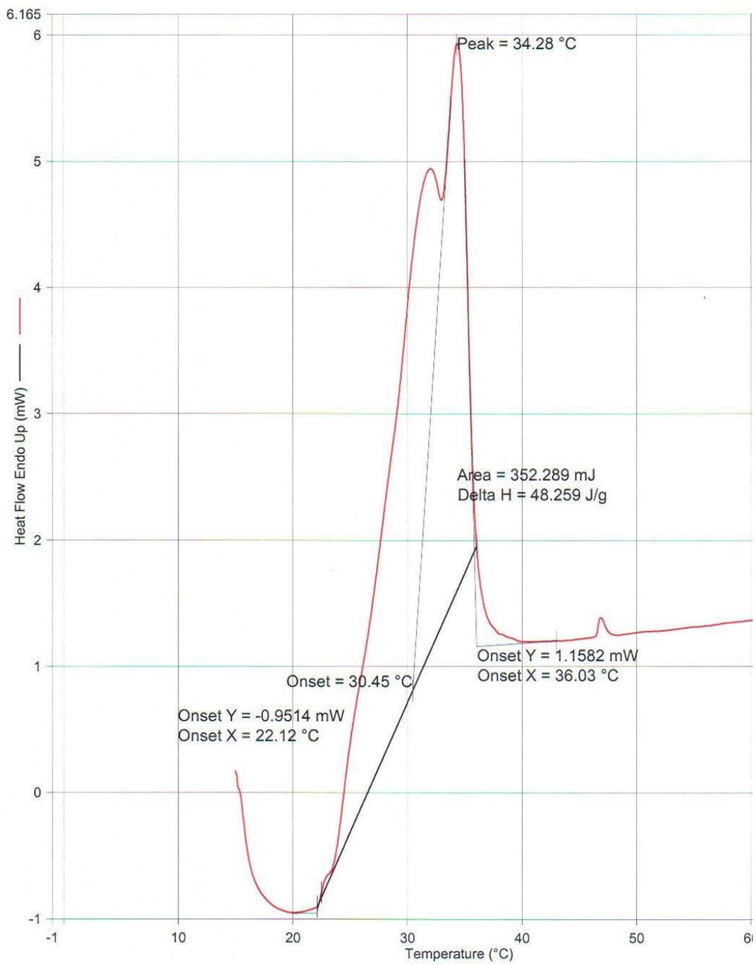
**Figure 40: DSC data for shear rate  $50.3s^{-1}$  (Heating rate of  $5^{\circ}C/min$ )**
