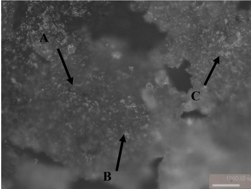
**Figure 29: Chocolate sheared at 40.5 s<sup>-1</sup> showing various crystal sizes (Arrows A, B, & C)**
