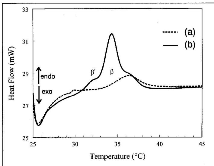
**Figure 7: DSC Recording of Dark Chocolate during a) first and b) second steps of the crystallization process<sup>15</sup>**
