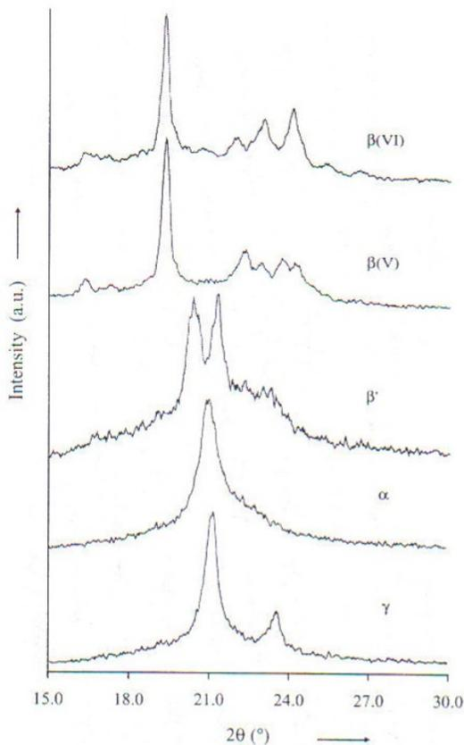
**Figure 6: XRPD Diffraction Example of Cocoa Butter<sup>8</sup>**
