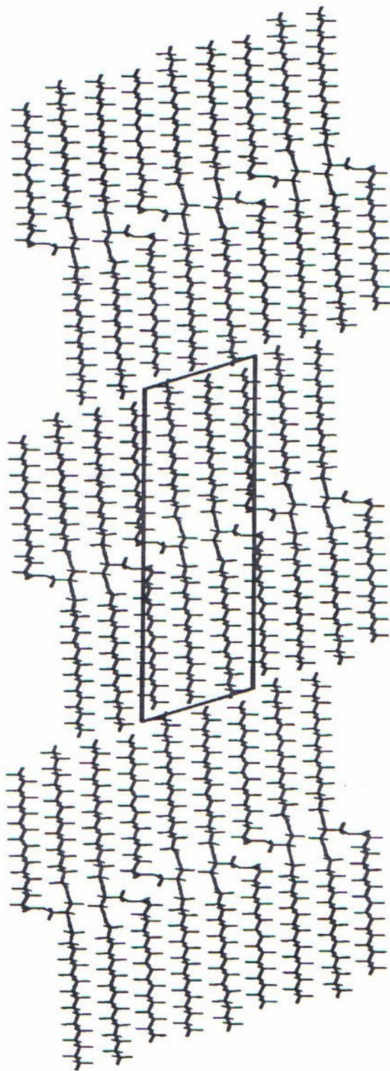
Figure 3: Crystal packing of  $\beta$  structure with  $c$ -axis perpendicular to the plane of the paper<sup>8</sup>
