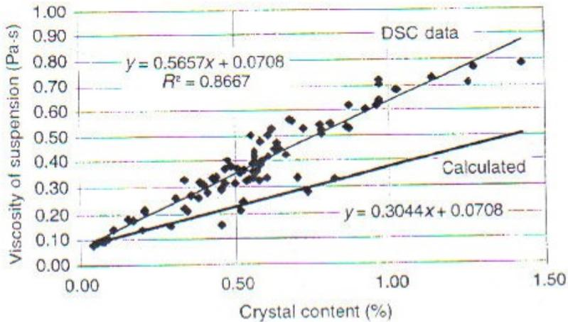
**Figure 13: Viscosity as a function of crystal content %**
