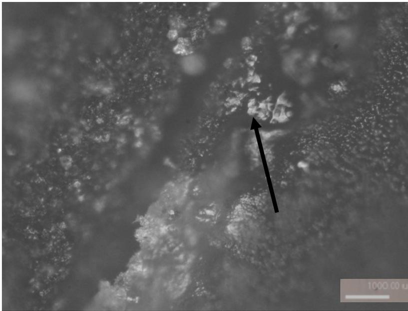
**Figure 27: Chocolate sheared at  $29.2\text{ s}^{-1}$  shows increased crystal size (Shown by Arrow)**
