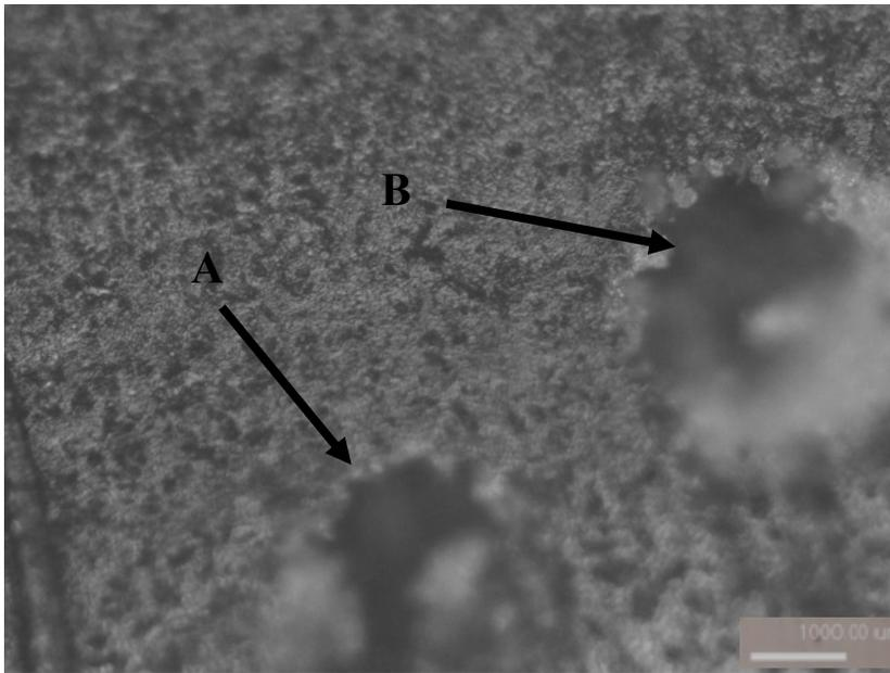
**Figure 24: Chocolate sheared at  $10.5 \text{ s}^{-1}$  (uncut) depicting craters along the surface (Shown by Arrows A & B)**
