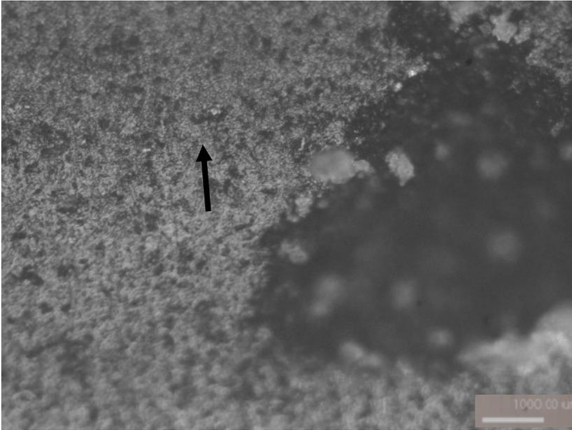
**Figure 26: Chocolate sheared at  $20.3 \text{ s}^{-1}$ ; Arrow shows the even cocoa crystals across surface of chocolate**
