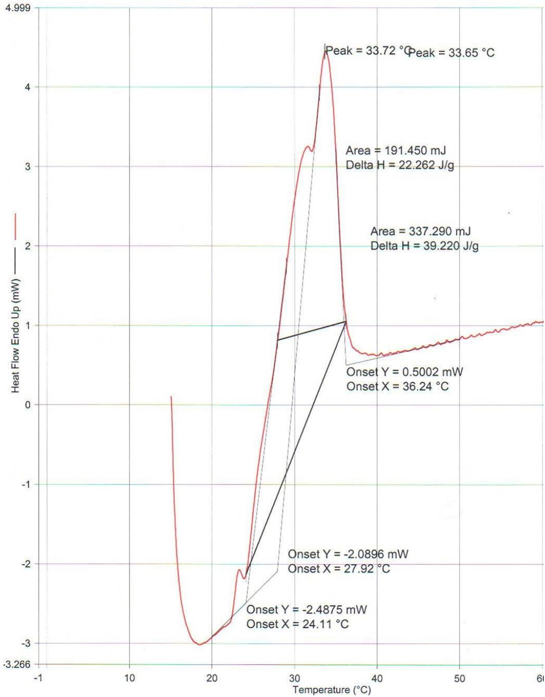
Figure 37: DSC data for shear rate  $20.3s^{-1}$  (Heating rate of  $5^{\circ}C/min$ )
