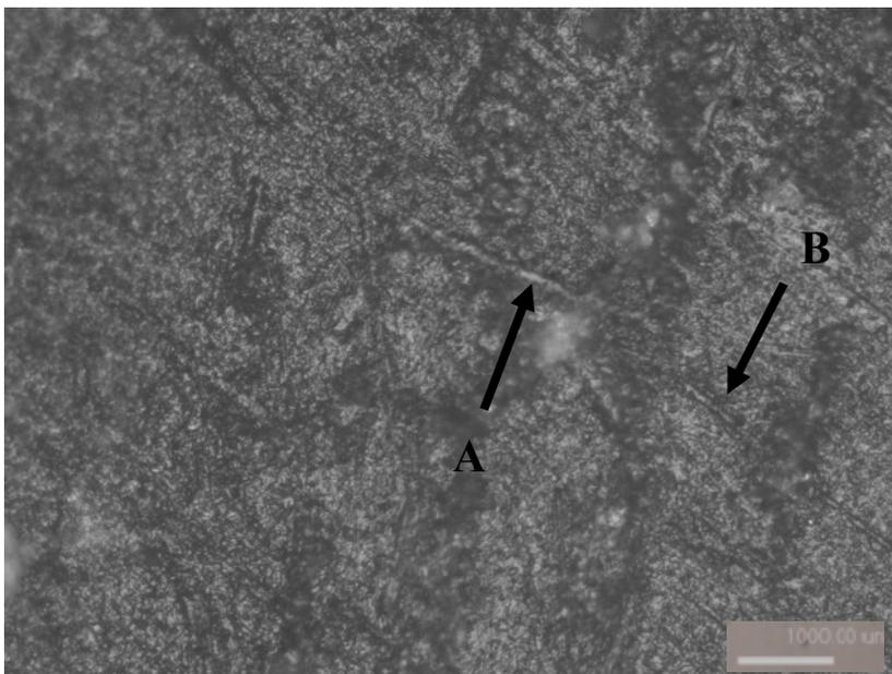
**Figure 28: Chocolate sheared at  $40.5\text{ s}^{-1}$  showing lacerations (Arrows A & B)**
