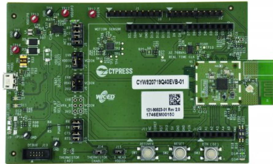
Figure 2.9: Picture of the CYW20719 evaluation board [21]. The micro-USB connection used to communicate with a computer is on the left, the buttons and user-controllable LEDs are in the bottom right, and the CYW20719 and built-in antenna are on the daughter board on the right.
