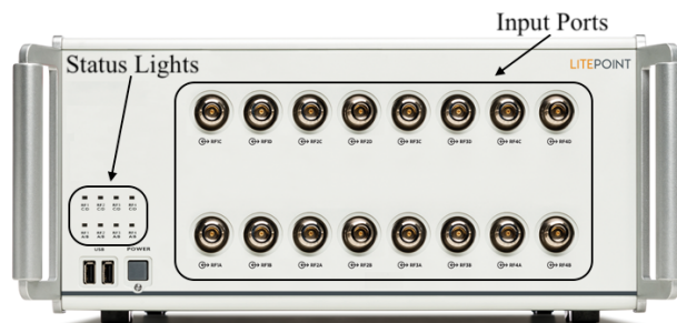
Figure 5.1: Image of Litepoint IQxel-M16W [13]. Each of the ports on the front can be configured as an input or an output and monitored separately.
