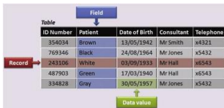
Figure 6: Format of a database table showing the records, fields, and data values. Source: https://doi.org/10.1016/j.mpaic.2013.12.002
