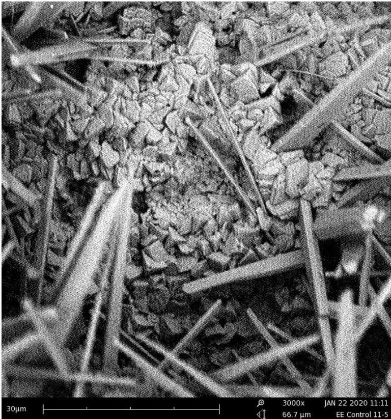
Calcium carbonate repair crystals:
