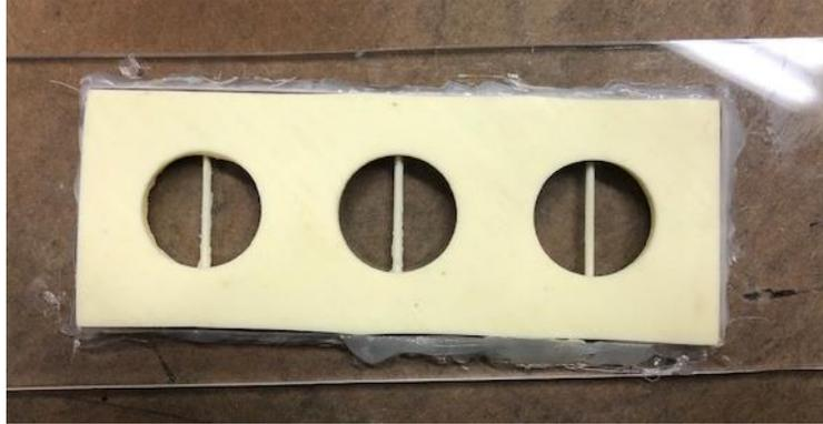
**Figure 6:** The silicon mold used to make concrete samples with a small v-shaped notch. Samples were used for SEM. Three cylinders were put in each mold for efficiency and ease in demolding.
