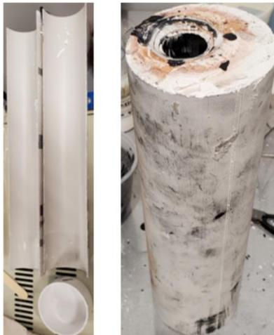
Figure 4.32: Three-part case mold and plaster mold produced with it.
