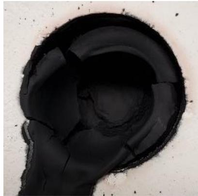
Figure 4.12: An LCM support sample which has cracked in the mold.
