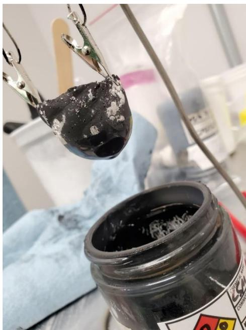
Figure 4.25: An unfired LCM support sample being dip coated. The sample is hung from a holder and the coating bath is raised around it. This method was problematic.
