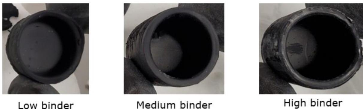
Figure 4.8: Casted supports with varying levels of PVA binder. Note that these samples were made with LSM rather than LCM and did not contain pore former.
