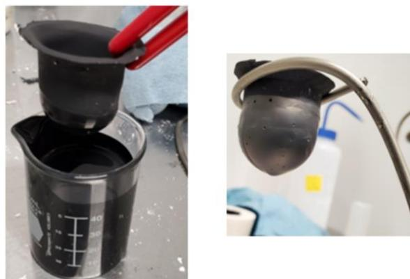
Figure 4.26: The improved dip coating process: the LCM support is dried, then dipped and dried by its flange.
