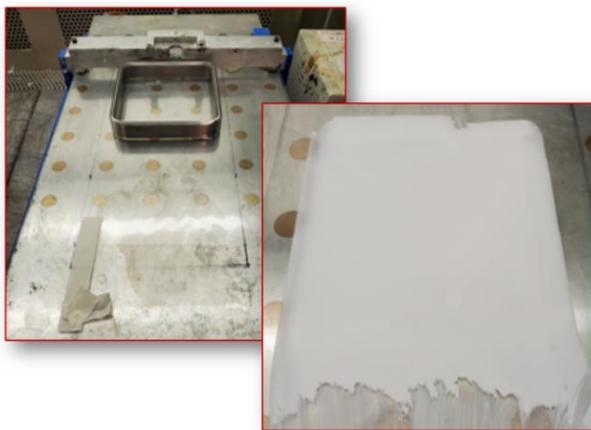
Figure 4.19: Left: the setup used to tape cast the YSZ slurry. Right: The dried YSZ film. This technique was a failed attempt to characterize the porosity of the electrolyte layer without coating it on a complete cell, but was not used in fabrication of the titular structure.
