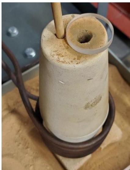
Figure 3.8: Setup used to melt the anode alloy.
