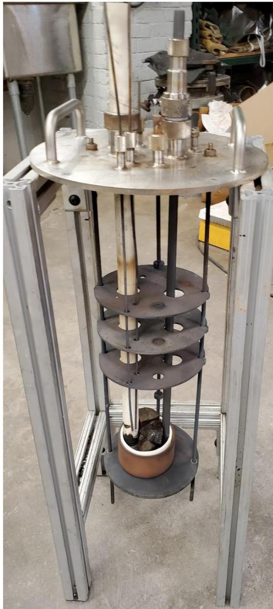
Figure 3.10: Testing insert for which was used to suspend the anode-containing crucible, cathode-electrolyte structure, and graphite fuel rod in the furnace.
