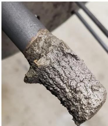
Figure 5.9: The anode current collector post-testing.
