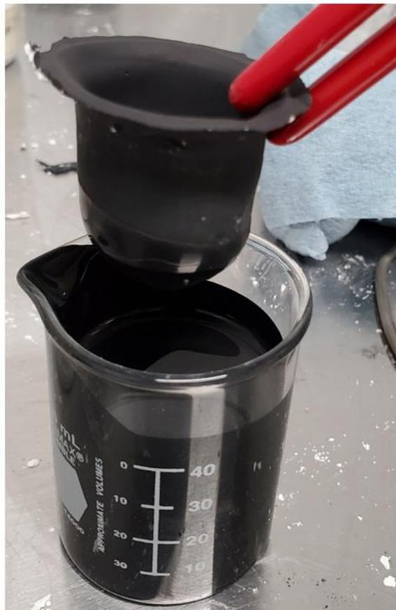
Figure 3.3: A dry support which has just been dip coated with cathode slurry.
