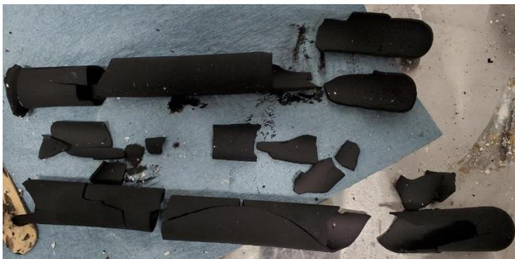
Figure 4.33: Samples casted in the scaled-up mold. They cracked while drying in the mold.
