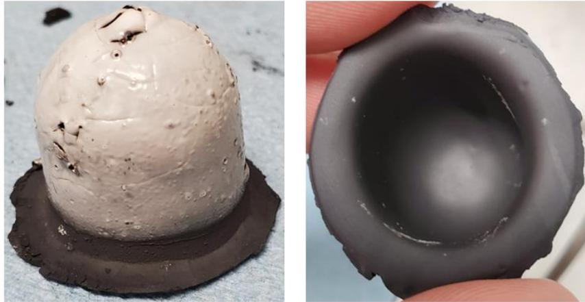
Figure 4.30: Left: an uncracked electrolyte layer. Pinhole defects in the electrolyte are due to entrained air in the slurry. This is the result of firing method 4. Right: the inside of the same sample, showing no cracks in the support.
