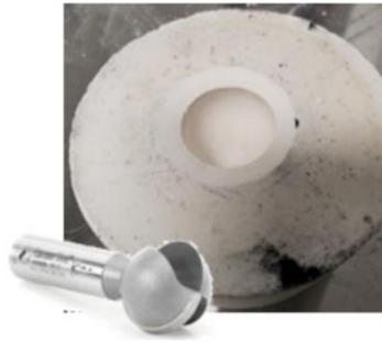
Figure 3.2: Hemispherical-bottomed mold, and the ball-end router tool used to create it.
