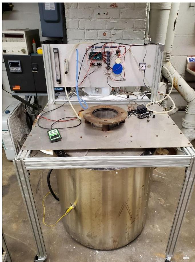
Figure 3.11: The Mellen induction furnace used to test the cell. The testing insert is inserted into the hole. The testing insert's flange is supported by the flange of the furnace tube.
