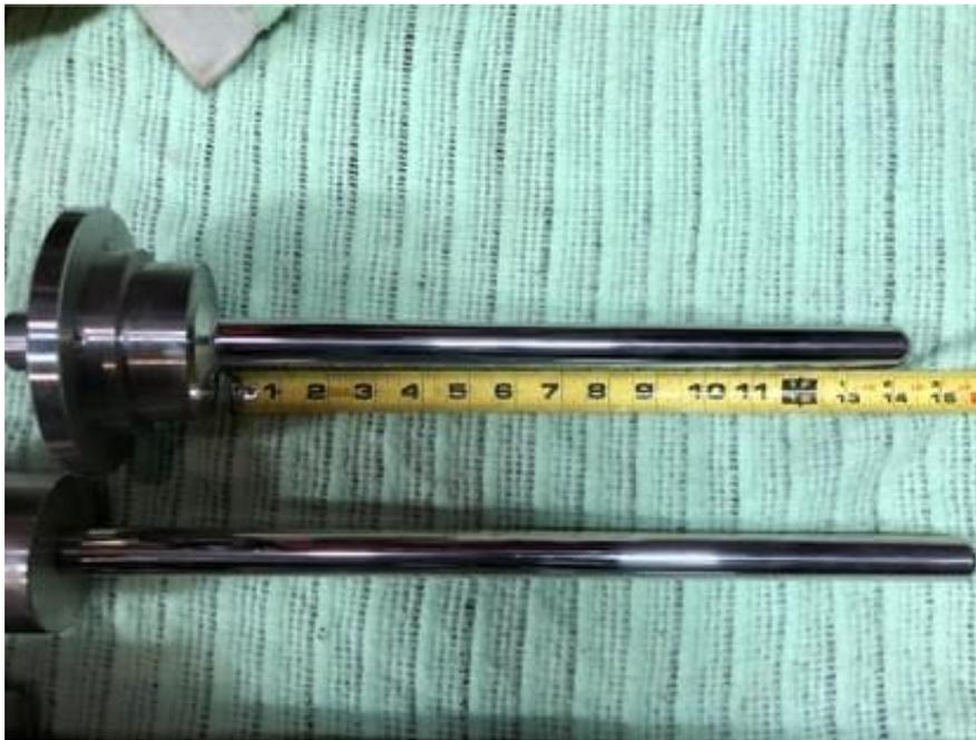
Figure 4.31: Mandrel used for producing scaled-up plaster molds. The mandrel was inserted into wet plaster and removed when the plaster dried.
