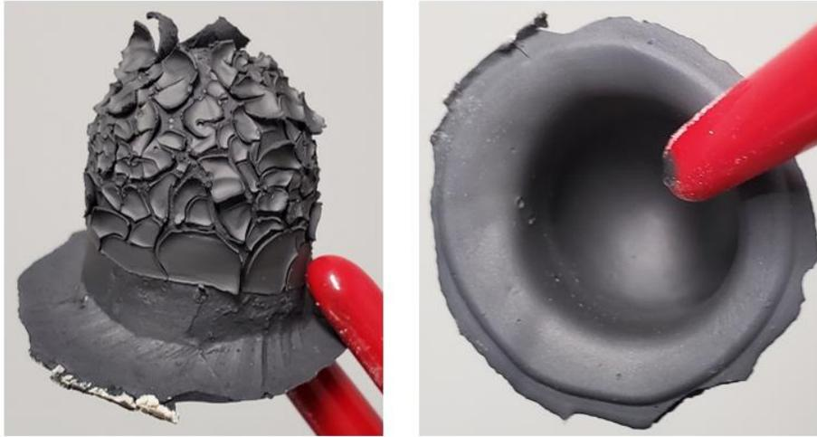
Figure 4.28: The result of firing methods 1 and 3. Left: A cathode layer which has cracked during firing. Right: the inside view of the same sample, showing a support with no significant cracking.
