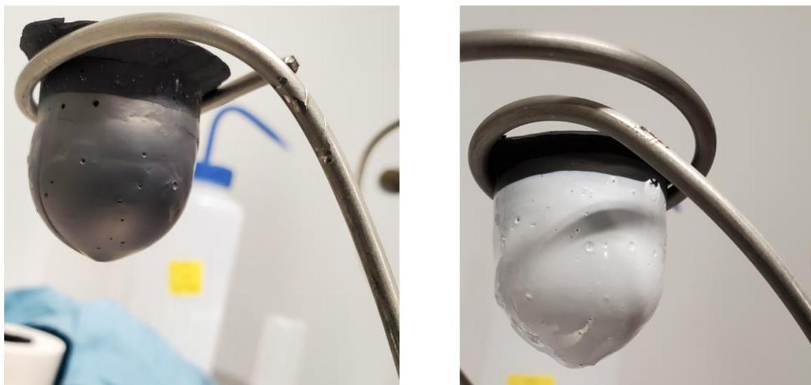
Figure 3.4: Dip-coated samples resting in their holders. Left: a dry cathode coating. Right: a dry electrolyte coating.
