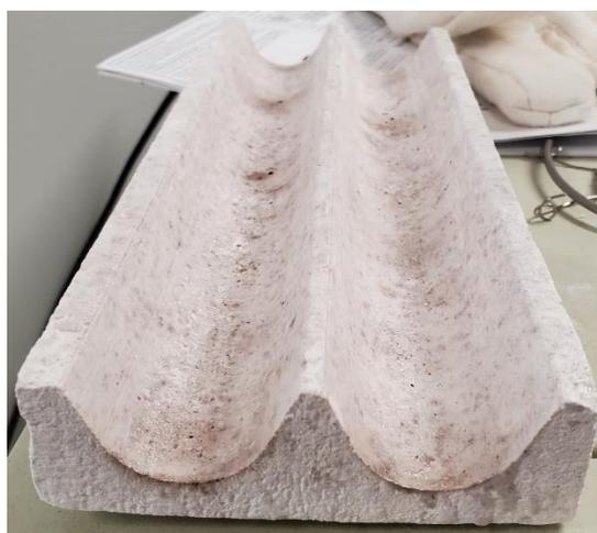
Figure 3.5: Firing trays used to lay-fire samples.
