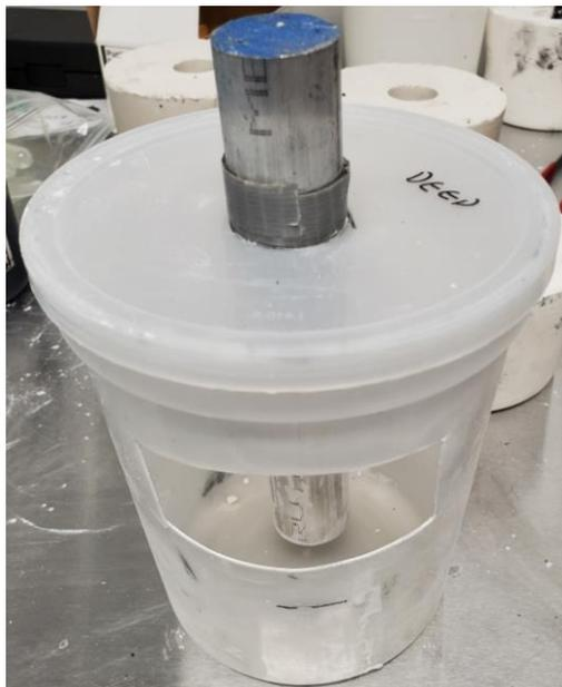
Figure 3.1: Initial setup for creating slip casting molds. The plaster was poured around the suspended rod, and once dry, the rod was removed.
