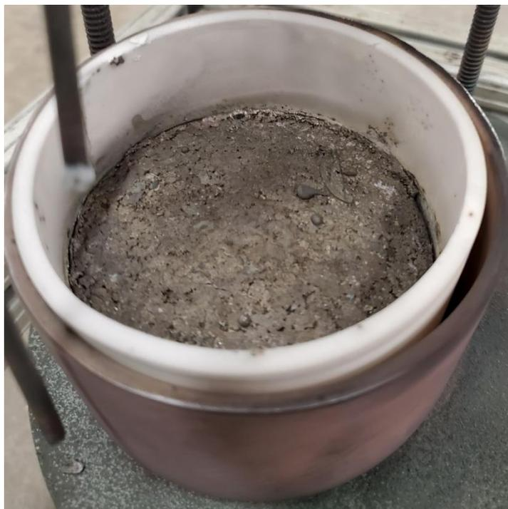
Figure 5.8: Alloy 1 post-testing. Complete melting was achieved.
