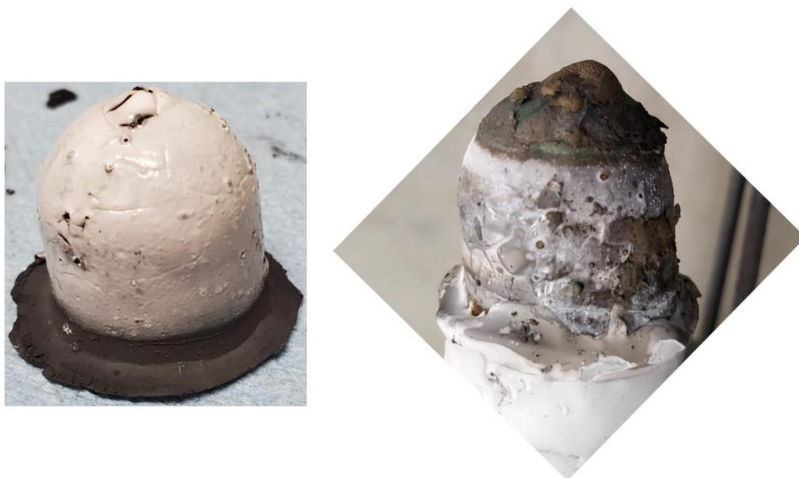
Figure 5.5: Left: cathode-electrolyte structure before testing. Right: The same structure after testing.
