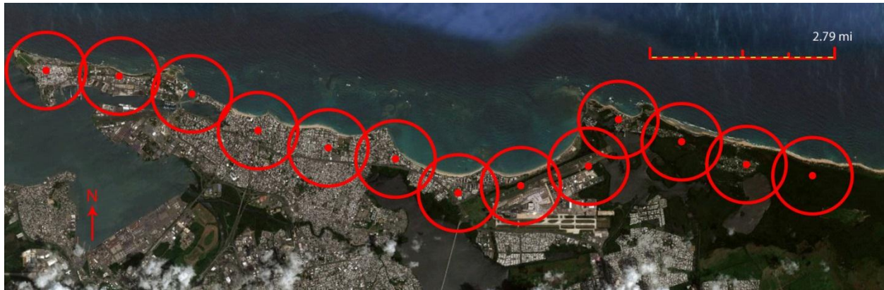
Figure 30: Possible placement of the thirteen 15V2T sirens along the San Juan Metropolitan coastline
