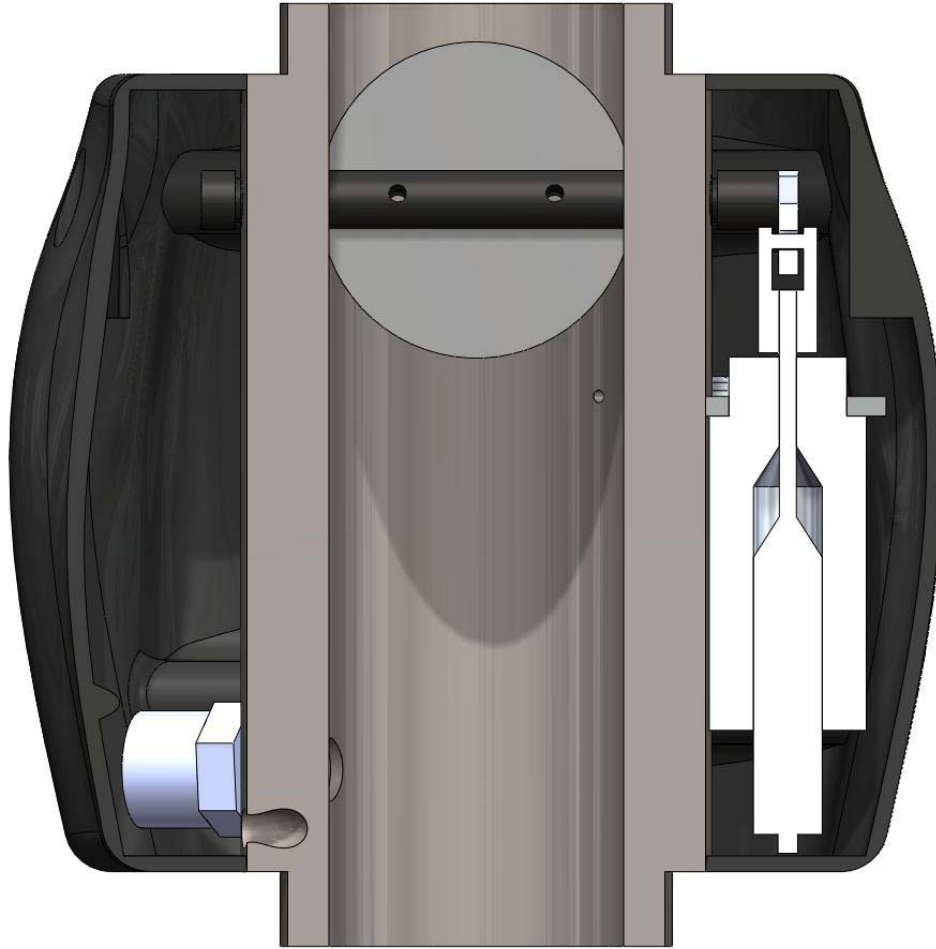
Figure 8-2: Intake System Cutaway
