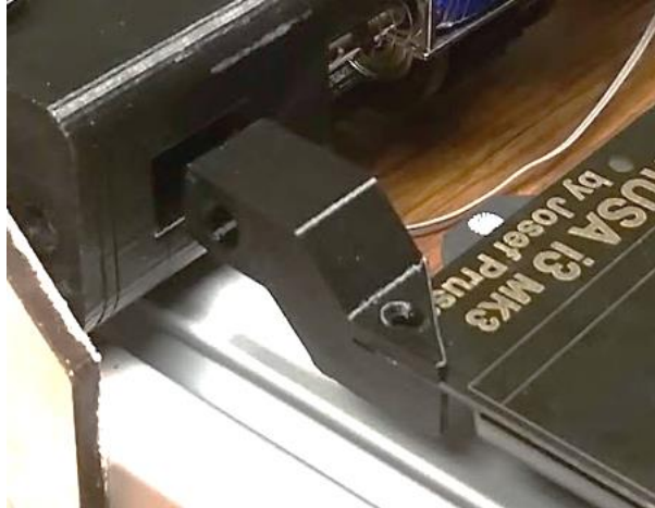
Figure 6: Blocks Permanently Attached to Build Plate
