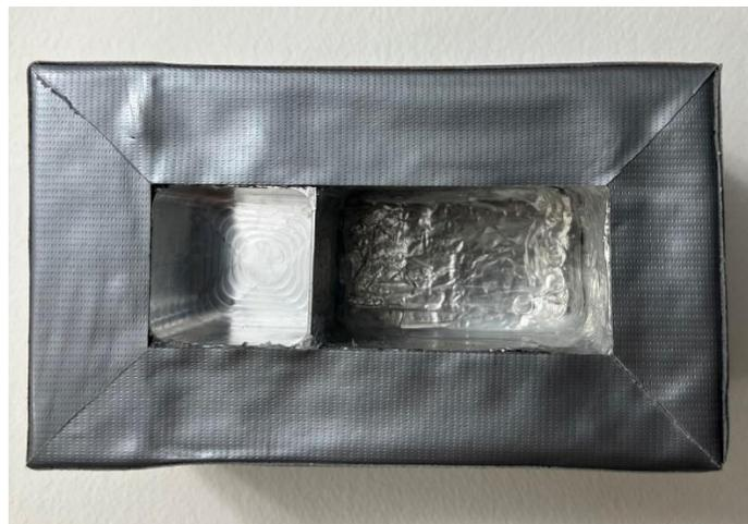
*Note.* The aluminum cube in this model was reused from the prototype's first iteration. Waterproof silicone sealant was used to keep the aluminum cube in place and seal off other portions of the prototype from the dry ice compartment, while the waterproof tape was used to make the inside of the dry ice portion more uniform. The prototype has around 3.81 inches in width and approximately 6.56 inches in length, while all the box's walls are 1 inch thick.
