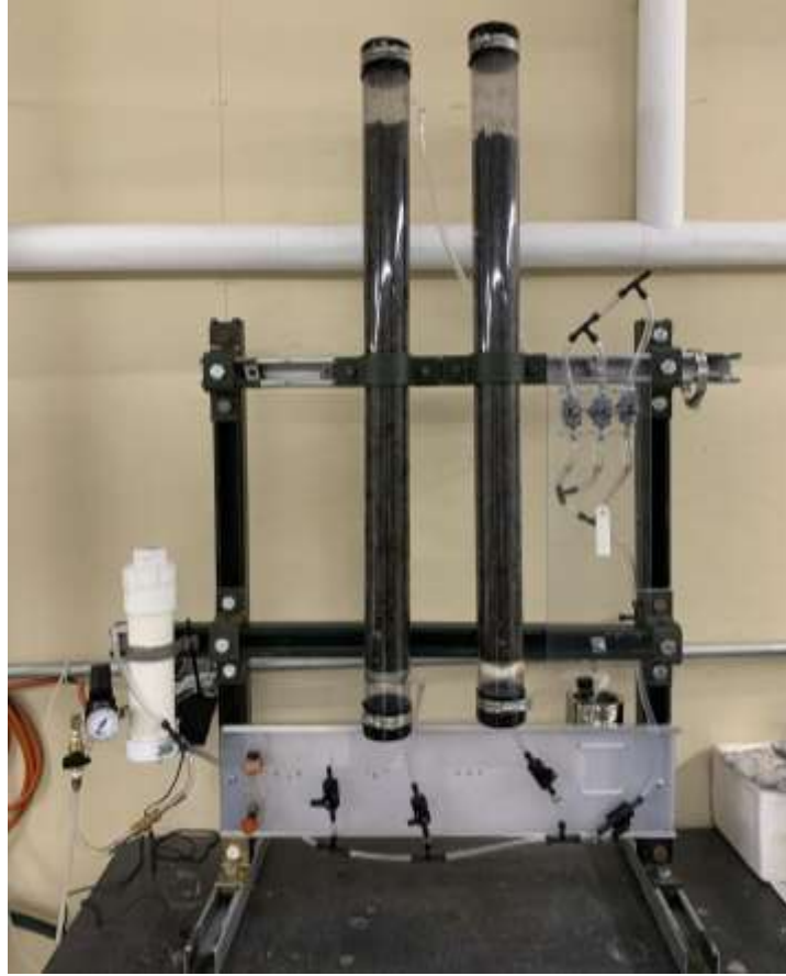
Figure 7. Bench-Scale Biofilter Model. Pictured in Goddard Hall
