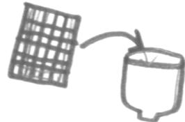
Place the mesh piece in the jug. The piece must cover the entire hole. This is to keep the mosquitoes out.
