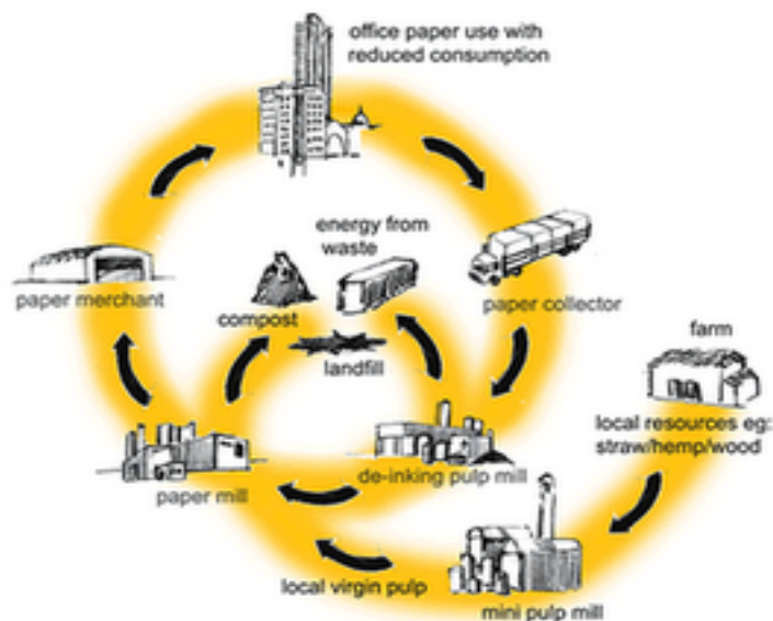
Figure 36: Schematic illustrating the production of paper from renewable resources at BioRegional MiniMills (BioRegional, 2012d)
