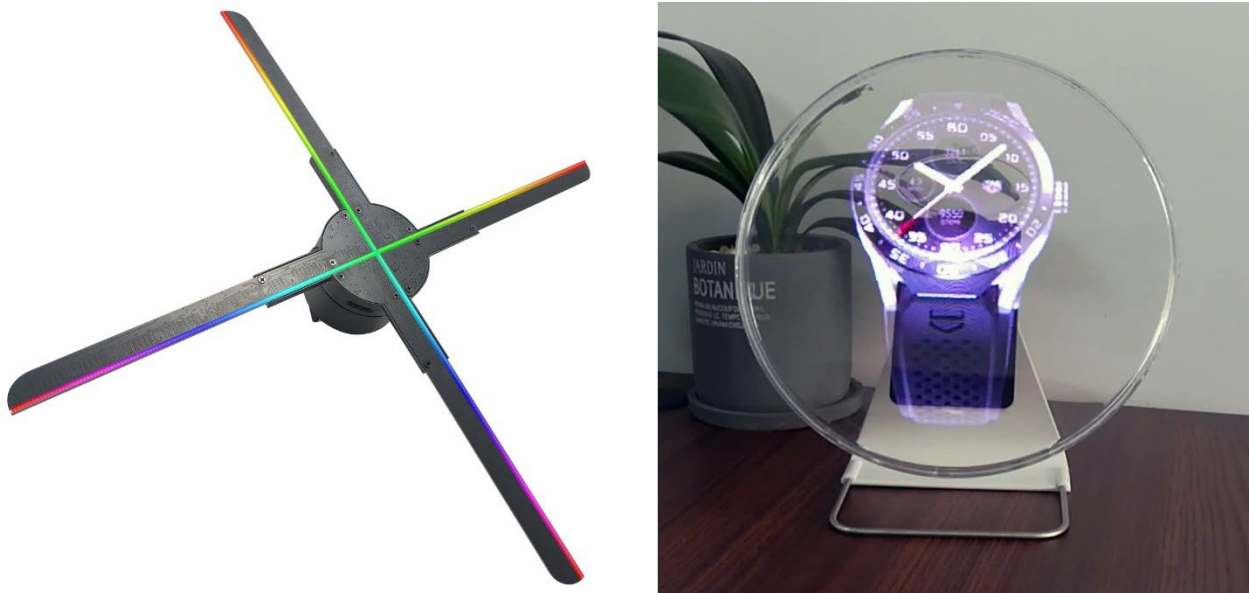
Figure 8. A deluxe 4-bladed 3D fan, and an image produced by a 2-bladed tabletop model. Source: URL .
