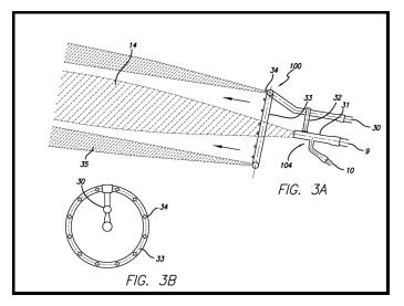
Figure 1: Ichinomiya Circular Nozzle Design of Snowmaking Apparatus and Method
