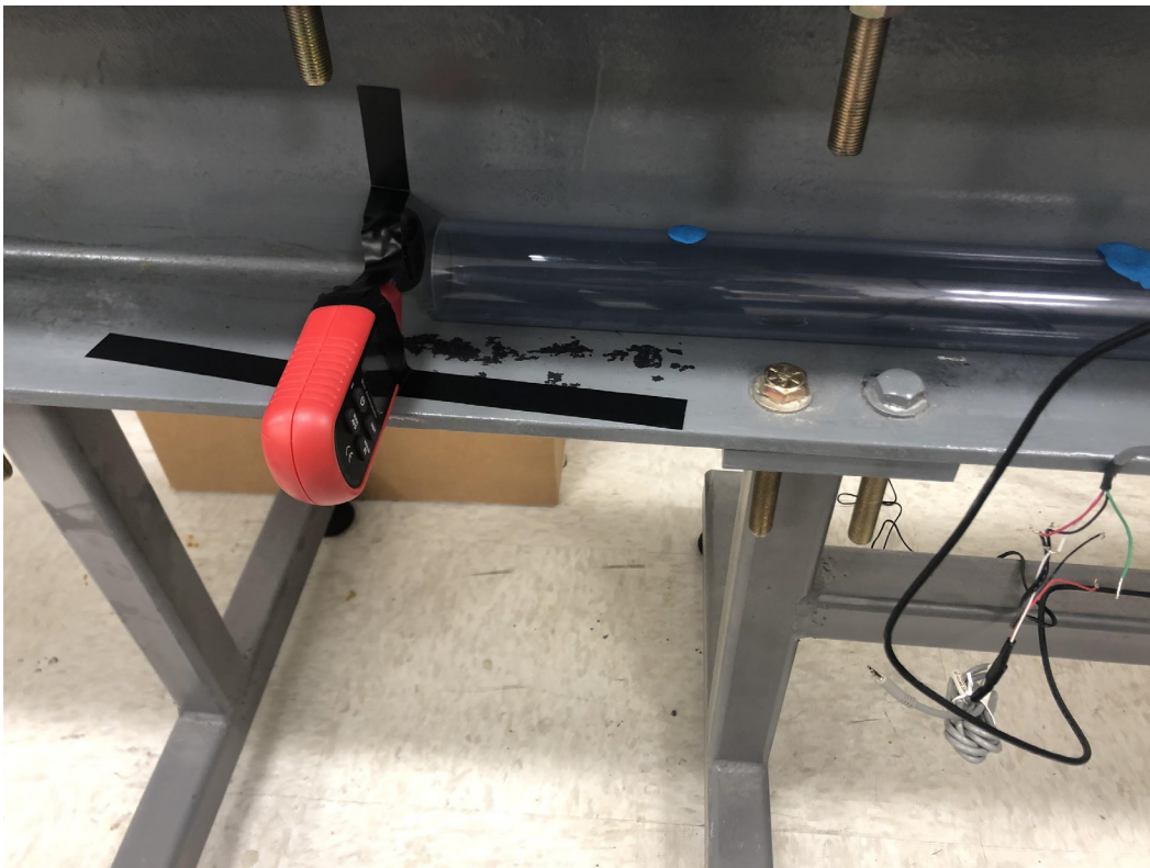
Figure 83: Setup of Mini Anemometer for Velocity Change Experiment
