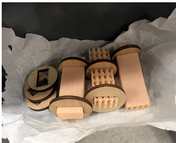
Figure 81: Example of Wooden Holsters Created for Thermal Experiments
