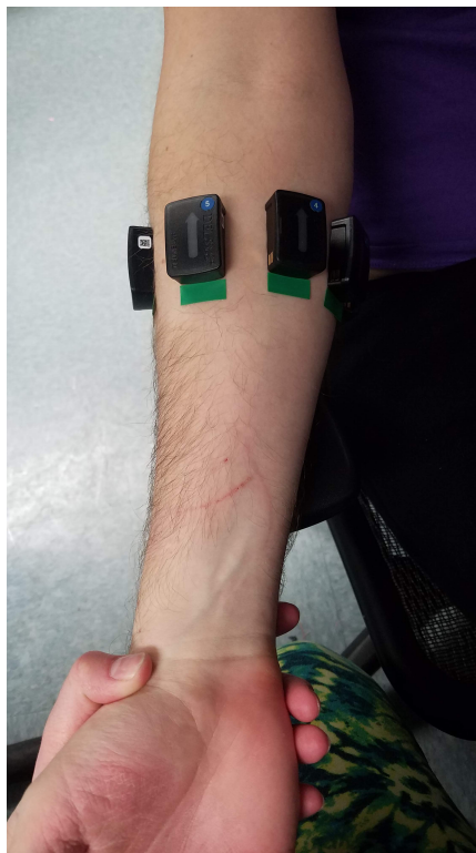
Figure 37: EMG sensors placed band configuration 1 which is when the sensors are placed in an array around the circumference of the forearm
