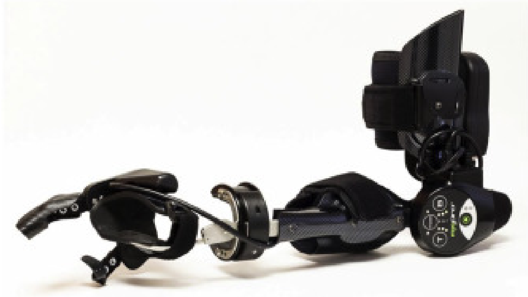
Figure 8: MyoPro by Myomo, Inc. (Cambridge, MA) ; a commercially available powered elbow, wrist, hand wearable assistive device (Peters et al., 2017)
