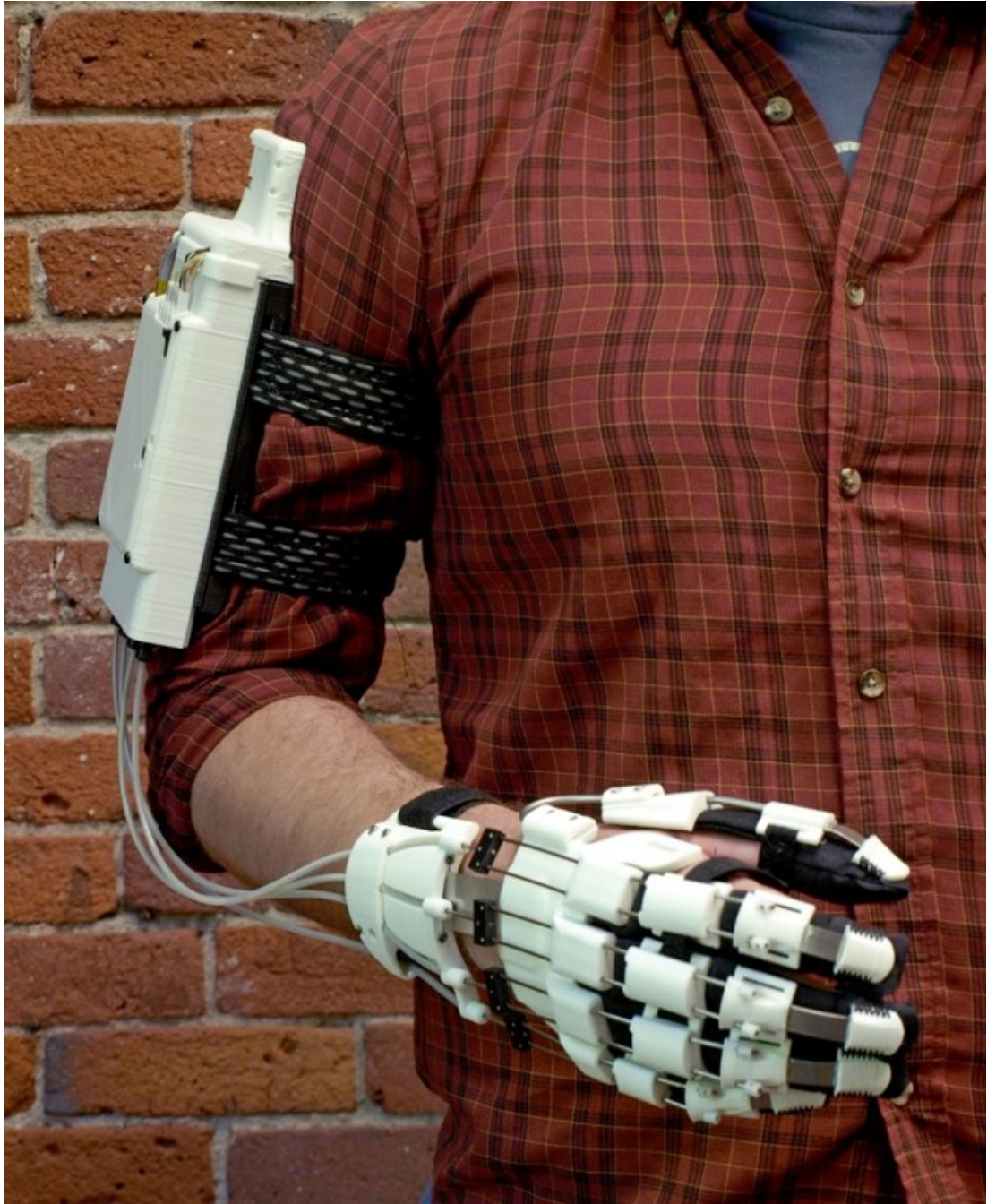
Figure 9: The HOPE (Hand Orthosis for Performing Extension) Hand 1.0 seen in a complete package with the actuation unit on the upper arm and the hand orthosis.
