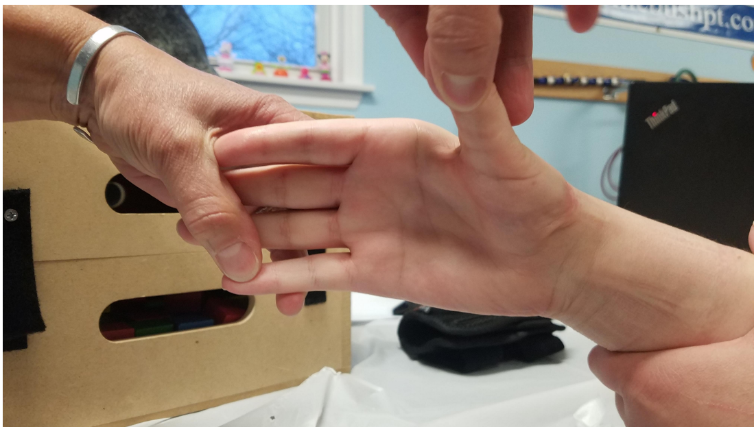
Figure 53: View of the palmar surface of the hand after approximately four hours of wearing the HOPE Hand 2; no irritation marks on the fingers, mild marking around the thumb from wrist brace, barely visible marking on the forearm
