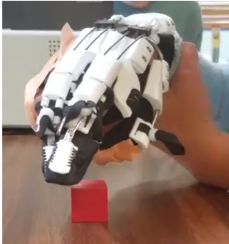
Figure 15: Wrist flexion cause by patient's hypertonia and very little wrist stabilization in the hand exoskeleton design
