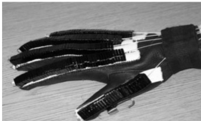
Figure 5: J-glove to perform finger extension for at-home rehabilitation from Saebo which was tested with voice recognition, electromyography, and manual control (Ochoa et al., 2009)
