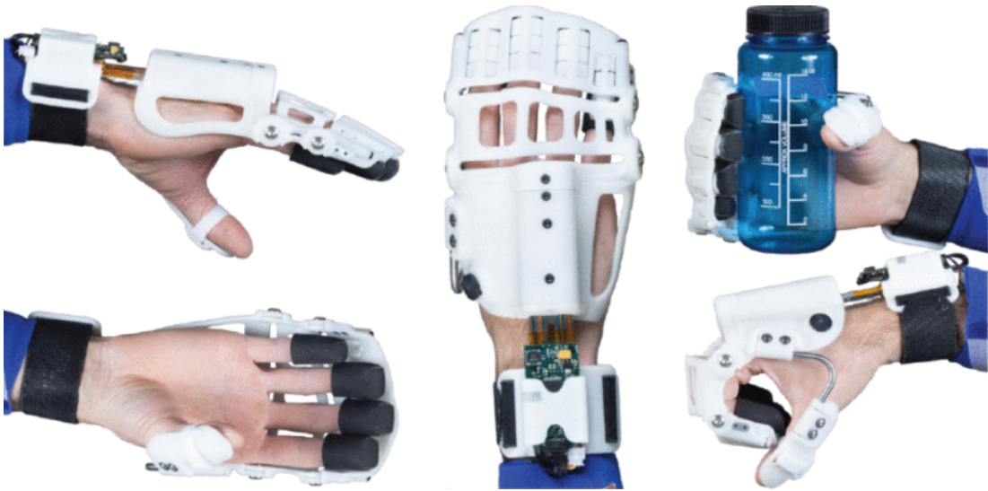
Figure 7: Hand Exoskeleton from Vanderbilt University moves all fingers together for successful power grasping (Gasser et al., 2017)
