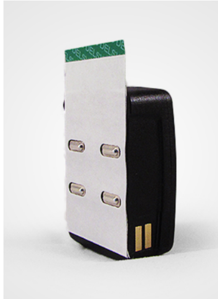
Figure 32: Sensor with adhesive tape for skin adhesion
