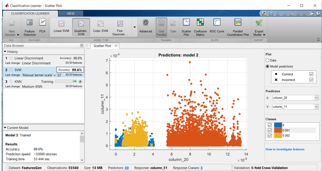
Figure 42: MATLAB Classification Learner App for Training EMG data using linear discriminant analysis and support vector machine
