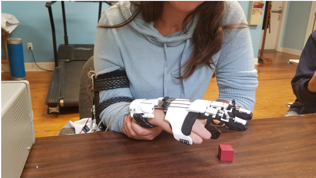
Figure 12: The subject wearing the HOPE Hand 1.0 which was customized to fit her hand
