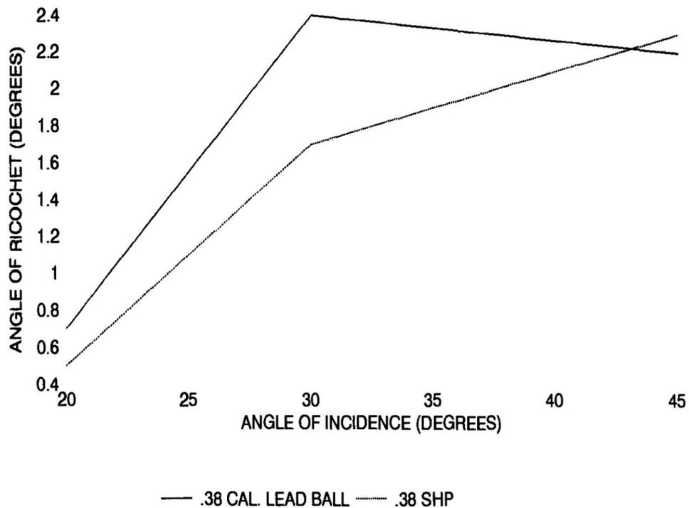
Figure 2: *Angle of ricochet versus angle of incidence. Solid line = .38 caliber lead ball; dashed line = .38 caliber semi-jacketed hollow point., Burk, Rowe.*
