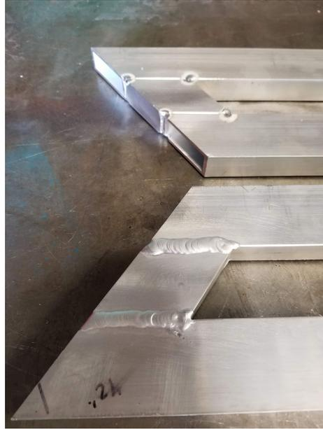
Figure 7: Complete weld compared to spot weld
