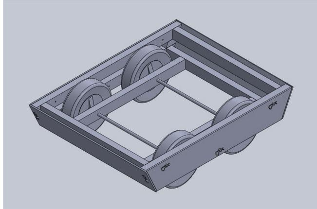
Figure 4: The frame assembly with the wheels installed
