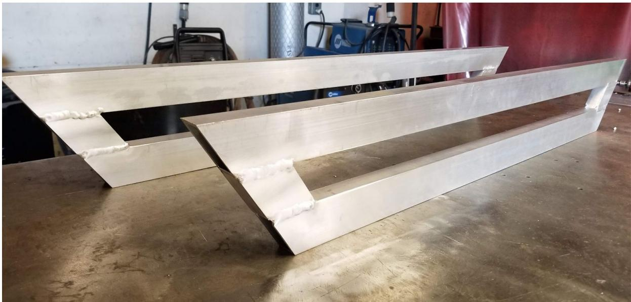
Figure 8: Completed weld of the sides of the frame
