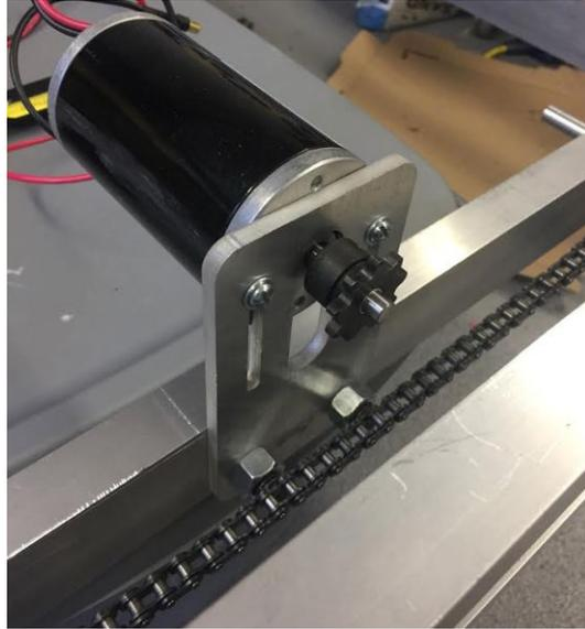
Figure 14: Motor Mount plates on the frame
