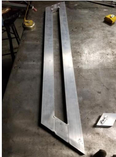
Figure 6: Side of the frame spot welded together.
