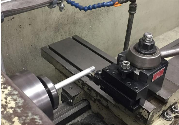
Figure 10: Turning the axles on the manual lathe
