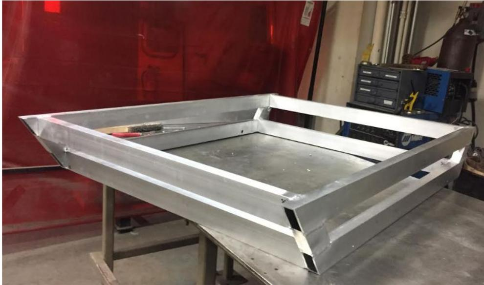
Figure 9: Four sides of the frame welded
