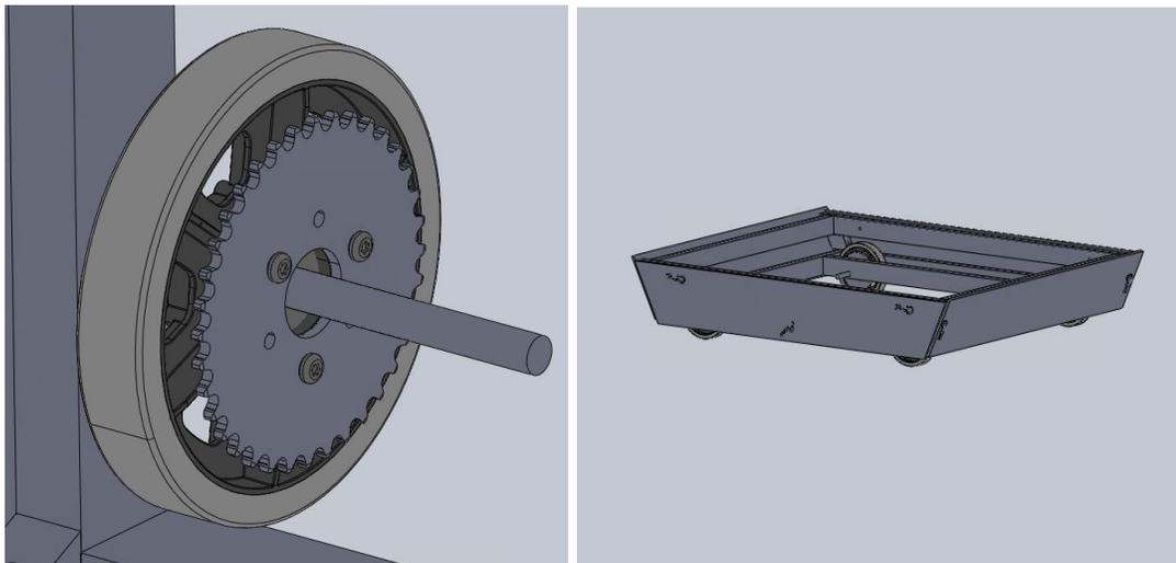
Figure 5: The frame assembly with a trimmed axle and wheel assembly
