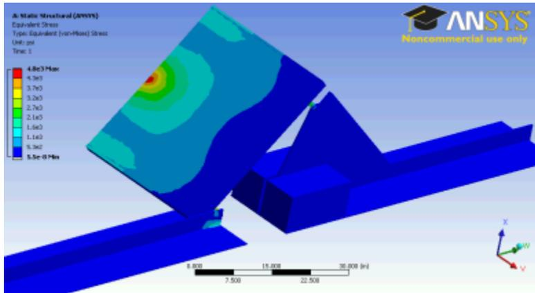
Figure 113. 1-inch Hail Strain, First Solar Ballasted
