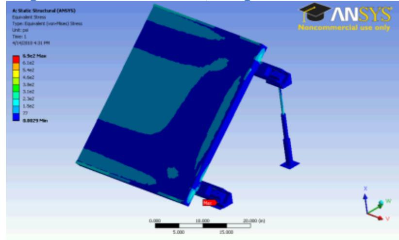
Figure 128. Baseline Strain, Evergreen Solar Attached
