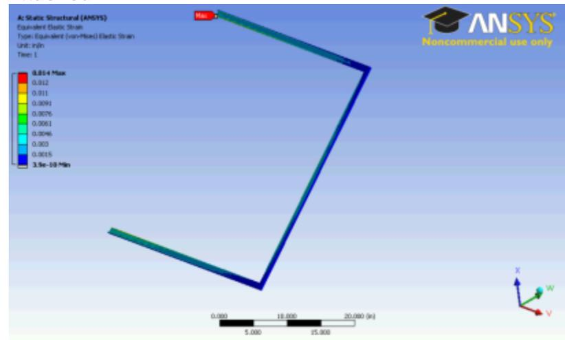
Figure 171. 1-inch Hail Impact Stress, Evergreen Solar Attached
