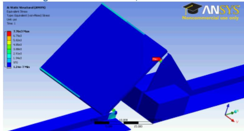
Figure 64. Wind Deformation, Evergreen Solar Ballasted
