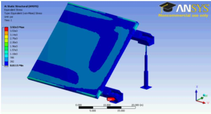
Figure 133. Wind Deformation, Front Surface, Evergreen Solar Attached
