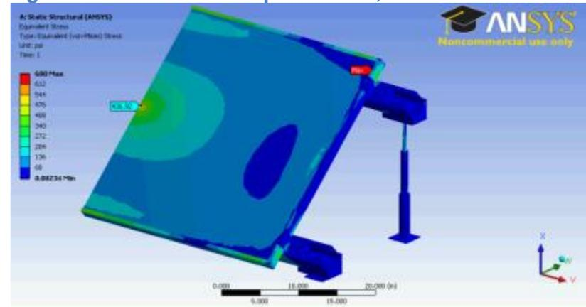
Figure 166. 2-inch Hail Impact Deformation, SunTech Attached
