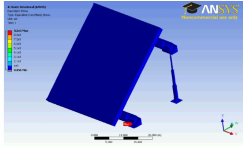
Figure 139. Wind Deformation, Front Surface, First Solar Attached
