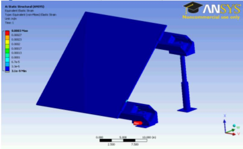
Figure 144. Wind Stress, Back Surface, First Solar Attached
