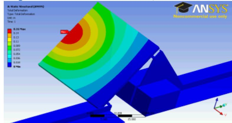
Figure 100. 1-inch Hail Deformation, Evergreen Solar Ballasted
