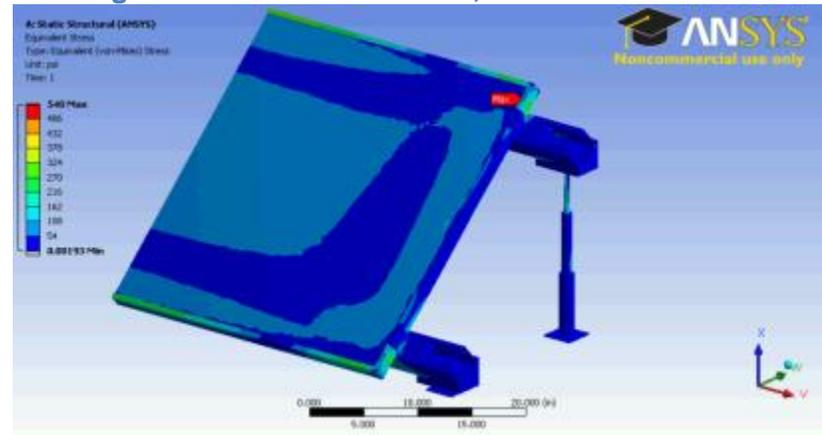
Figure 127. Baseline Deformation, Evergreen Solar Attached
