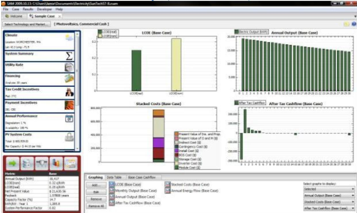
Figure 207. Performance Analysis, Evergreen Solar Tilted 27°, Oriented South
