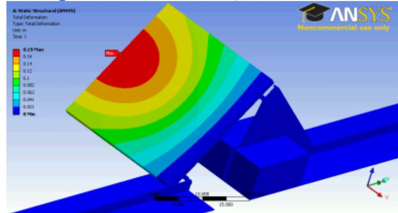
Figure 84. Ice Stress, Evergreen Solar Ballasted
