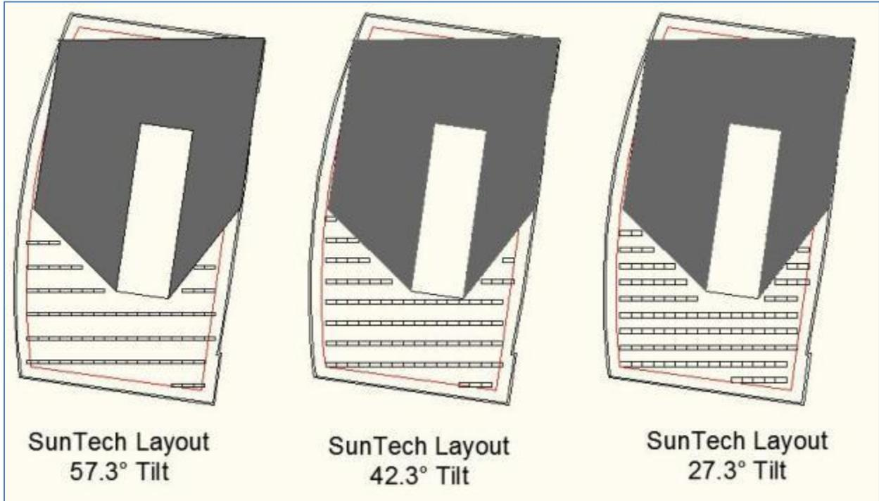
Figure 196. SunTech Layouts, Aligned with Roof Edge
