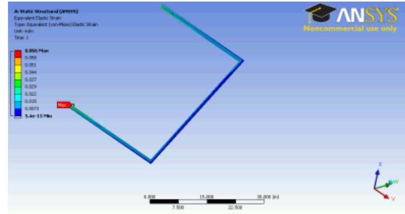
Figure 111. 2-inch Wind-driven Hail Stress, Evergreen Solar Ballasted
