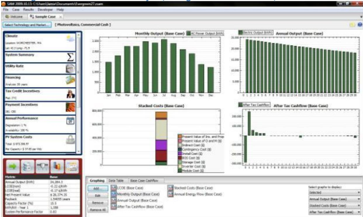
Figure 208. Performance Analysis, Evergreen Solar Tilted 27°, Oriented South -8°
