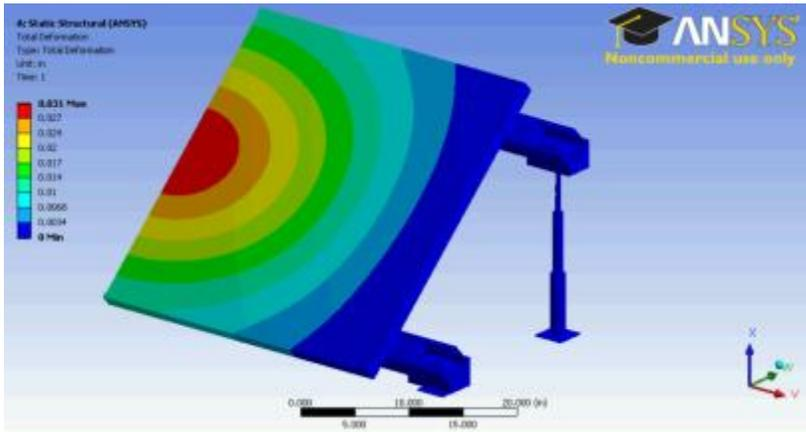
Figure 164. 1-inch Hail Impact Strain, SunTech Attached
