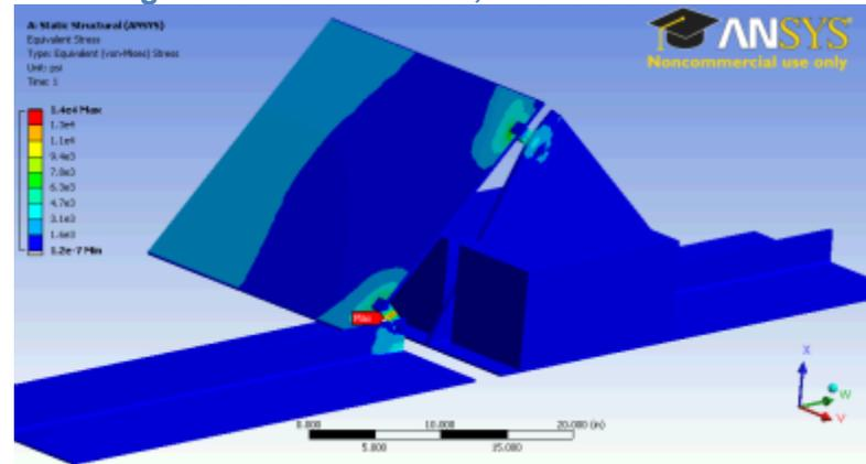
Figure 77. Snow Strain, First Solar Ballasted
