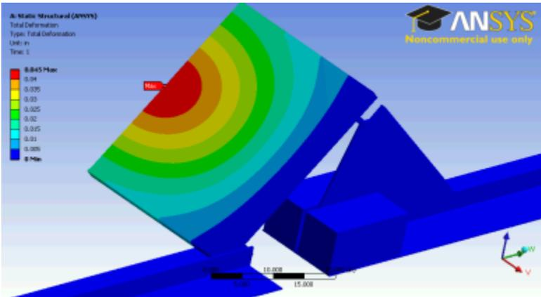
Figure 102. 1-inch Hail Stress, Evergreen Solar Ballasted
