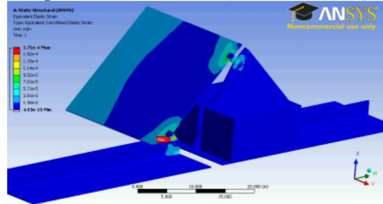
Figure 112. 1-inch Hail Deformation, First Solar Ballasted
