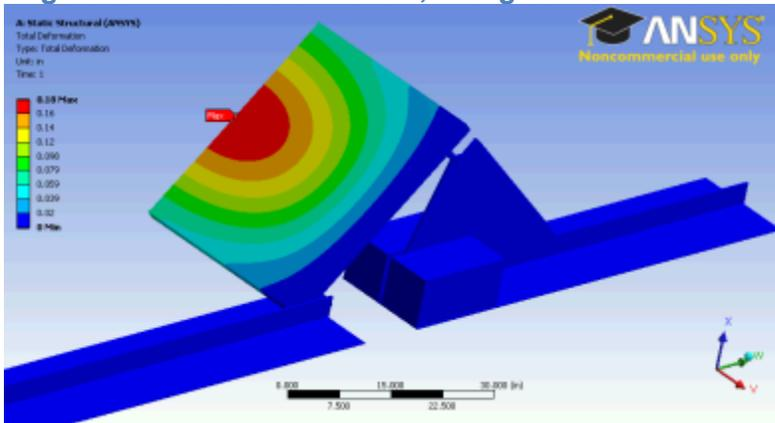
Figure 66. Wind Stress, Evergreen Solar Ballasted
