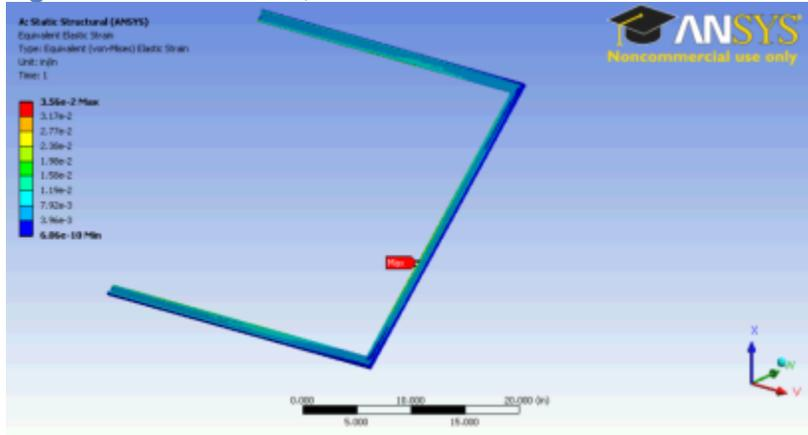
Figure 157. Ice Deformation, Evergreen Solar Attached
