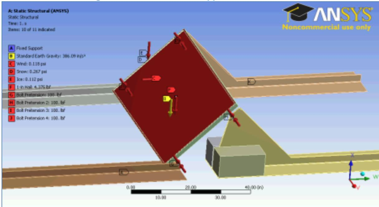
In the solution phase of a static structural simulation in ANSYS™ software, the stress, strain and deformation is calculated for each element. The average stress in an element is given by [65-67]
