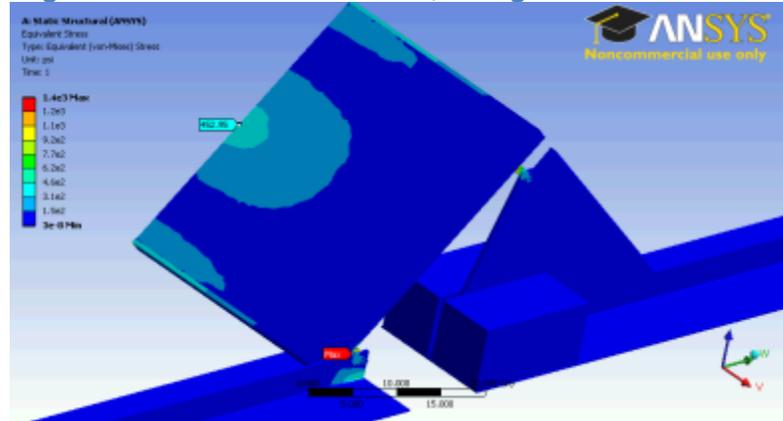
Figure 101. 1-inch Hail Strain, Evergreen Solar Ballasted
