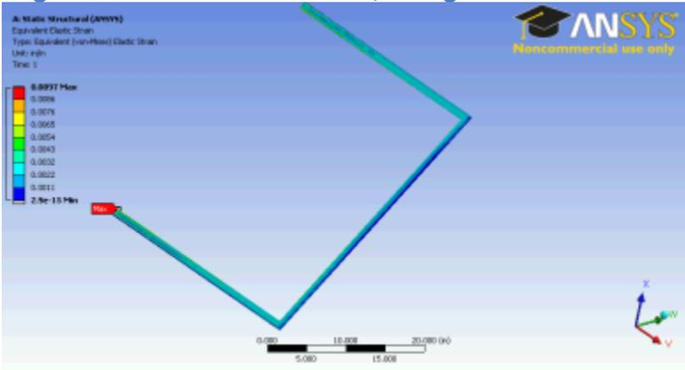
Figure 103. 2-inch Hail Deformation, Evergreen Solar Ballasted
