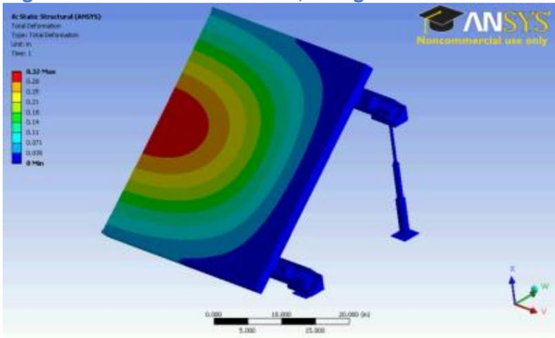
Figure 150. Snow Stress, Evergreen Solar Attached
