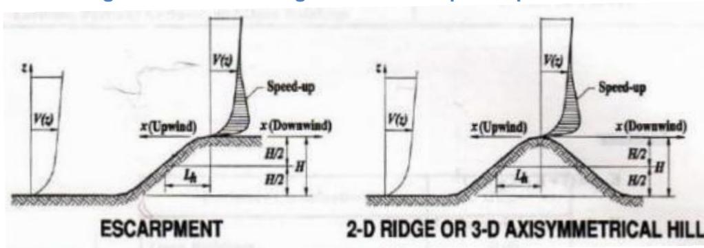
Figure 190. ASCE Charts for Wind Parameters
