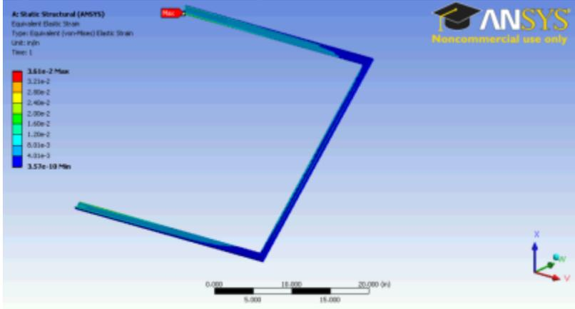
Figure 168. 2-inch Hail Impact Stress, SunTech Attached
