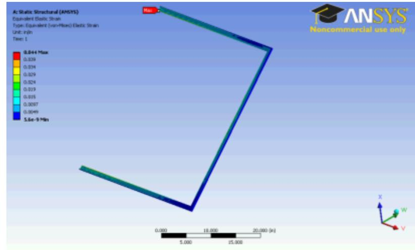
Figure 136. Wind Deformation, Back Surface, Evergreen Solar Attached
