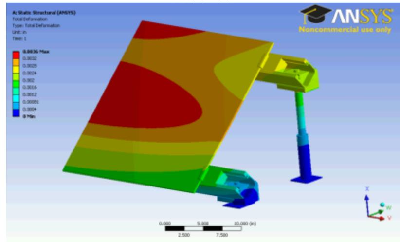
Figure 143. Wind Strain, Back Surface, First Solar Attache
