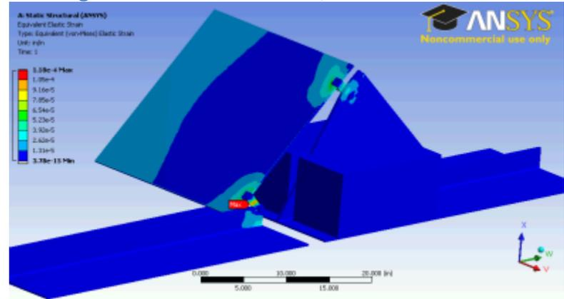
Figure 60. Baseline Stress, First Solar Ballasted
