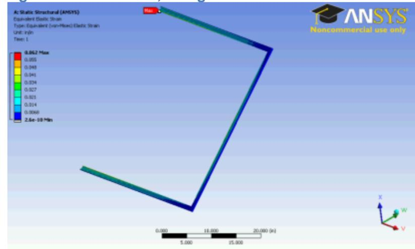
Figure 159. Ice Stress, Evergreen Solar Attached
