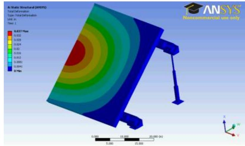
Figure 170. 1-inch Hail Impact Strain, Evergreen Solar Attached
