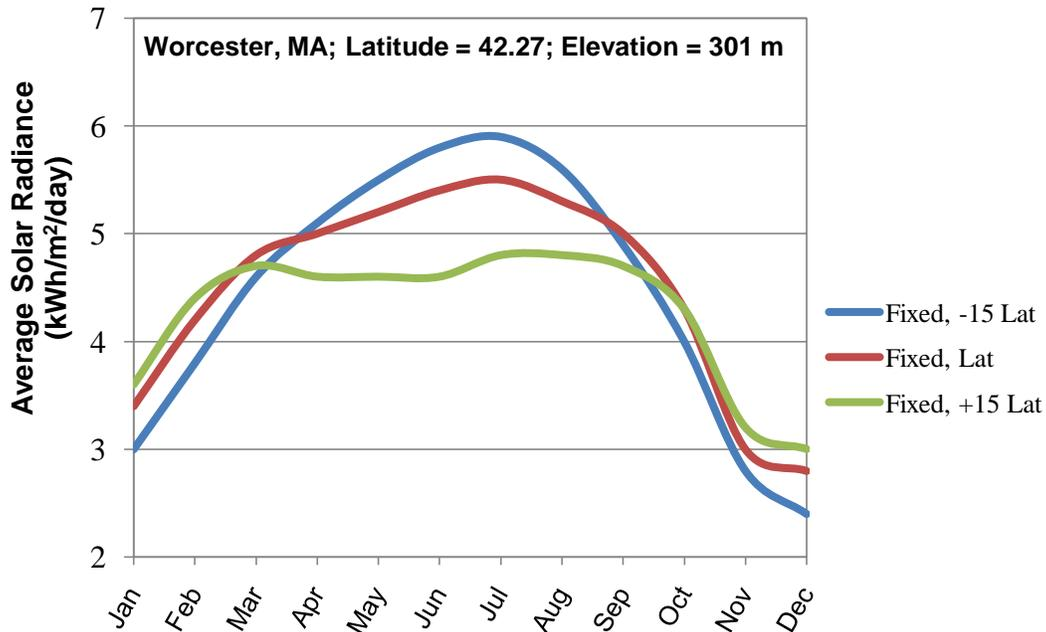
Accurate solar resource data requires advanced study of highly variable weather conditions, atmospheric particles (such as ozone, aerosols, water vapor, etc.), and reflected radiation [10]. The performance analysis of the WPI PV array was calculated using state-of-the-art software
