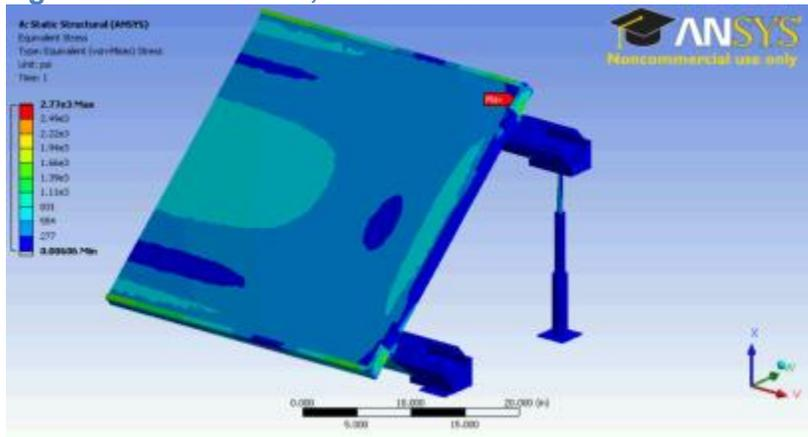
Figure 158. Ice Strain, Evergreen Solar Attached
