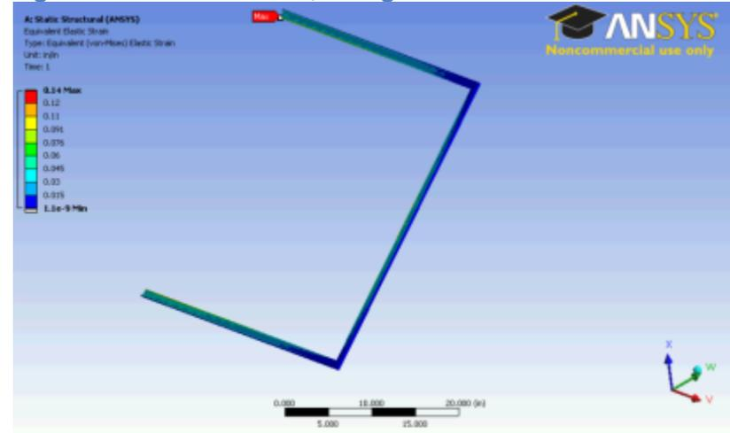
Figure 148. Snow Deformation, Evergreen Solar Attached
