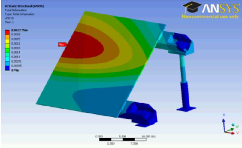
Figure 162. Ice Stress, First Solar Attached
