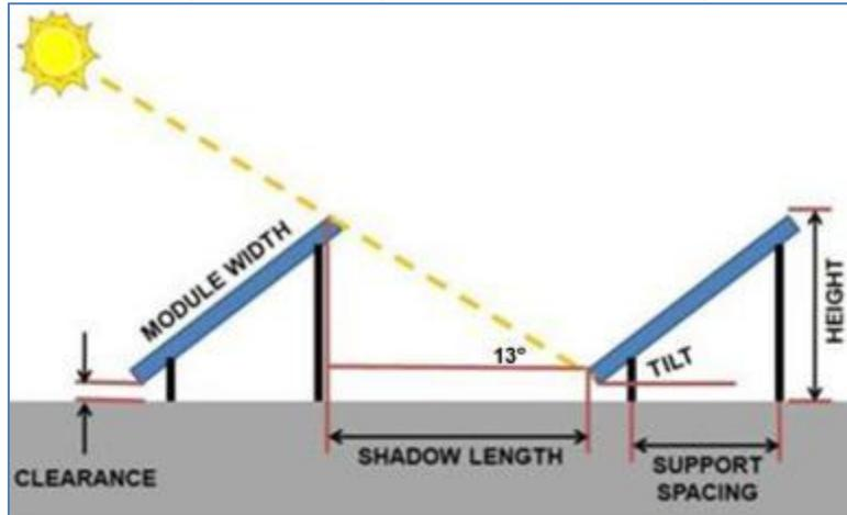
In order to calculate the optimum module row spacing, the shadow length ( $S$ ) is calculated using the sun's elevation ( $E_s$ ) on the winter solstice, the module width ( $W$ ), and the height of the system projected from the module width line ( $H_p$ ). The  $H_p$  is determined from  $W$  and the tilt angle ( $\theta_T$ ) such that
