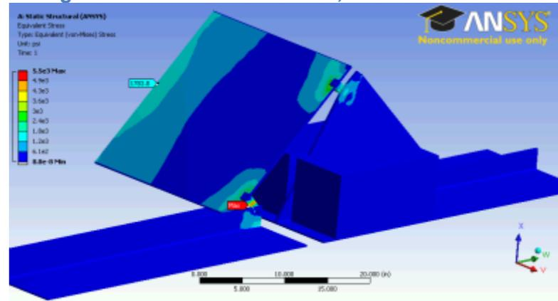
Figure 116. 2-inch Hail Strain, First Solar Ballasted
