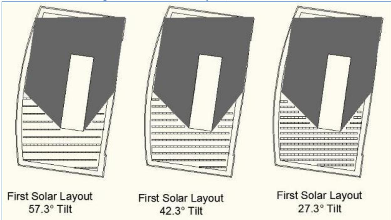
Figure 200. First Solar Layout, Aligned with Roof Edge
