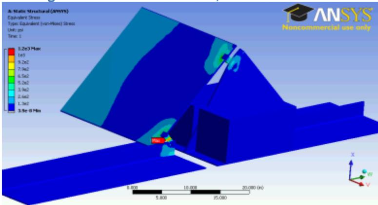
Figure 62. Wind Strain, SunTech Ballasted
