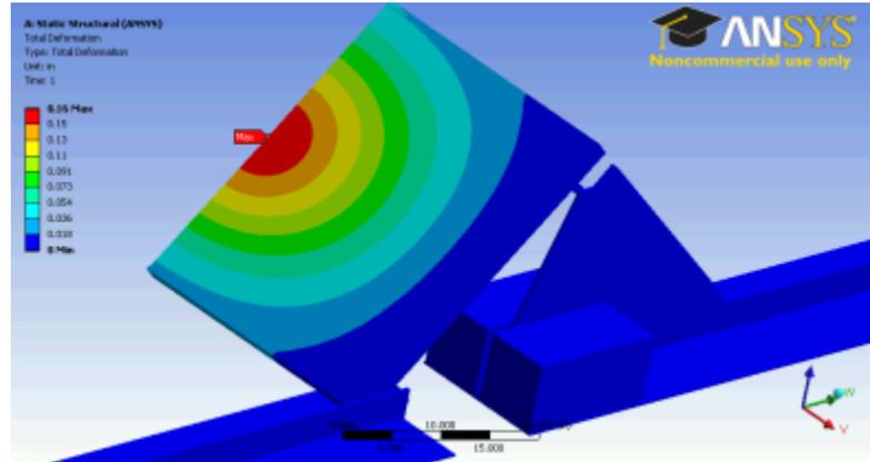
Figure 108. 1-inch Wind-driven Hail Stress, Evergreen Solar Ballasted
