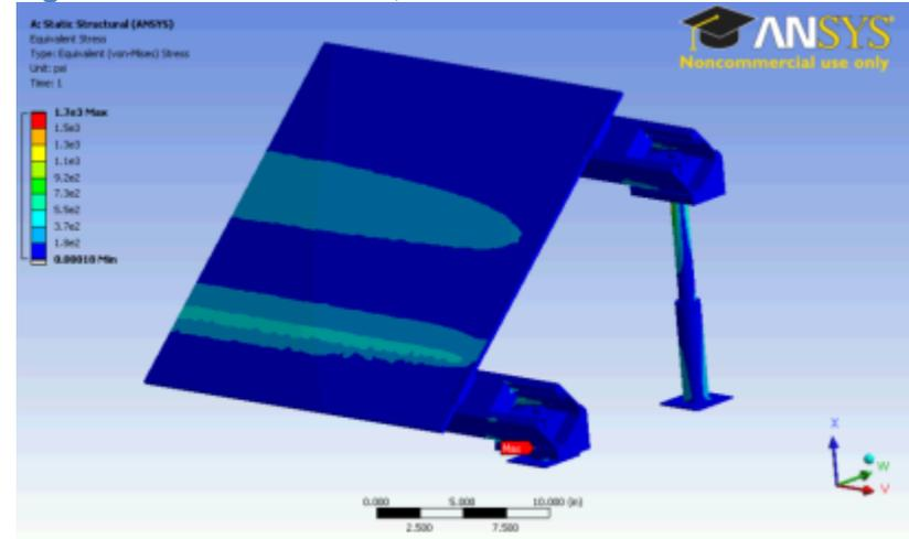
Figure 152. Snow Strain, First Solar Attached
