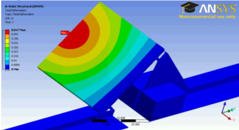
Figure 90. 1-inch Hail Stress, SunTech Ballasted
