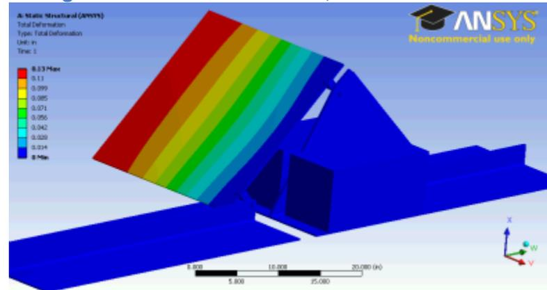
Figure 72. Snow Stress, SunTech Ballasted
