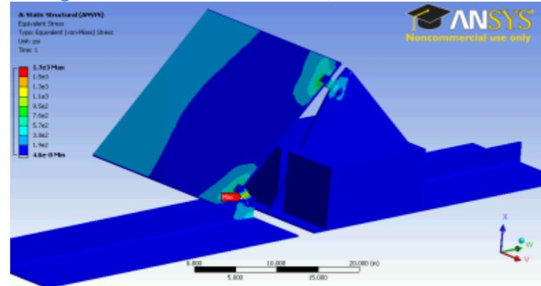
Figure 115. 2-inch Hail Deformation, First Solar Ballasted
