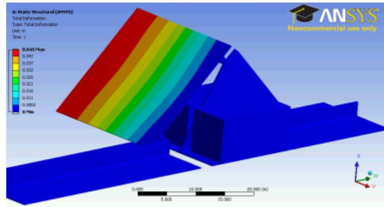
Figure 123. 2-inch Wind-driven Hail Stress, First Solar Ballasted
