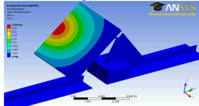
Figure 110. 2-inch Wind-driven Hail Strain, Evergreen Solar Ballasted
