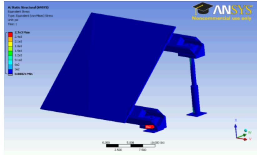
Figure 140. Wind Strain, Front Surface, First Solar Attached
