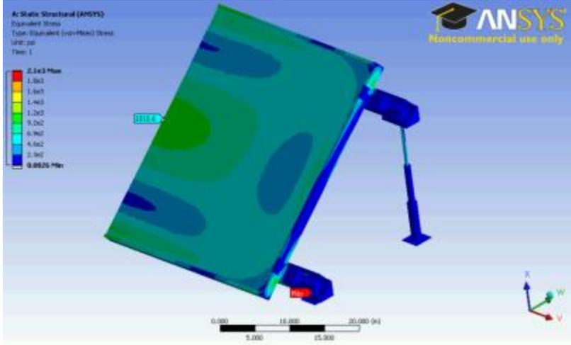
Figure 161. Ice Strain, First Solar Attached
