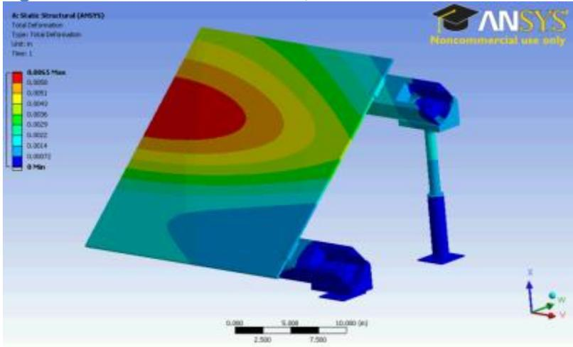
Figure 153. Snow Stress, First Solar Attached
