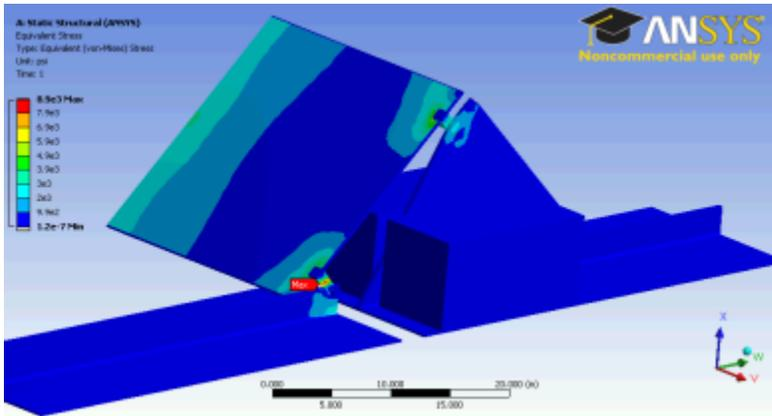
Figure 125. Baseline Strain, SunTech Attached
