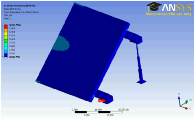
Figure 137. Wind Strain, Back Surface, Evergreen Solar Attached
