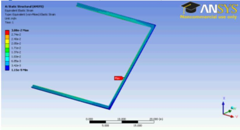
Figure 132. Wind Stress, Front Surface, SunTech Attached
