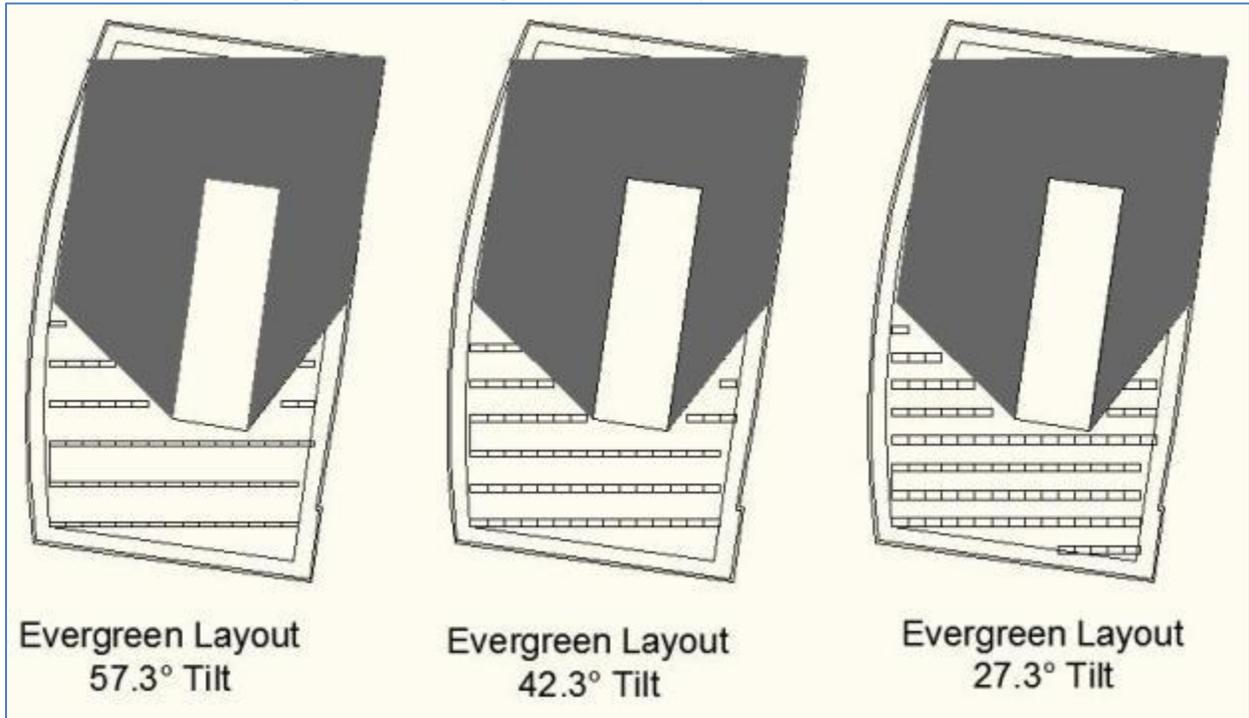
Figure 198. Evergreen Solar Layout, Aligned with Roof Edge
