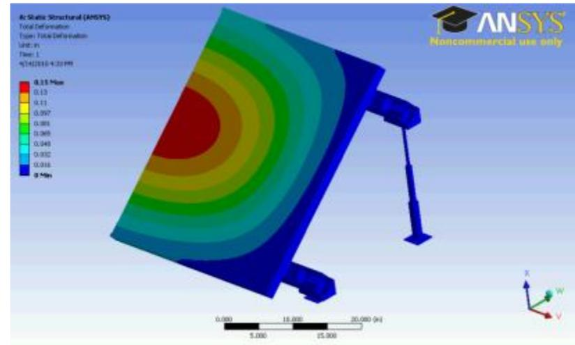
Figure 134. Wind Strain, Front Surface, Evergreen Solar Attached
