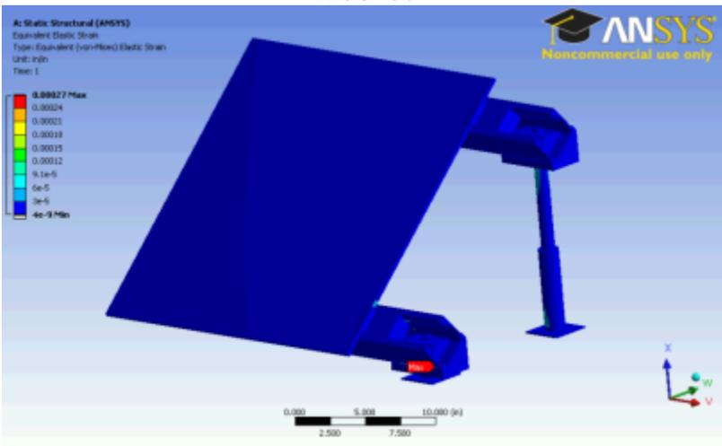
Figure 142. Wind Deformation, Back Surface, First Solar Attached
