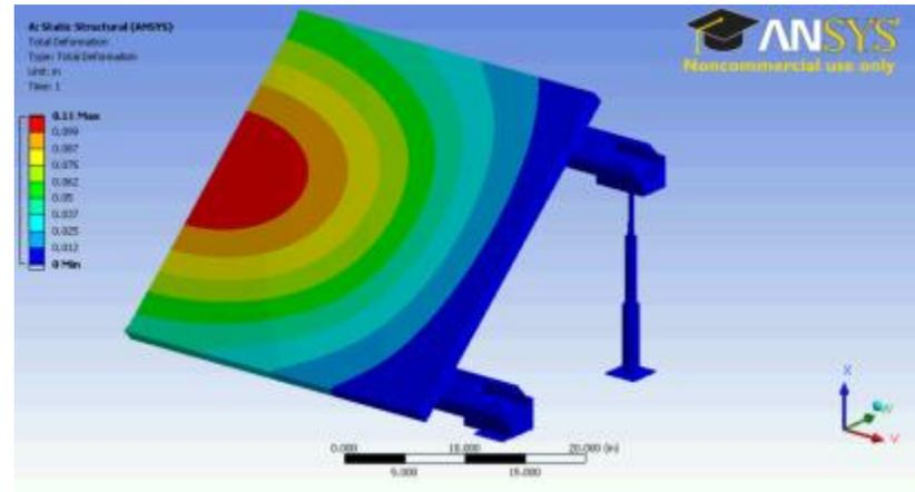
Figure 131. Wind Strain, Front Surface, SunTech Attached
