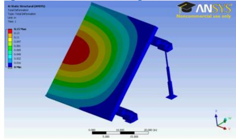
Figure 156. Ice Stress, SunTech Attached
