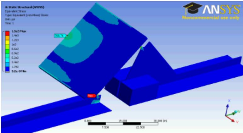
Figure 109. 2-inch Wind-driven Hail Deformation, Evergreen Ballasted
