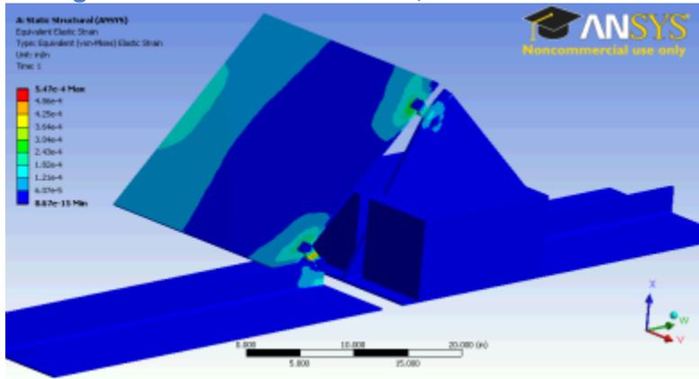
Figure 118. 1-inch Wind-driven Hail Deformation, First Solar Ballasted
