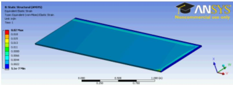
Figure 184. August Stress in a CdTe PV Module
