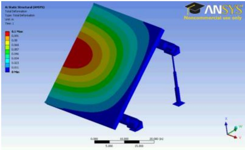
Figure 138. Wind Stress, Back Surface, Evergreen Solar Attached
