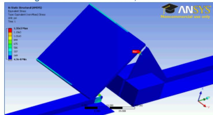
Figure 53. Baseline Strain, SunTech Ballasted
