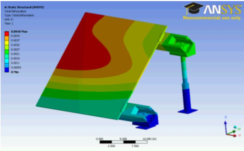
Figure 141. Wind Stress, Front Surface, First Solar Attached
