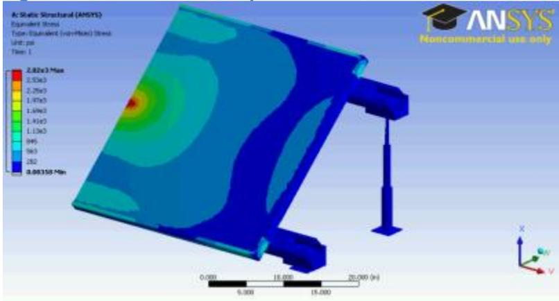
Figure 169. 1-inch Hail Impact Deformation, Evergreen Solar Attached
