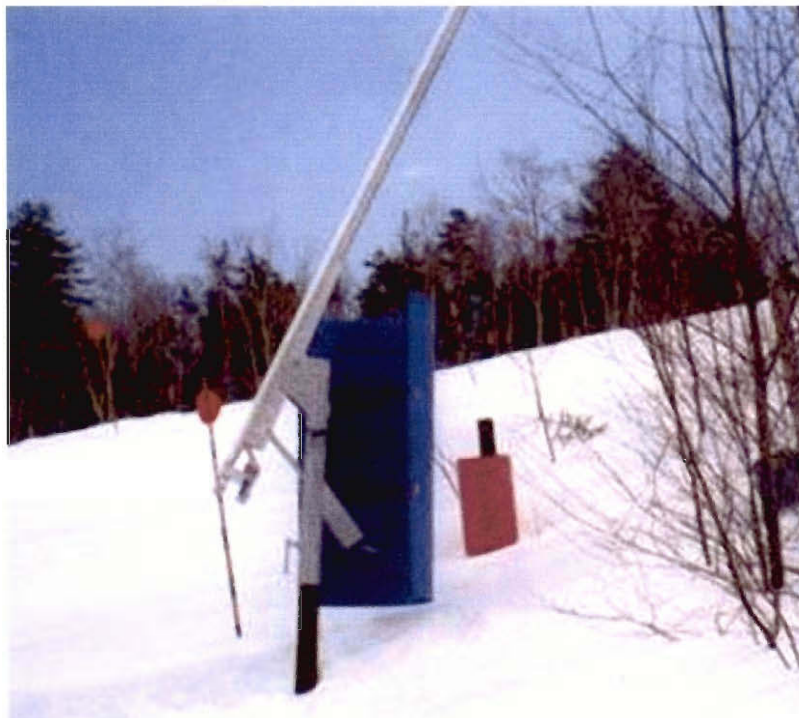
Fig 3.67 Braced shield on tower gun
