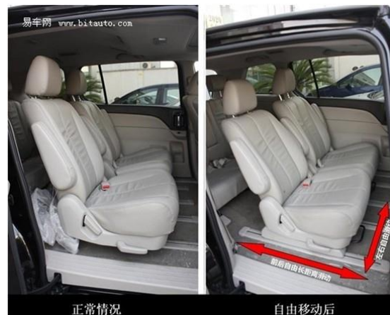
Figure 2.5 Moving (Sliding) Method
