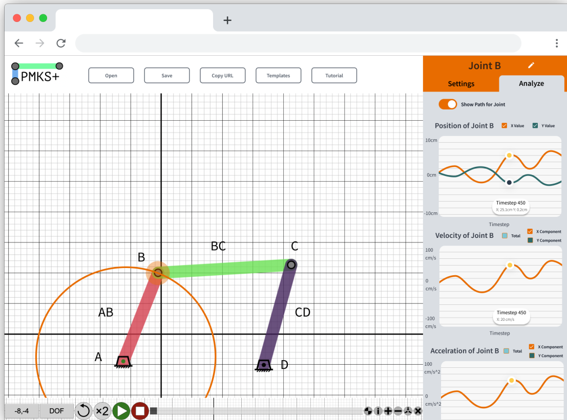
Figure 29: Mockup one introduces the idea of clicking an object to select it. The right panel shows settings (position, grounded?) or analysis graphs for the selected object.
