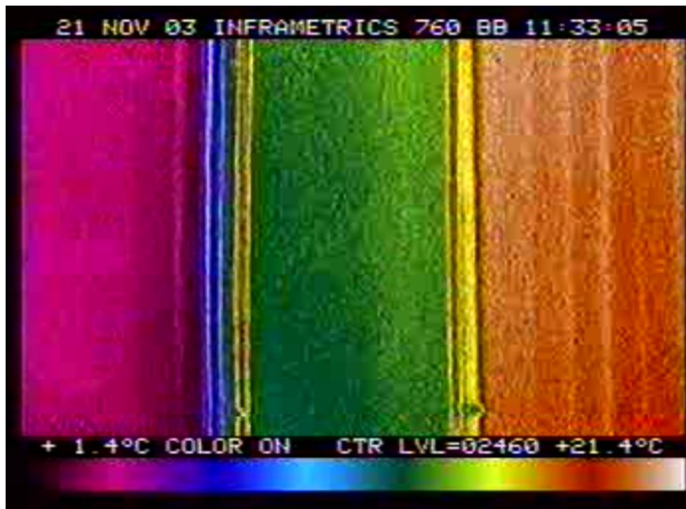
Figure 14a. Thermal Image of Regular Window, Storm Window, and Blinds
