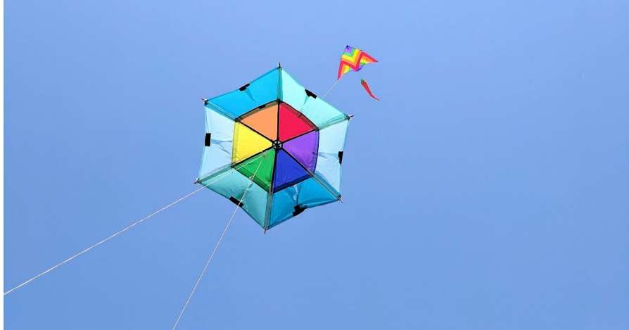
Figure 28. Third Iteration Popper during Field Testing. The delta kite area is greater than the popper area.
