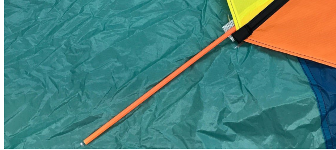
Figure 22. Additional Support Poles to Support New Panels on First Iteration Popper
