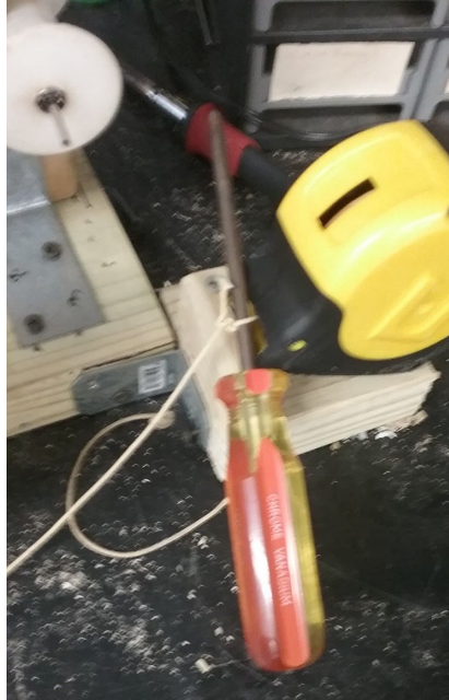
Figure 44. Intentional, reversible jamming of the retraction system with a screwdriver.
