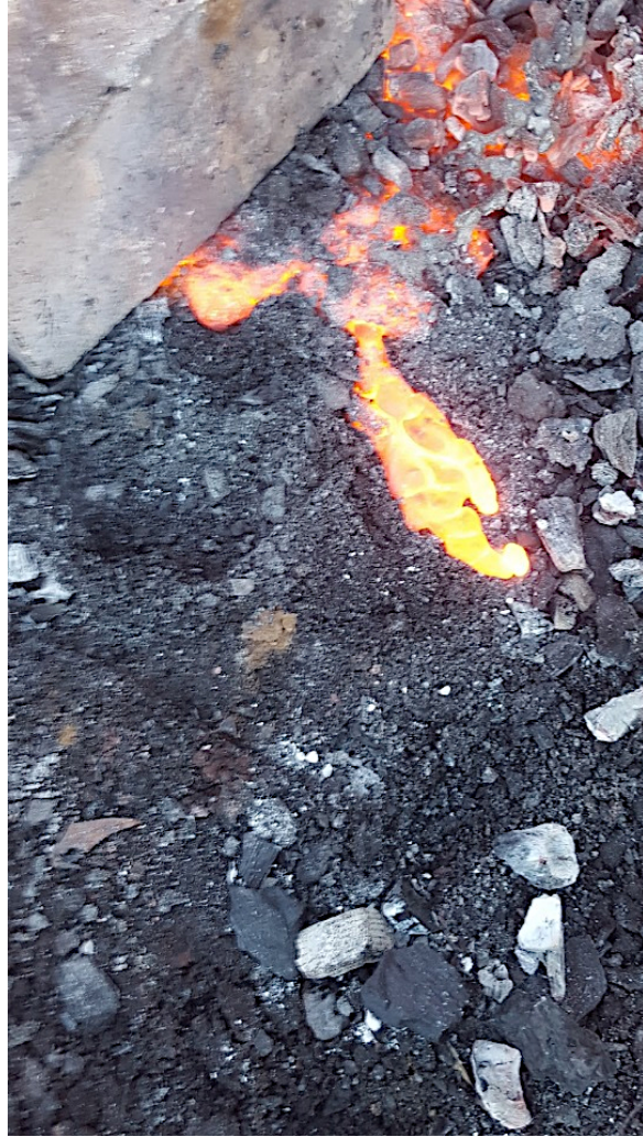
FIGURE 44. TAPPING SLAG FROM FURNACE.
