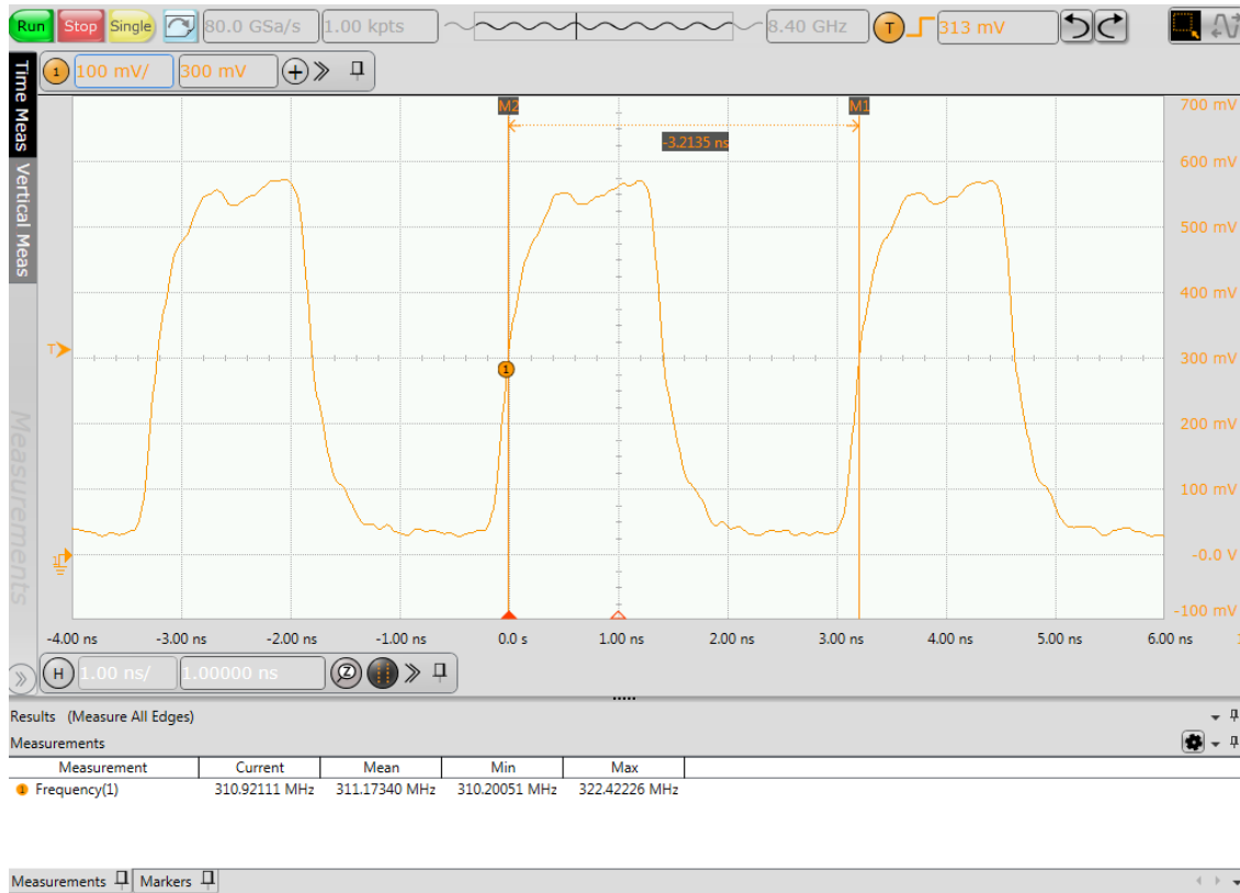
Figure 5.10: Waveform of VCO at V_{in} = 1.8V (Maximum)
