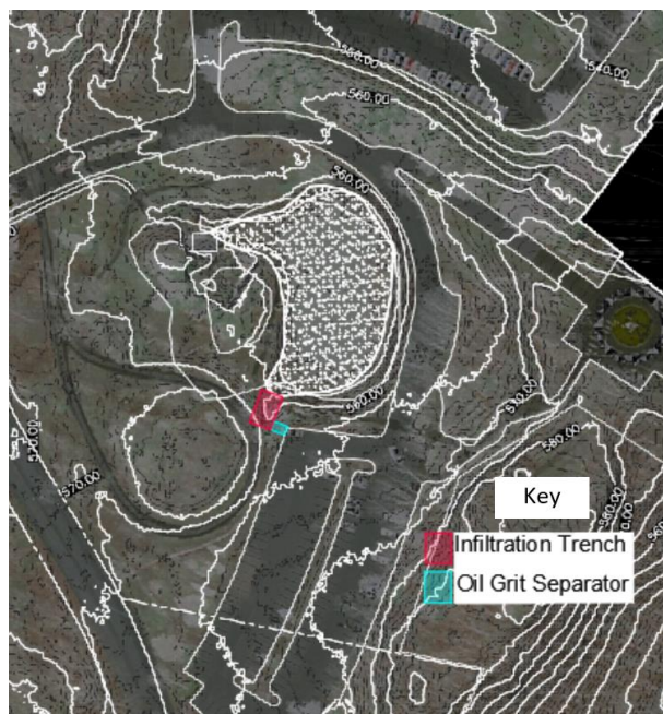
Figure 16: The location of the oil/grit separator and infiltration trench compared to the upper lot. The outline of the upper parking lot can be seen next to the oil/grit separator. The pond can be seen above the infiltration trench.
