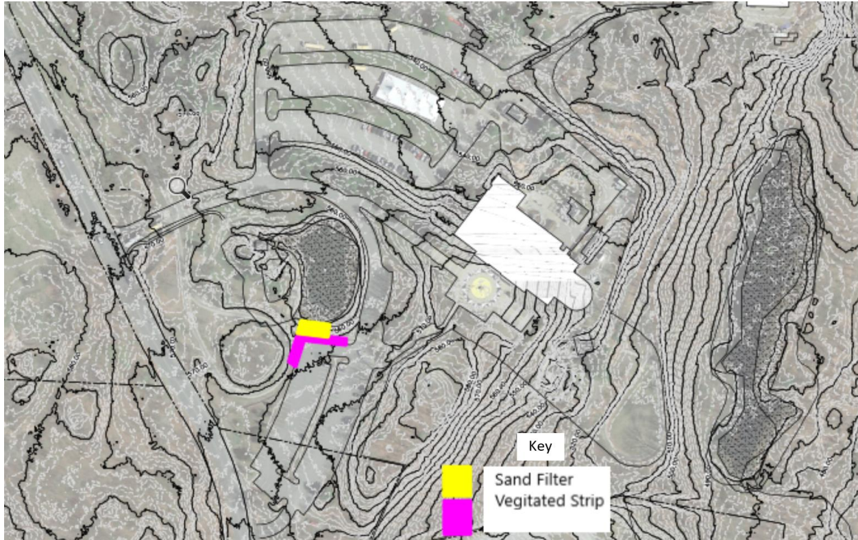
Figure 17: The location of the vegetated filter strip and sand filter. The vegetated filter strip lines the corner of the upper parking lot and the sand filter runs to the edge of the upper pond.
