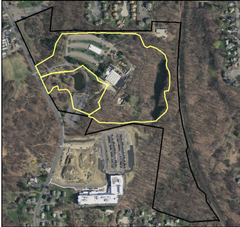
Figure 14: The subcatchments around the EcoTarium Ponds. The smaller yellow section contains the flow from the upper parking lot into the upper pond. The larger yellow section contains the lower parking lot and the stream. They both flow into the lower pond. The black line shows the perimeter of the EcoTarium.
