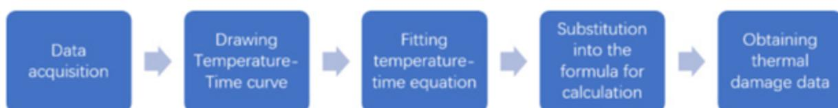
Figure 36: General method for thermal damage calculation [22]
