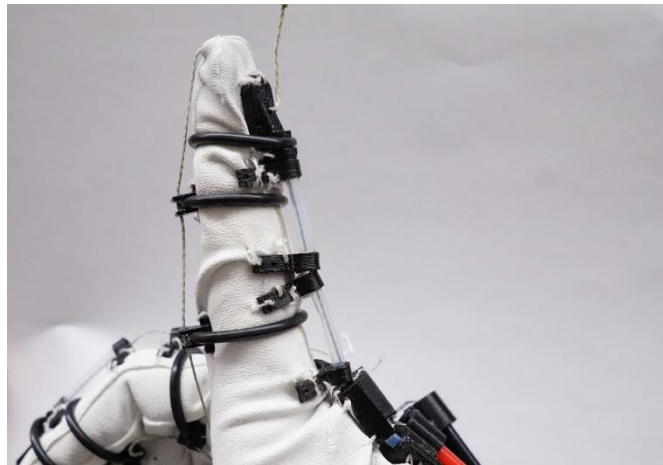
FIGURE 35: EXOSKELETON GLOVE INDEX FINGER AT MAXIMUM FLEXION LIMIT
