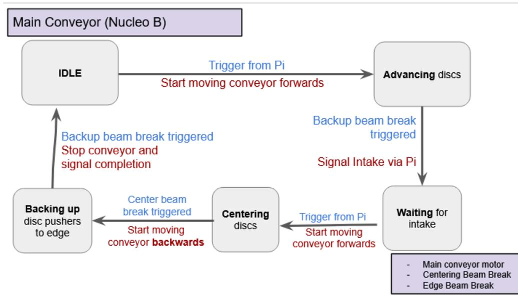
Figure 15. State machine diagram for the main conveyor system
