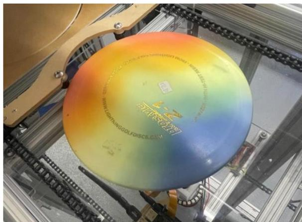
*Figure 12. Picture of the chain and disc alignment tool system of the main conveyor*
