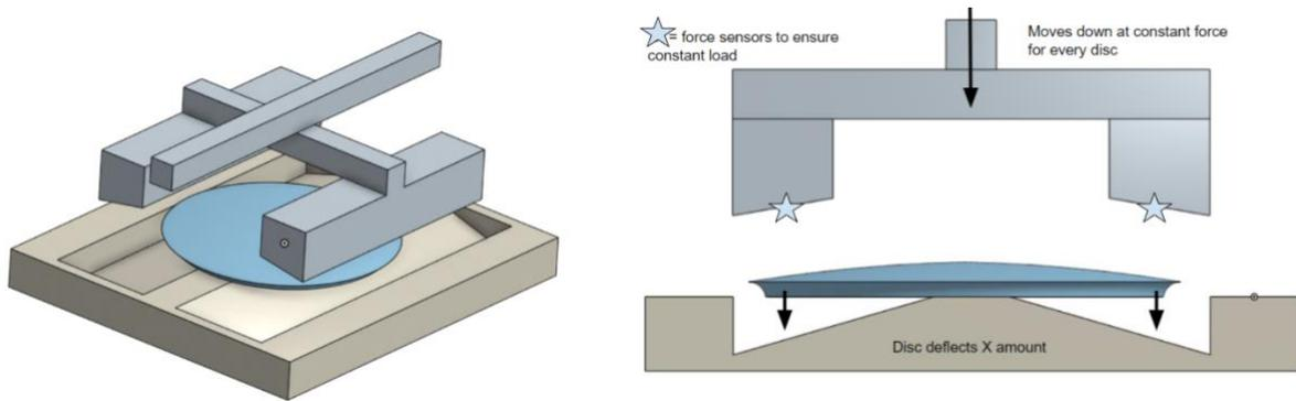
Figure 21. Isometric view (left) and side view (right) of first flexibility's prototype
