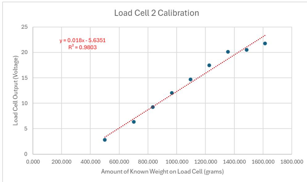
Figure 27. Calibration curve for load cell 2
