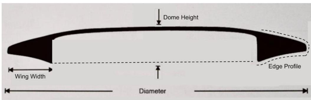
*Figure 1. Desired measurements of a disc*
