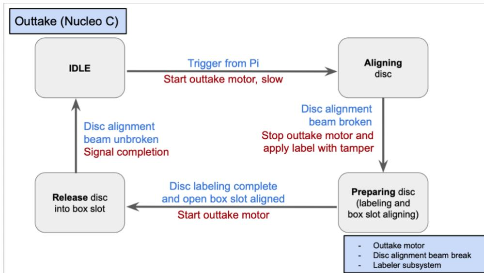
Figure 40. State diagram for the outtake ramp assembly
