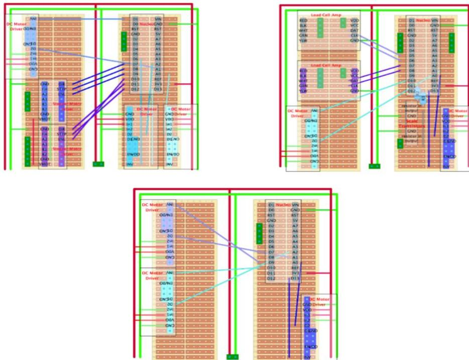
Figure 51. Wire diagrams for Nucleo A (first), B (second), and C (third) from left to right
