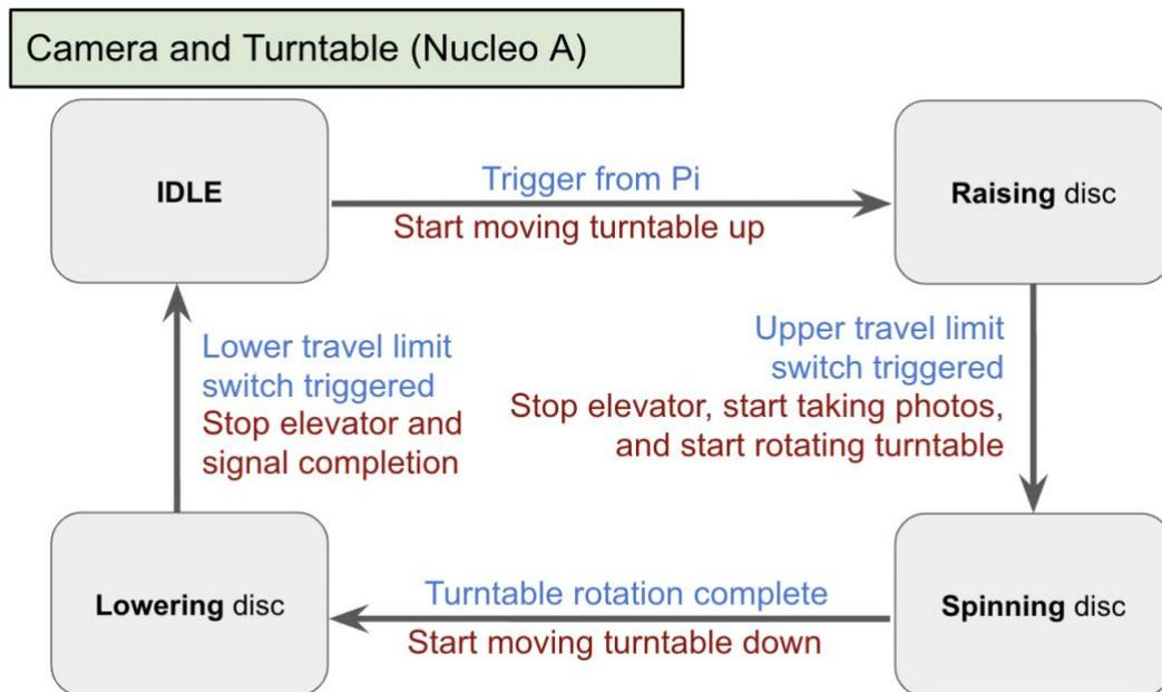
Figure 18. State machine diagram for camera and turntable system
