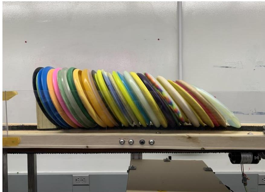
*Figure 9. Inherited design with loaded discs showing slippage*
