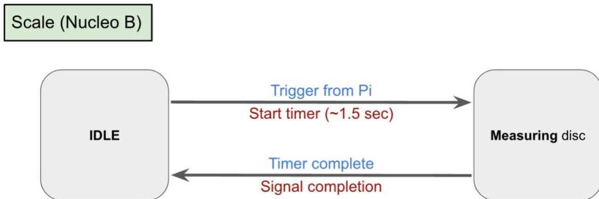
Figure 29. State diagram of scale module
