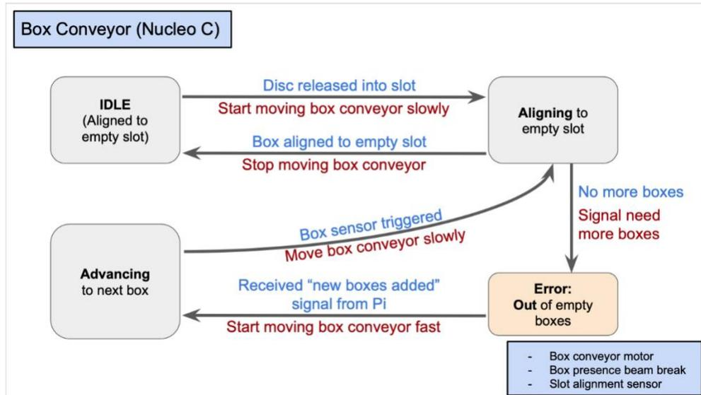
Figure 39. State diagram for the box conveyor assembly
