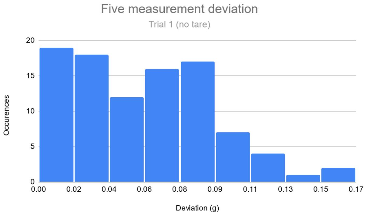
Figure 32. Scale repeatability testing deviation after 5 measurements
