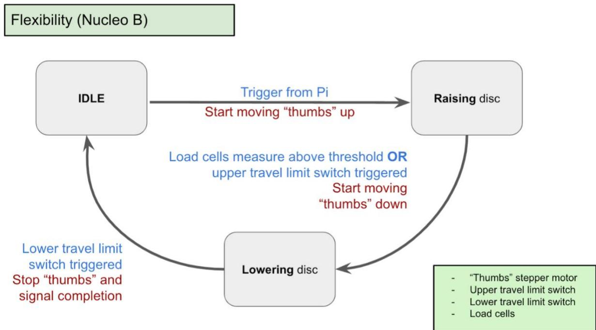
Figure 25. Flexibility module state diagram
