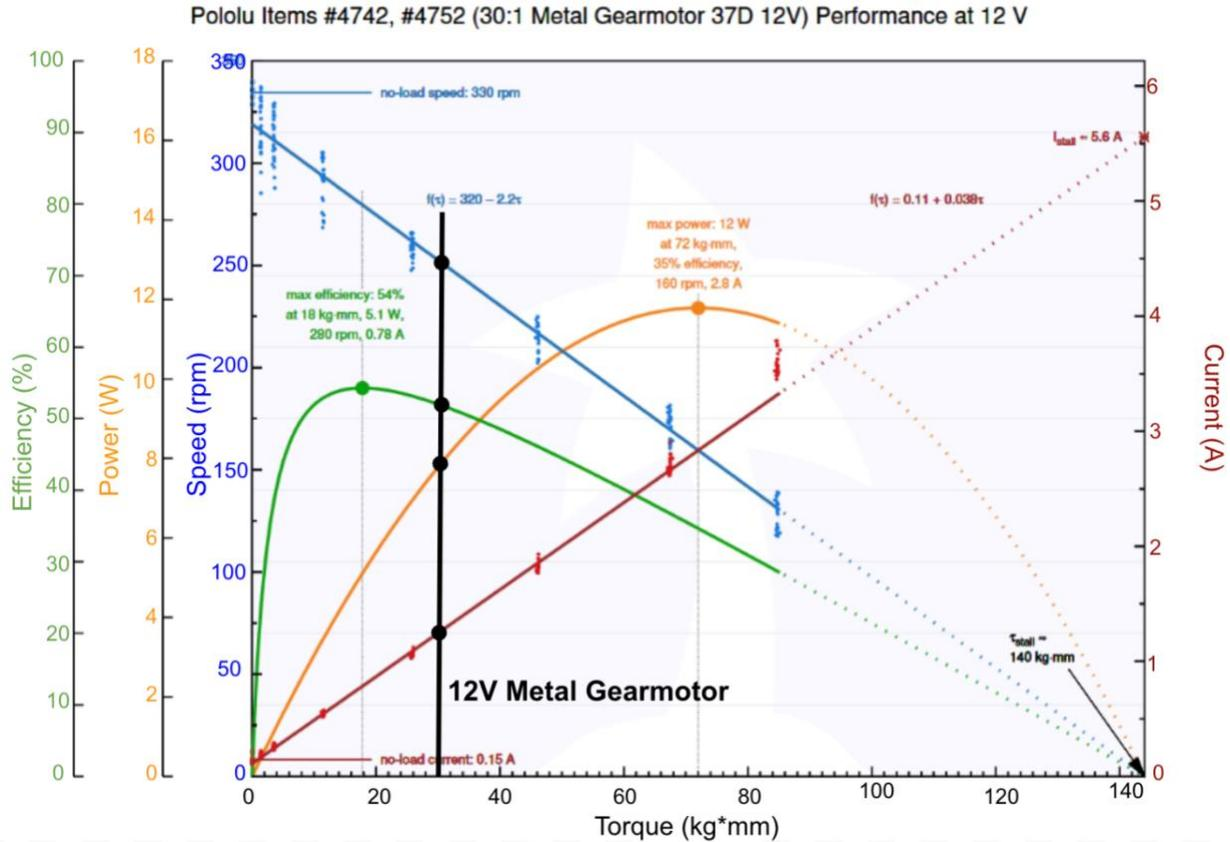
Figure 14. Motor specification diagram for the 12V 37D Metal Gearmotor
