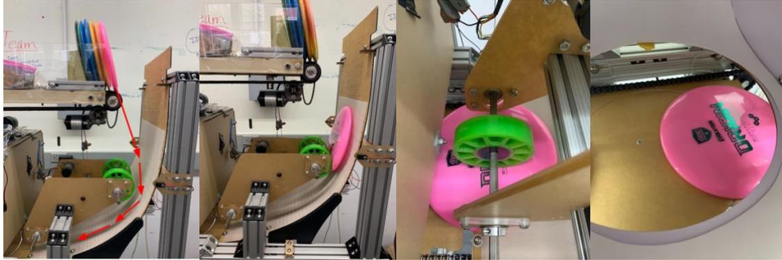
*Figure 8. Demonstration of disc motion from top conveyor through the intake*
