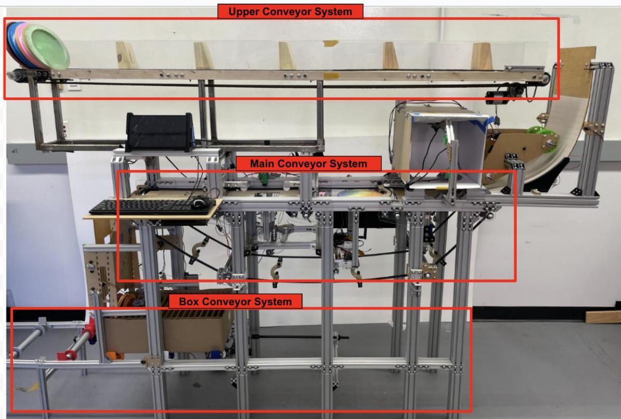
Figure 3. System overview of conveyors on the machine
