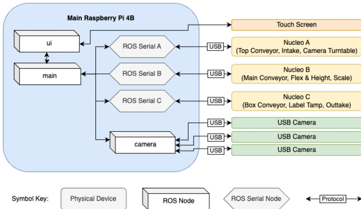
Figure 5. Raspberry Pi and ROS communication with Nucleo subsystems
