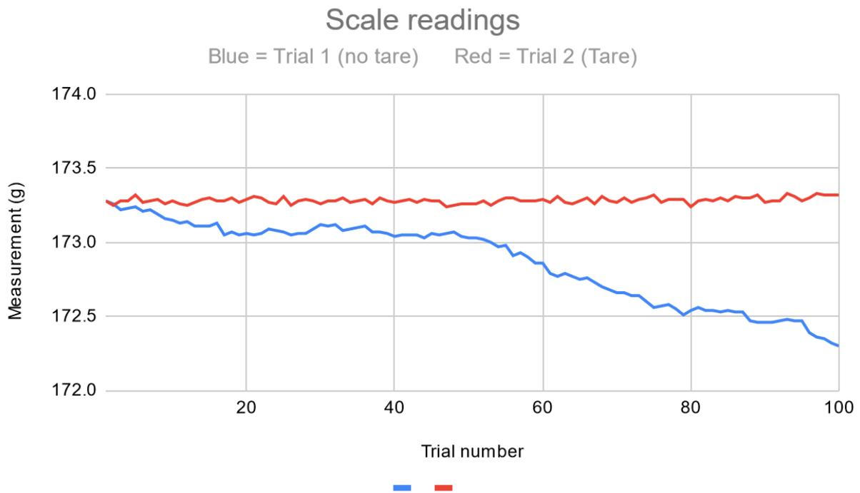
Figure 30. Scale repeatability testing recorded measurements over course of trials
