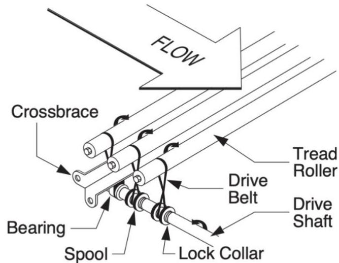
*Figure 38. Shaft and pulley driving diagram*
