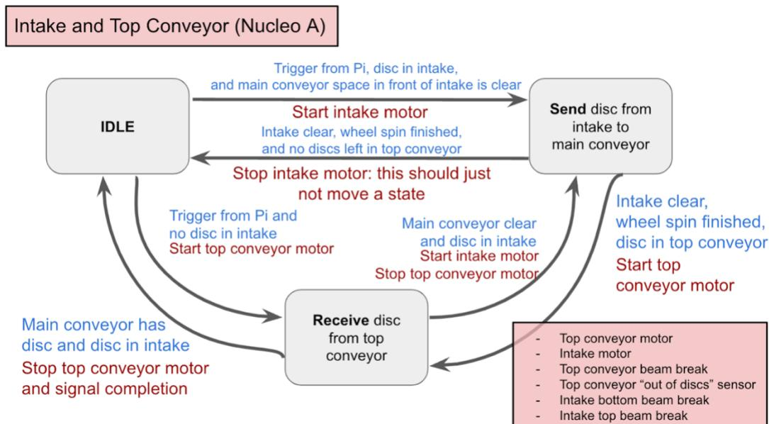
Figure 11. State machine diagram for the upper conveyor and intake system
