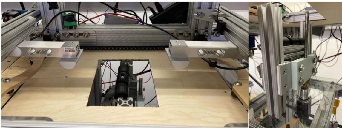
*Figure 23. Flexibility module assemblies above (left) and below (right) the main conveyor*
