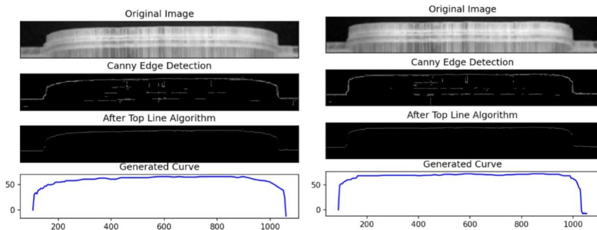
Figure 42. Images of different discs using profile module (top), Canny Edge Detection processing on captured profile image (second from top), graph using custom algorithm to isolate topmost pixels of Canny Edge (third), and final generated curve (bottom)
