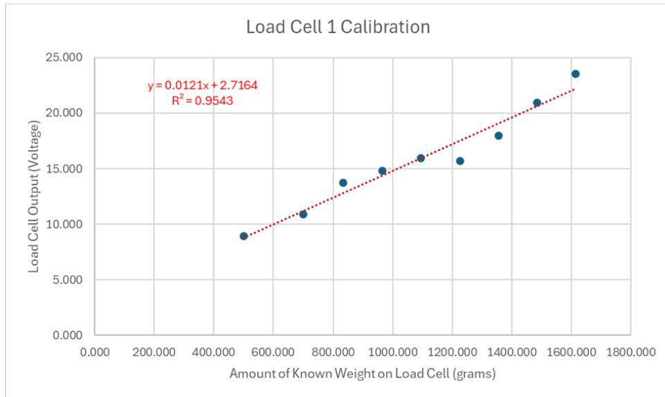
Figure 26. Calibration curve for load cell 1
