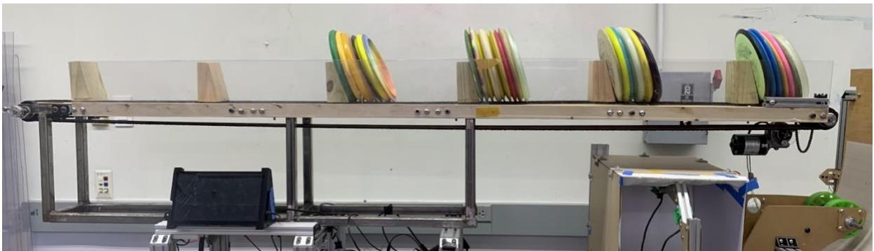
*Figure 7. The upper conveyor loaded with all the discs available to the team*
