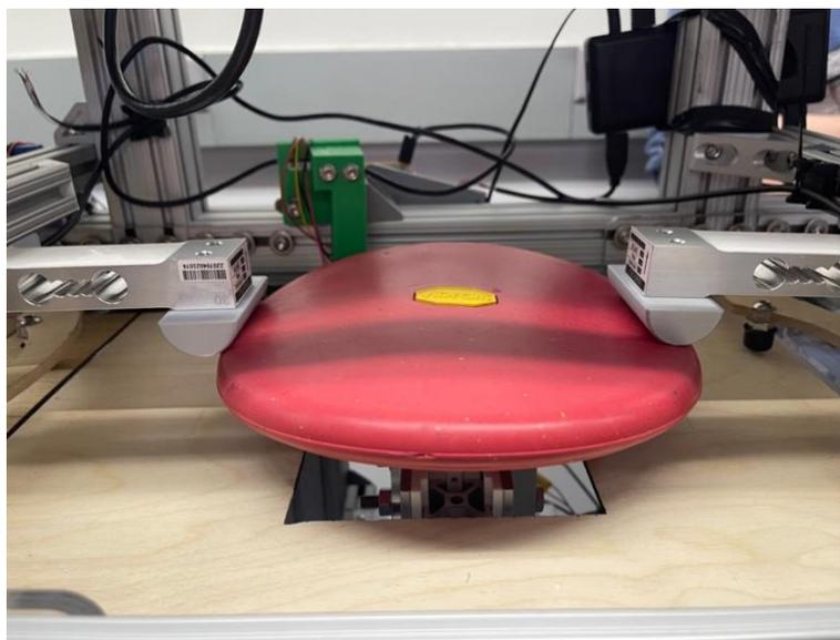
*Figure 24. Successful bend of a disc in the flexibility module*
