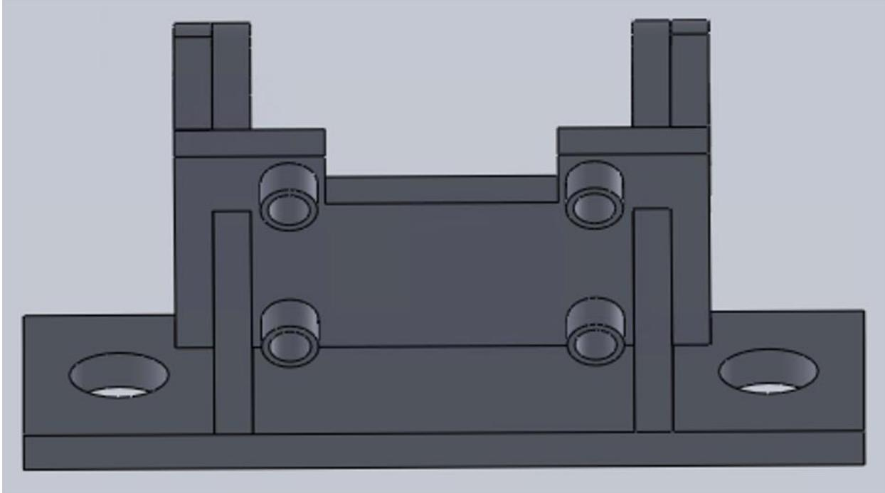
*Figure 36. Distance sensor mount*
