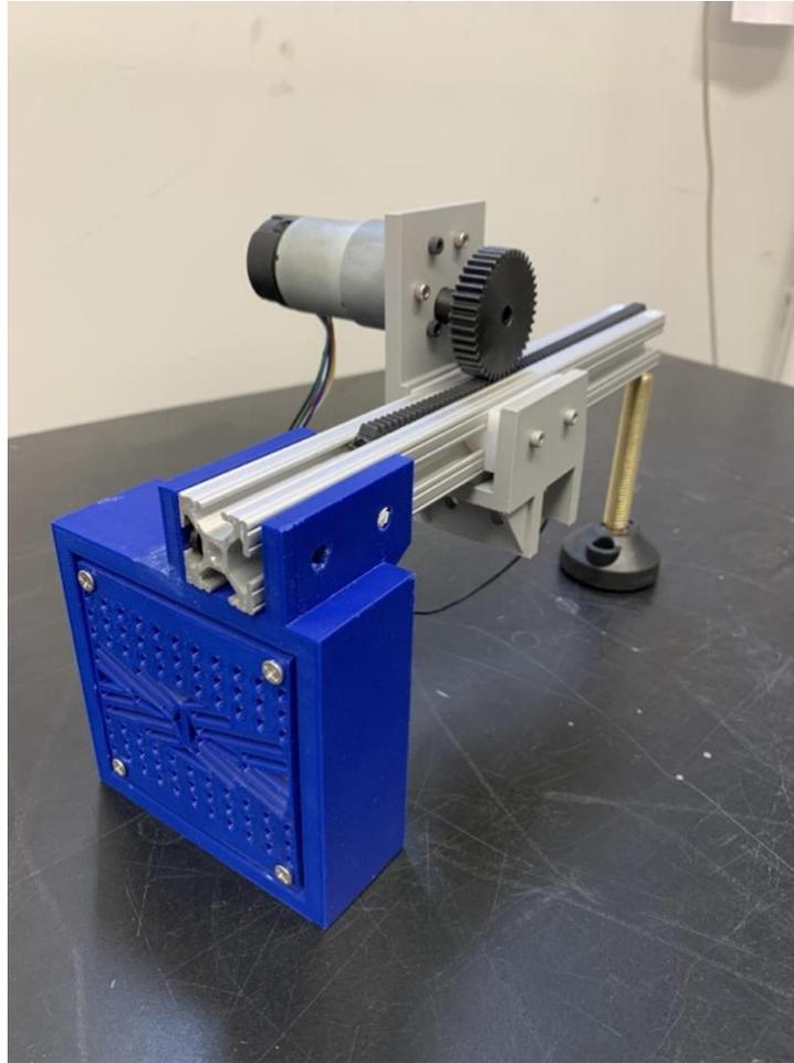
*Figure 43. Labeler tamper prototype which features a rack and pinion linear actuator and a suction box to grab the label*
