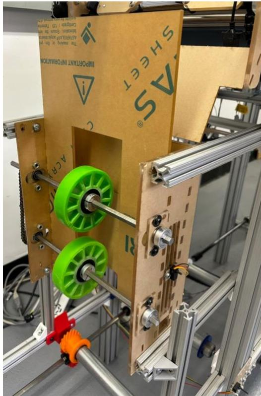
*Figure 35. Outtake ramp assembly*
