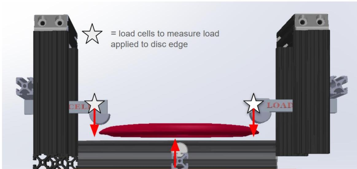
*Figure 22. Side view of final flexibility module design*
