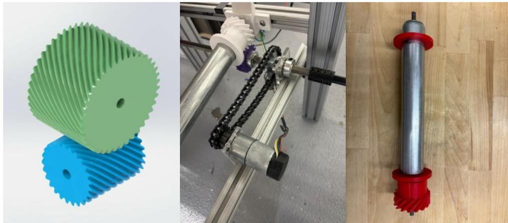
*Figure 33. Box conveyor parts and driving mechanism*
