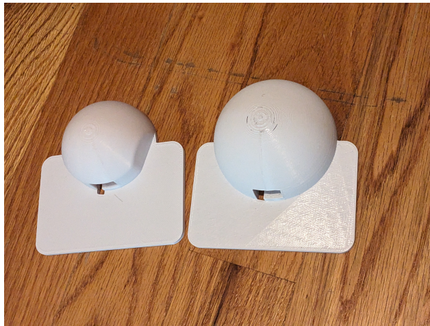
Figure 20: Palm rests for the miniaturized PCB view from the top.
