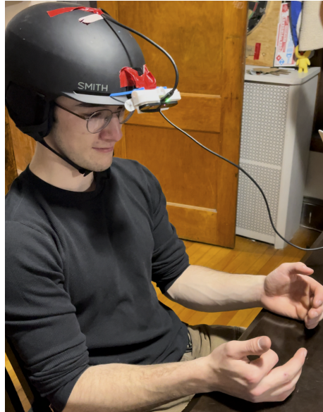
Figure 15: Leap Motion 2 mounted to a helmet for a VR view of hand movement.
