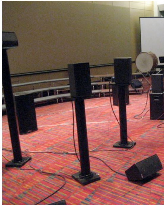
Photo 9: Speaker Stands of Different Heights Create High Frequency Instrument Depth Effect
