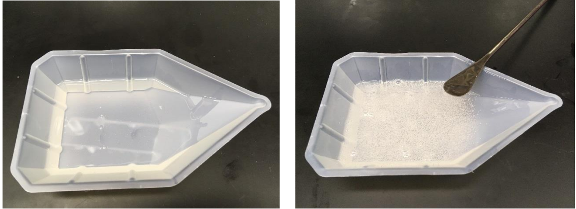
Figure 9 PDMS solution before mixture (left) and PDMS solution being mixed with a chemical spoon (right)
