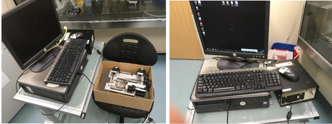
Figure 27 Left picture shows the entire stretching system. the right picture shows the computer and control box
