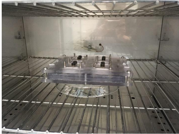
Figure 15 PDMS mold inside 70 Celsius oven. A cell culture dish is put beneath the mold to keep it leveled
