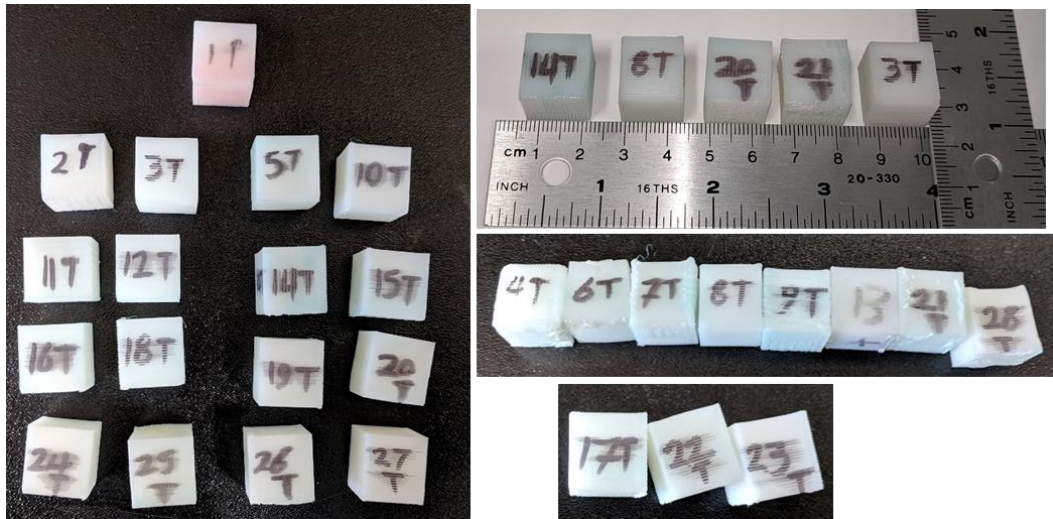
Fig. 61. The 28 cubical samples with size of 1.5×1.5×1.5 mm printed under different build parameters to measure the relationship between chosen parameters and density, contact quality, and SR.
