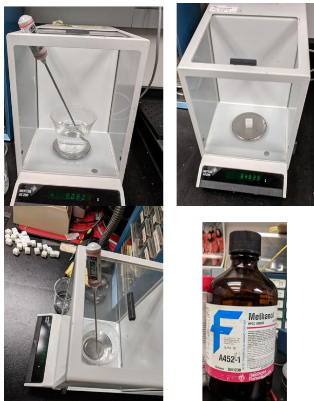
Fig. 63. The setup used for measurements of the density using the buoyancy forces: (a) the precise scale capable of measuring weight with 0.1 mg resolution; (b) the thermometer and the glass filled with Methanol to measure the weight of the cubes and their buoyant weights, and (c) the 99.9% Methanol manufactured by Fisher.
