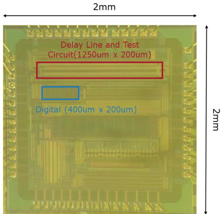
Figure 6.5: Chip Micrograph of Proposed DLL
