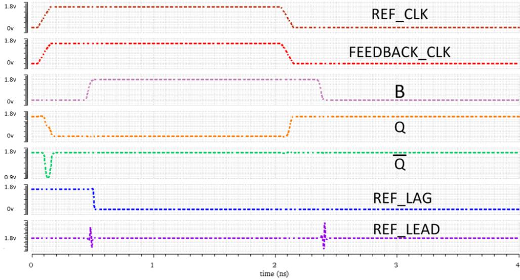
Figure 5.12: Simulation Result When Reference CLock Leads 0.1ps
