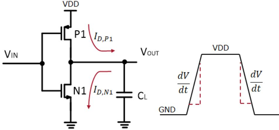
Figure 2.7: Schematic of Inverter
