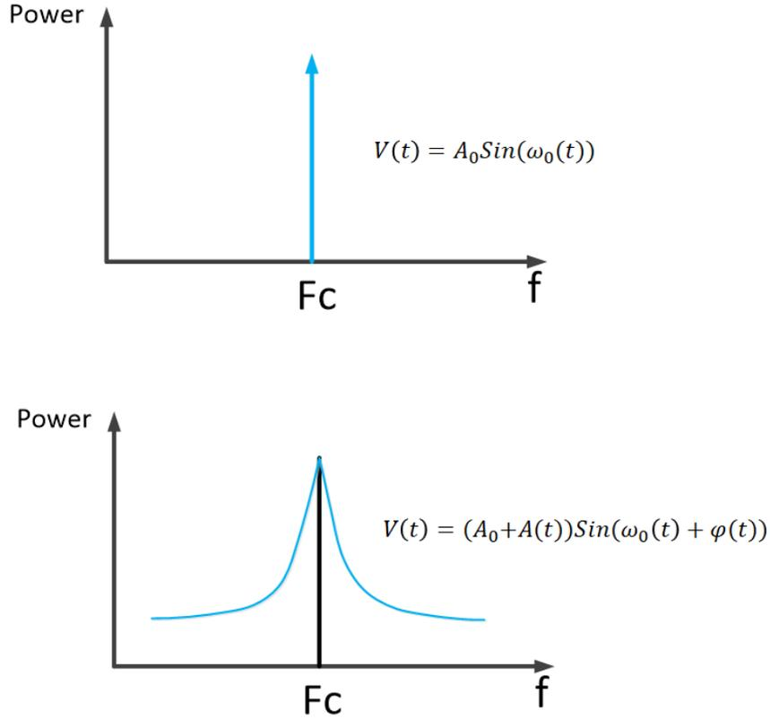
Figure 2.3: Jitter in Frequency Domain - Phase Noise
