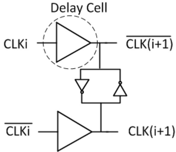
Figure 3.5: Schematic of Single Delay Stage.
