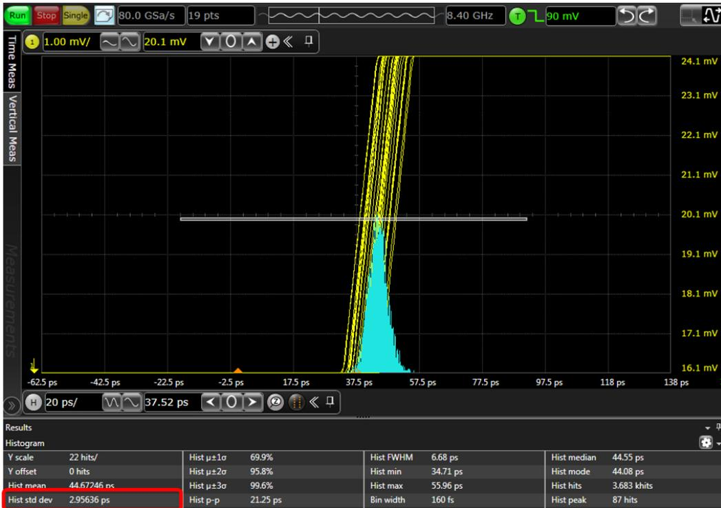
Figure 4.9: Measured jitter of 1st stage,  $\sigma=2.95636\text{ps}$
