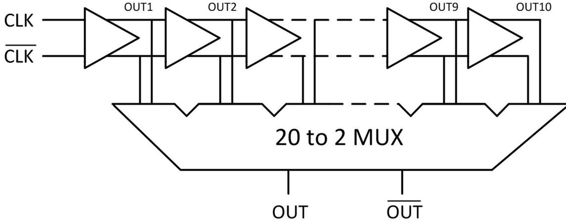
Figure 3.1: System design of the test chip
