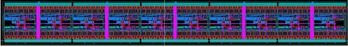
Figure 3.4: Zoom in layout of the delay line
