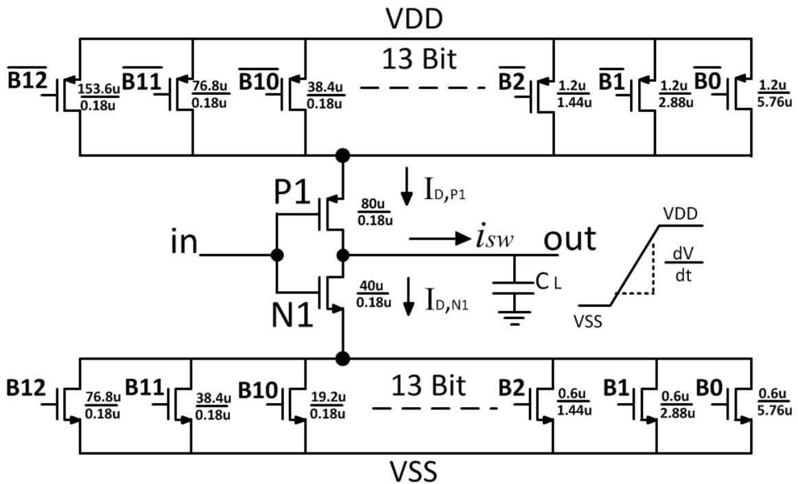
Figure 3.6: Schematic of Single Delay Cell.
