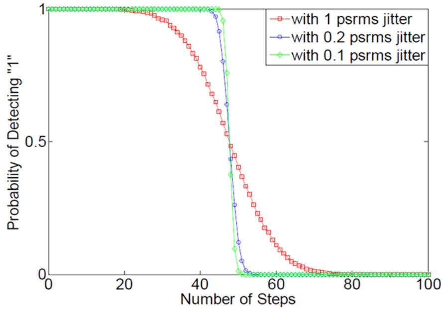
Figure 5.15: Probability of detecting “1” with different value of jitter
