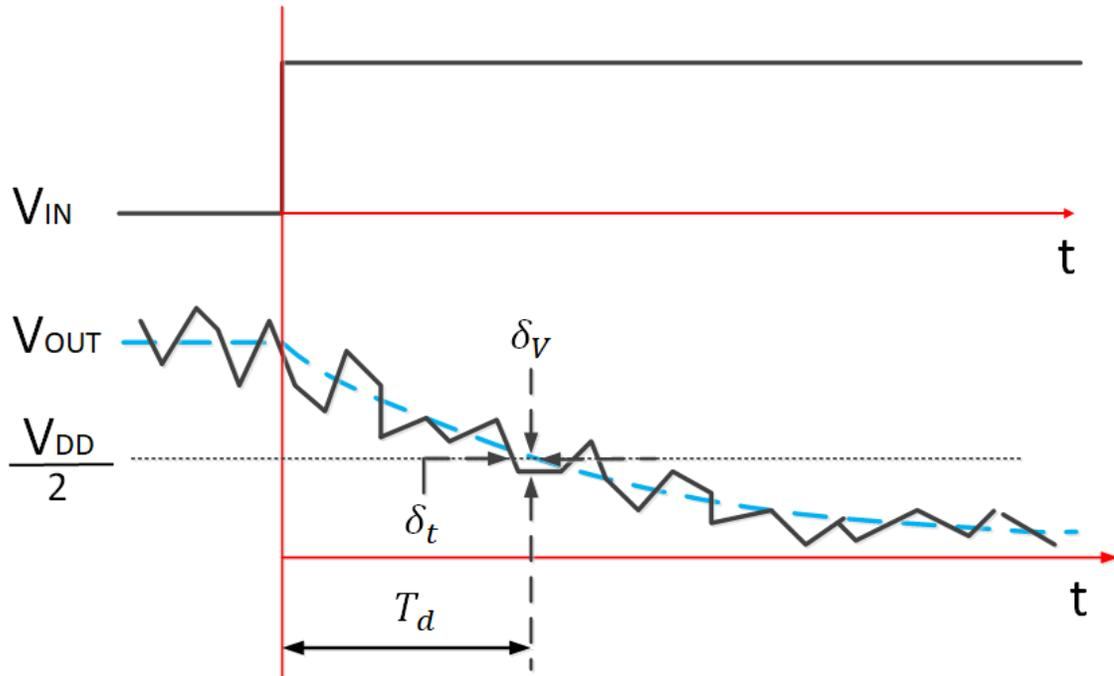
Figure 2.9: noise waveform of inverter
