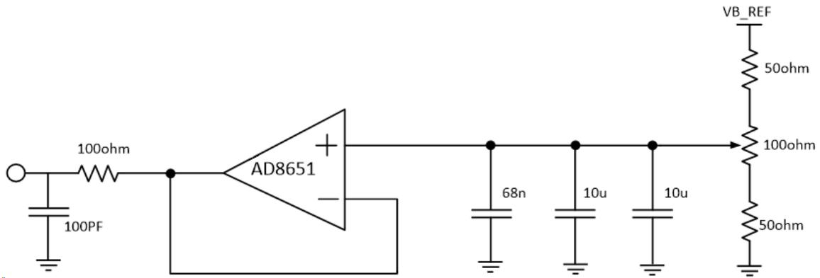
Figure 4.4: Schematic of the 0.9v reference voltage generation circuit
