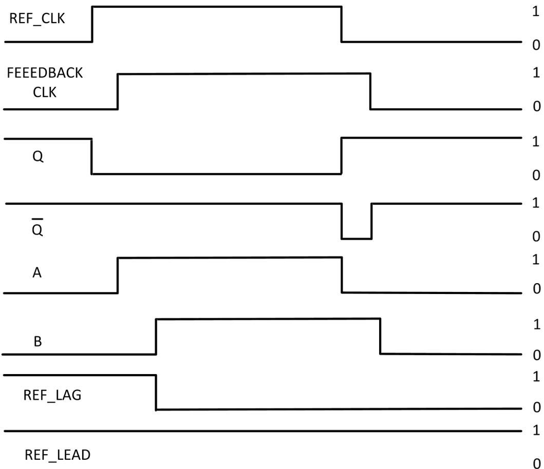
Figure 5.8: Timing Diagram of Proposed BBPD
