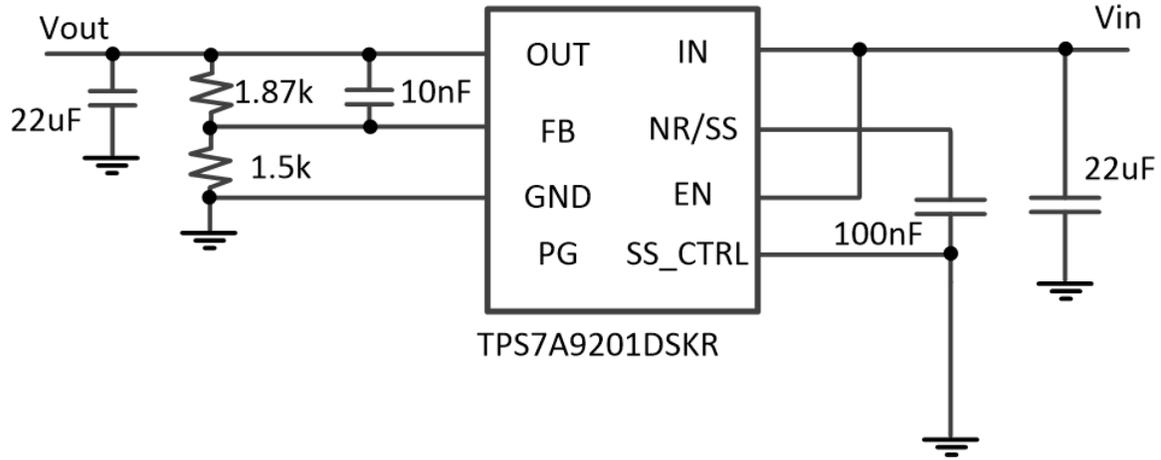
Figure 6.3: Schematic of the Low Dropout Voltage Regulator
