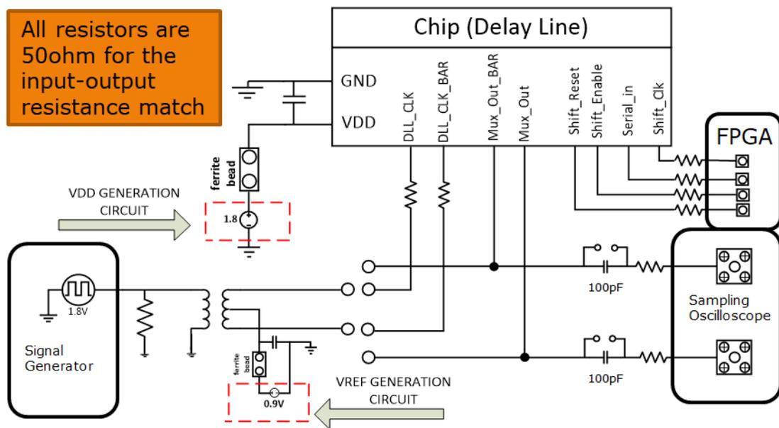
Figure 4.1: System Level Printed Circuit Board Design
