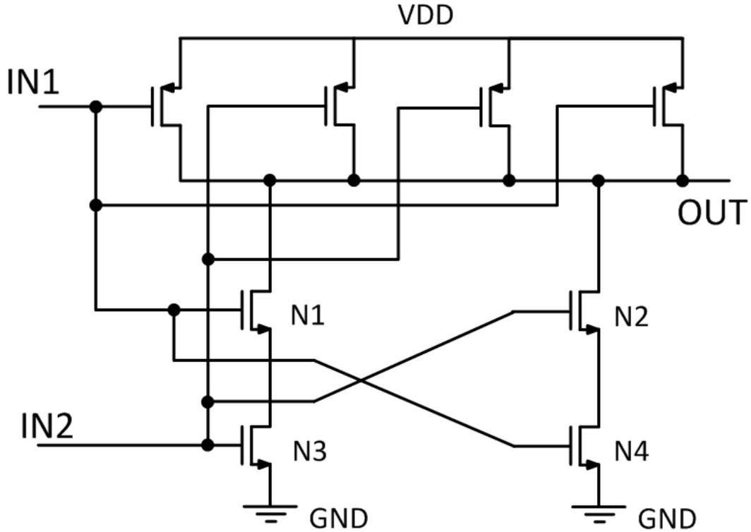
Figure 5.10: Schematic of Proposed Symmetric NAND Gate
