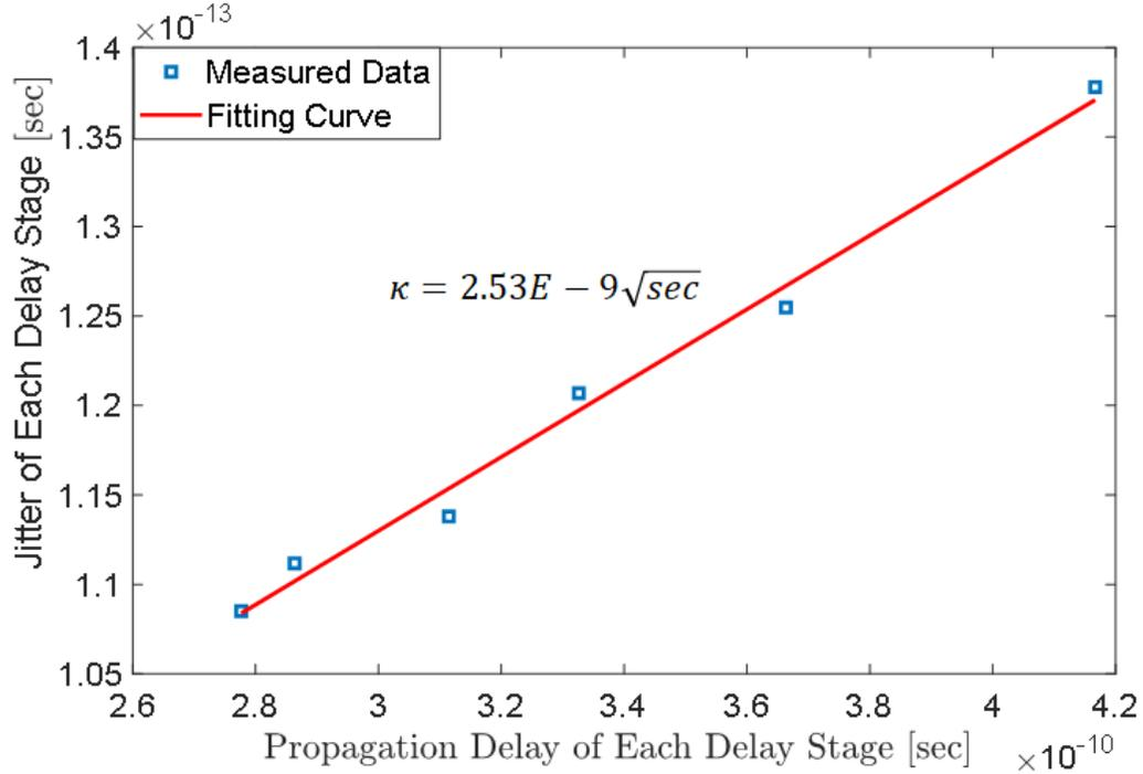
Figure 6.10: Measured Jitter When Propagation Delay Change,  $I_{PEAK}=4.2\text{mA}$
