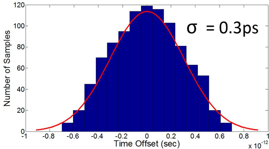
Figure 5.11: Monte Carlo Simulation for Proposed Bang-Bang Phase Detector
