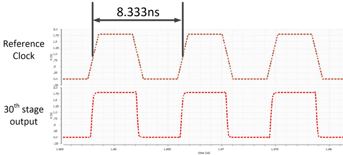
Figure 5.19: Simulation of Low Jitter Delay-Locked Loop
