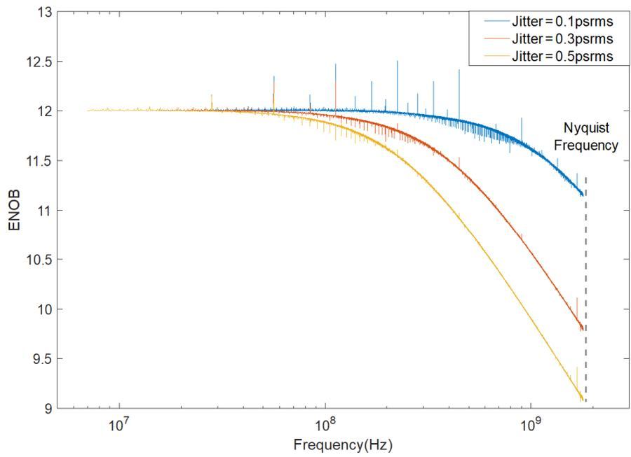
Figure 5.4: ENOB vs Input Signal Frequency,  $f_s = 3.6\text{GHz}$
