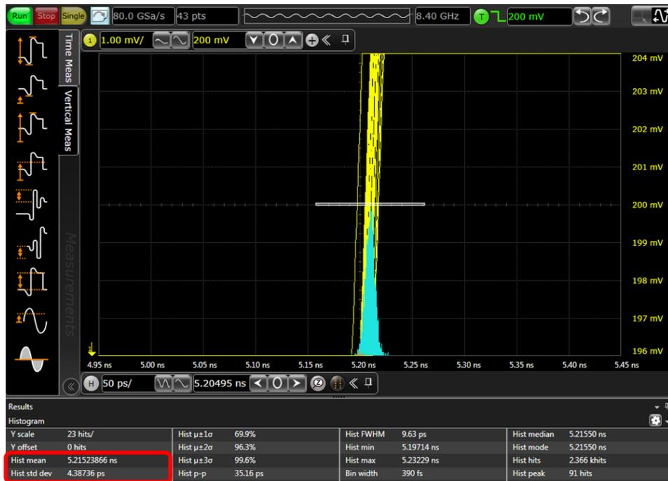
Figure 6.8: Jitter of Low Jitter Delay-Locked Loop 20th Output: 4.38736 psrms
