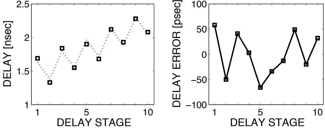
Figure 4.7: (a) Propagation delay of each stage ( $n_{CTL} = 1024$ ) (b) Nonuniformity of stage delay in psec
