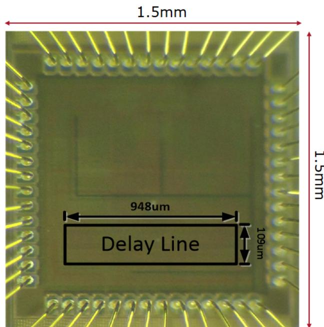
Figure 4.5: Chip Micrograph of Low Jitter Delay Line.
