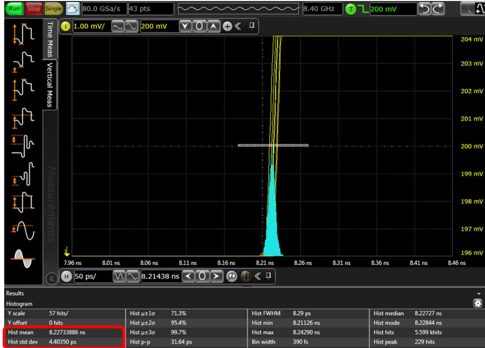
Figure 6.9: Jitter of Low Jitter Delay-Locked Loop 30th Output: 4.40350 psrms
