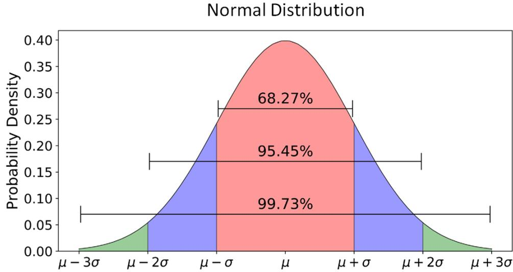
Figure 2.4: Normal Distribution of Random Jitter: probability of a large amount of random jitter is small, but not zero.
