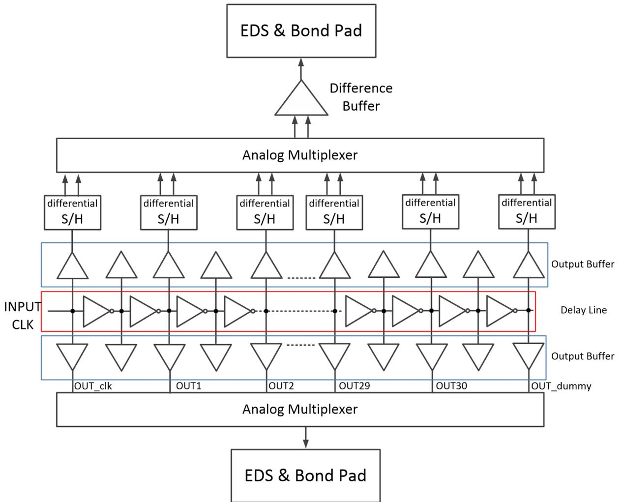
Figure 5.20: Block Diagram of Delay Line Test Circuit
