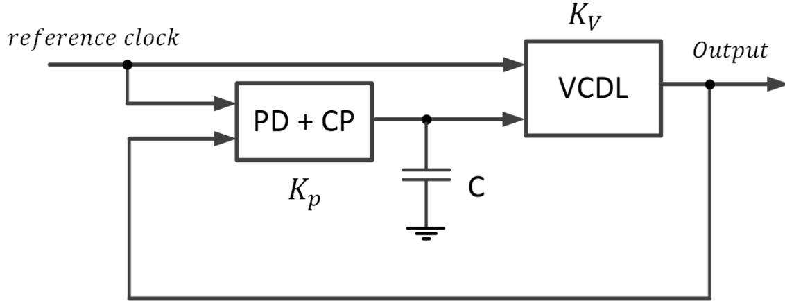
Figure 2.13: Block Diagram of Delay Locked Loop
