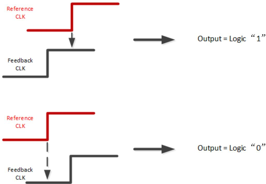
Figure 5.5: Output of Bang-Bang Phase Detector in different cases
