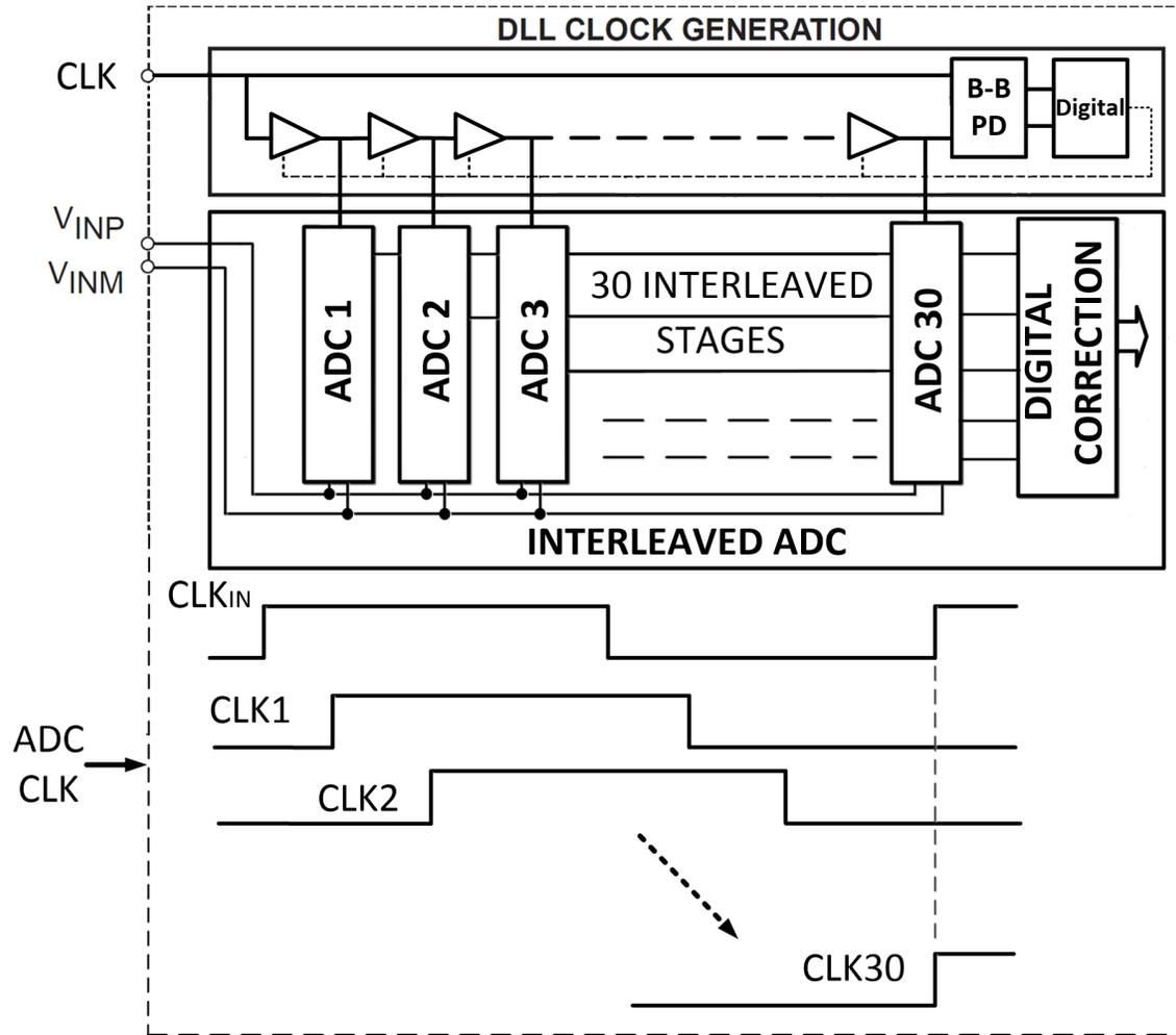
Figure 2.14: System Block of Time Interleaved ADC
