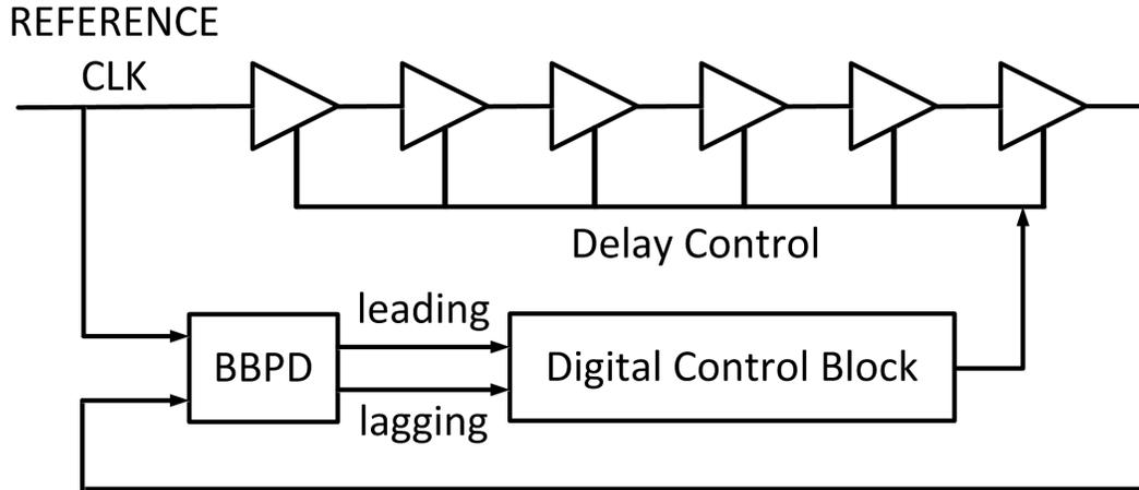
Figure 5.6: System Block Diagram for BBPD application.
