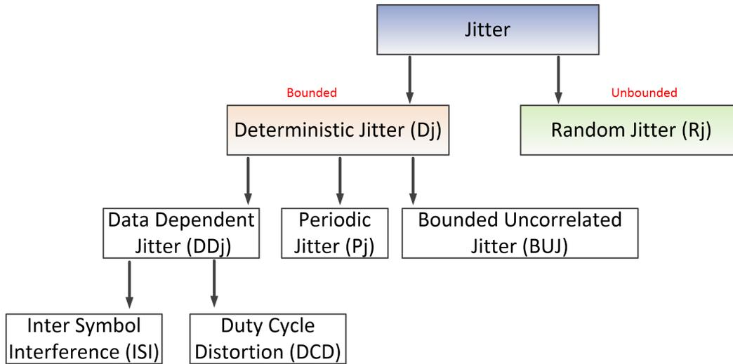
Figure 2.1: Jitter Component Classification Tree
