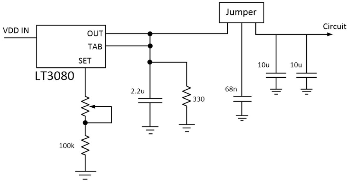
Figure 4.3: Schematic of the regulator on PCB (resistor unit is Ohm, capacitor unit is Farad)
