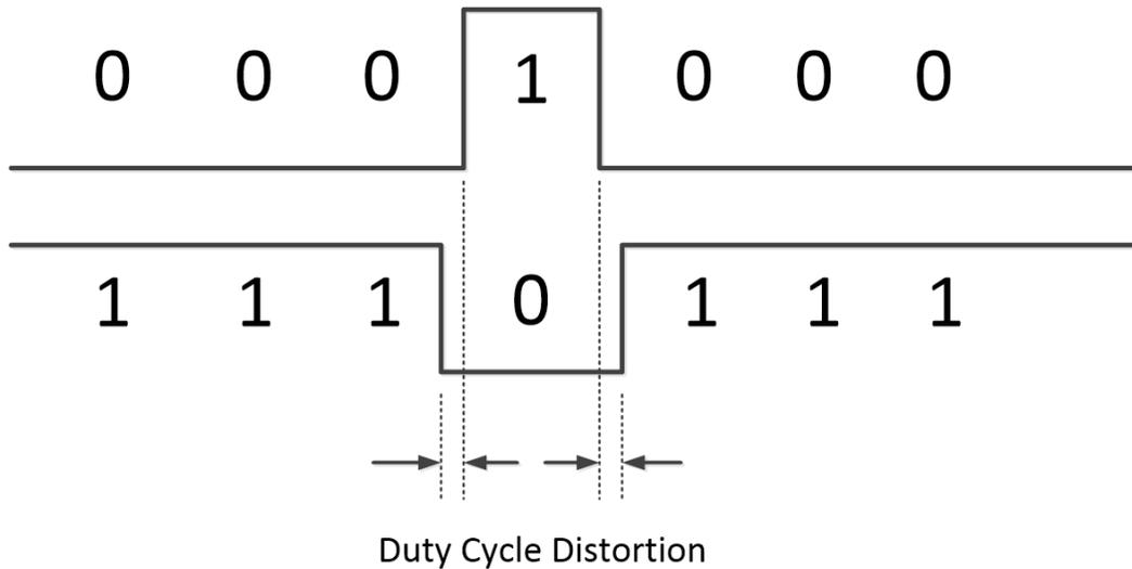
Figure 2.6: Duty Cycle Distortion Example
