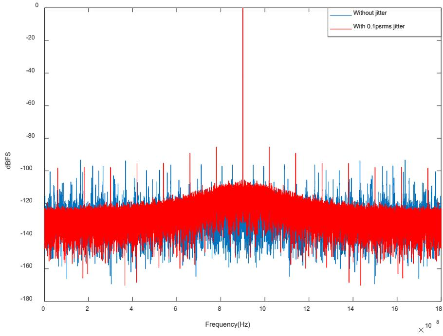
Figure 5.3: FFT of ADC output with/without 0.1 psrms jitter
