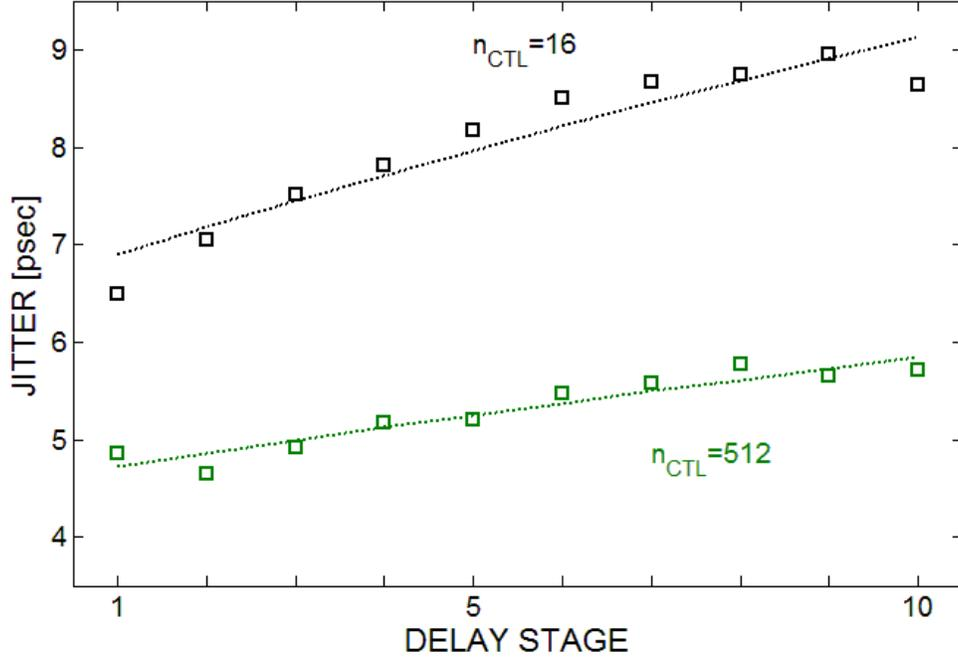
Figure 4.8: Jitter of the Clock under different Digital Control Code
