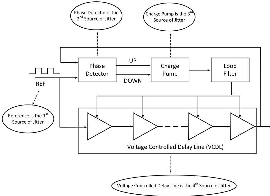
Figure 5.2: Jitter Source of Traditional Delay-Locked Loop [92]
