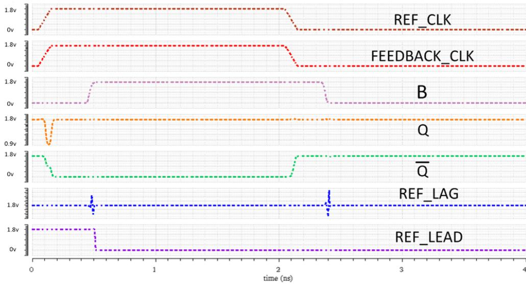
Figure 5.13: Simulation Result When Reference Clock Lags 0.1ps
