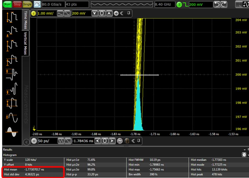
Figure 6.6: Jitter of Input Reference Clock Source: 4.36321 psrms
