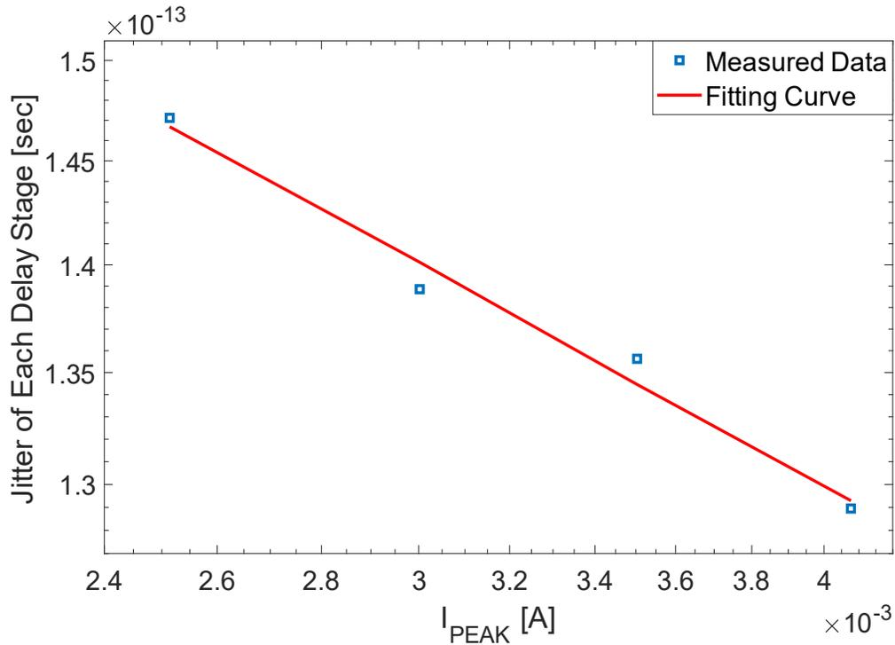
Figure 6.11: Measured Jitter when  $I_{PEAK}$  change.  $t_{PD} = 10\text{ns}$
