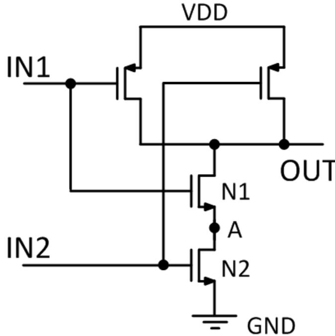
Figure 5.9: Schematic of traditional NAND Gate
