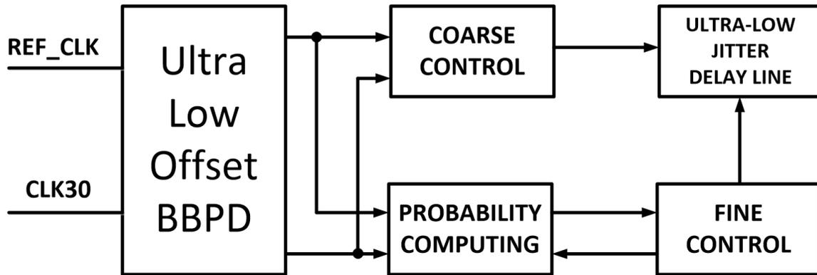
Figure 5.1: Low Jitter Delay-Locked Loop System Diagram
