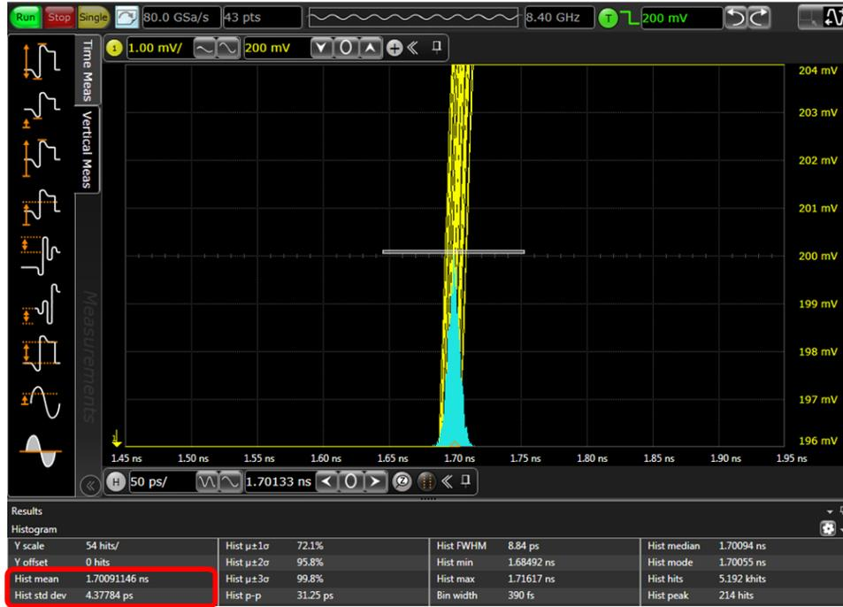
Figure 6.7: Jitter of Low Jitter Delay-Locked Loop 10th Output: 4.37784 psrms
