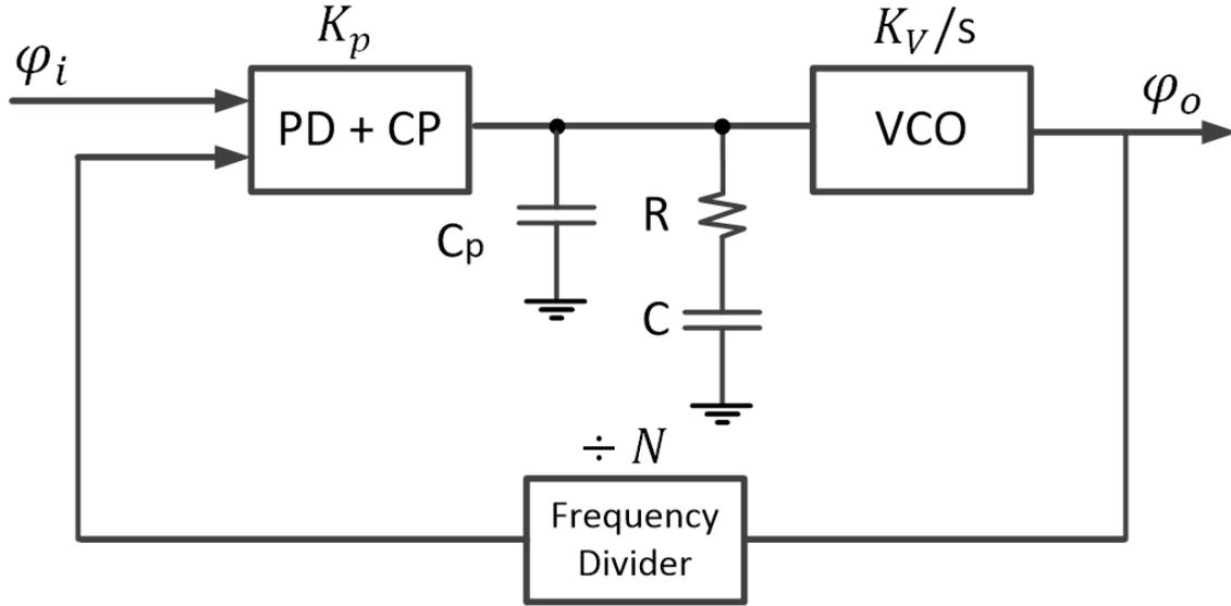
Figure 2.12: Block Diagram of Phase Locked Loop
