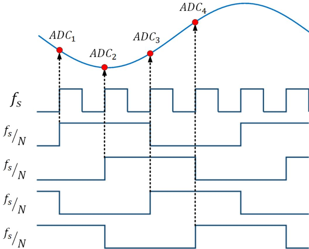
Figure 2.15: Example of Time Interleaved ADC. The sample rate of each sub ADC is  $f_s/N$ , the final sampling rate of the time interleaved ADC is  $f_s$ . In the example,  $N = 4$
