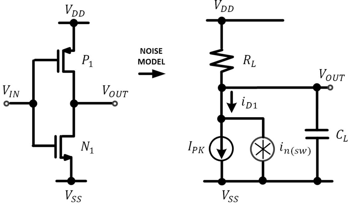
Figure 2.11: Switching element noise model of single ended inverter
