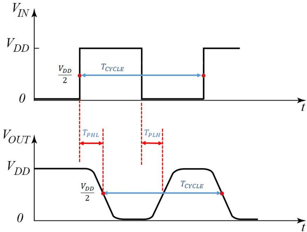
Figure 2.8: Propagation Delay of Inverter
