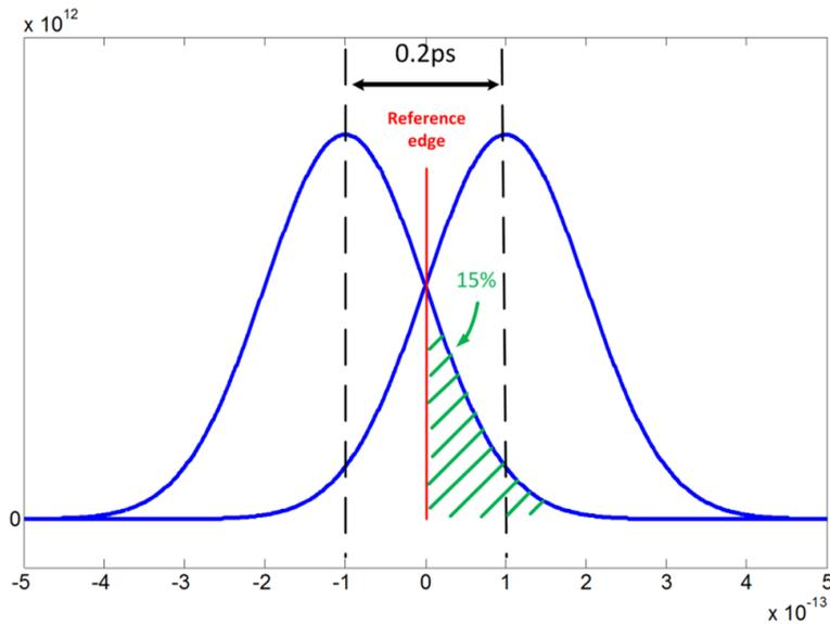
Figure 5.16: With 0.2ps step resolution,  $15\% < p\{1\} < 85\%$  can be considered as the DLL lock condition
