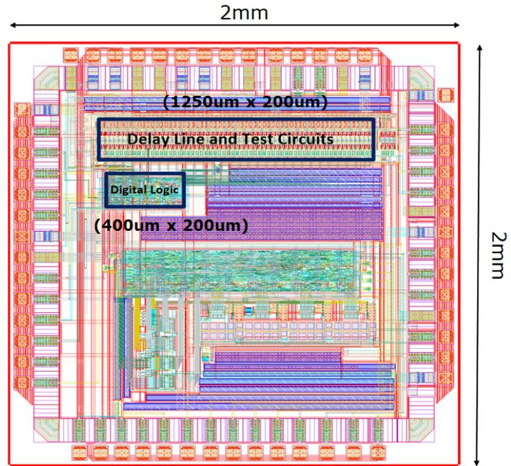
Figure 6.4: Chip Layout of Proposed DLL
