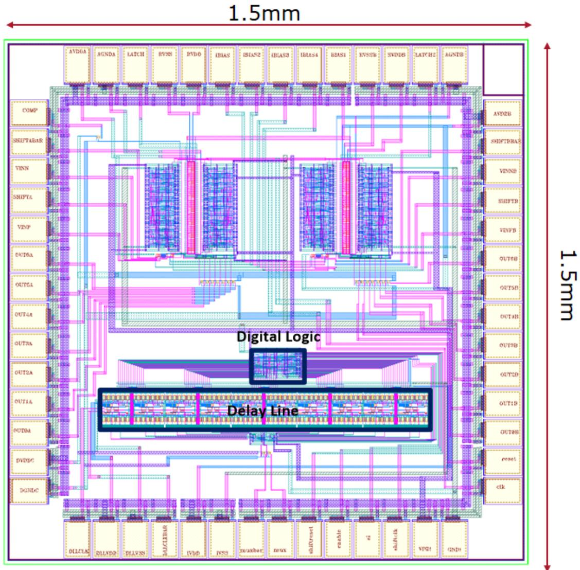
Figure 3.3: Layout of the Low jitter Delay Line
