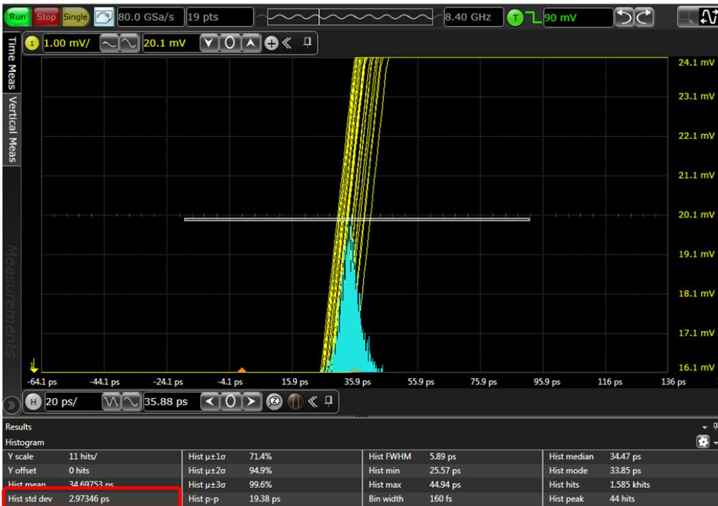
Figure 4.10: Measured jitter of 10th stage,  $\sigma=2.97346\text{ps}$
