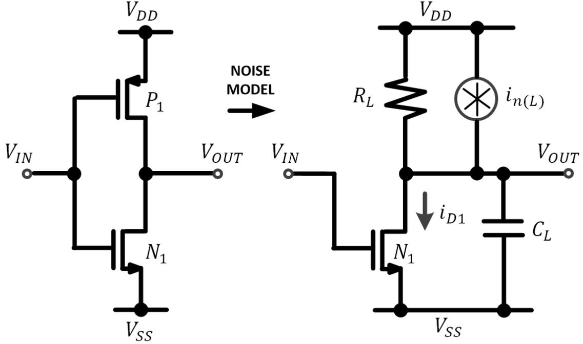
Figure 2.10: Load resistance noise model of single ended inverter
