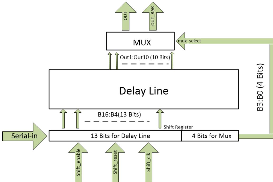
Figure 3.2: Digital control block diagram of chip
