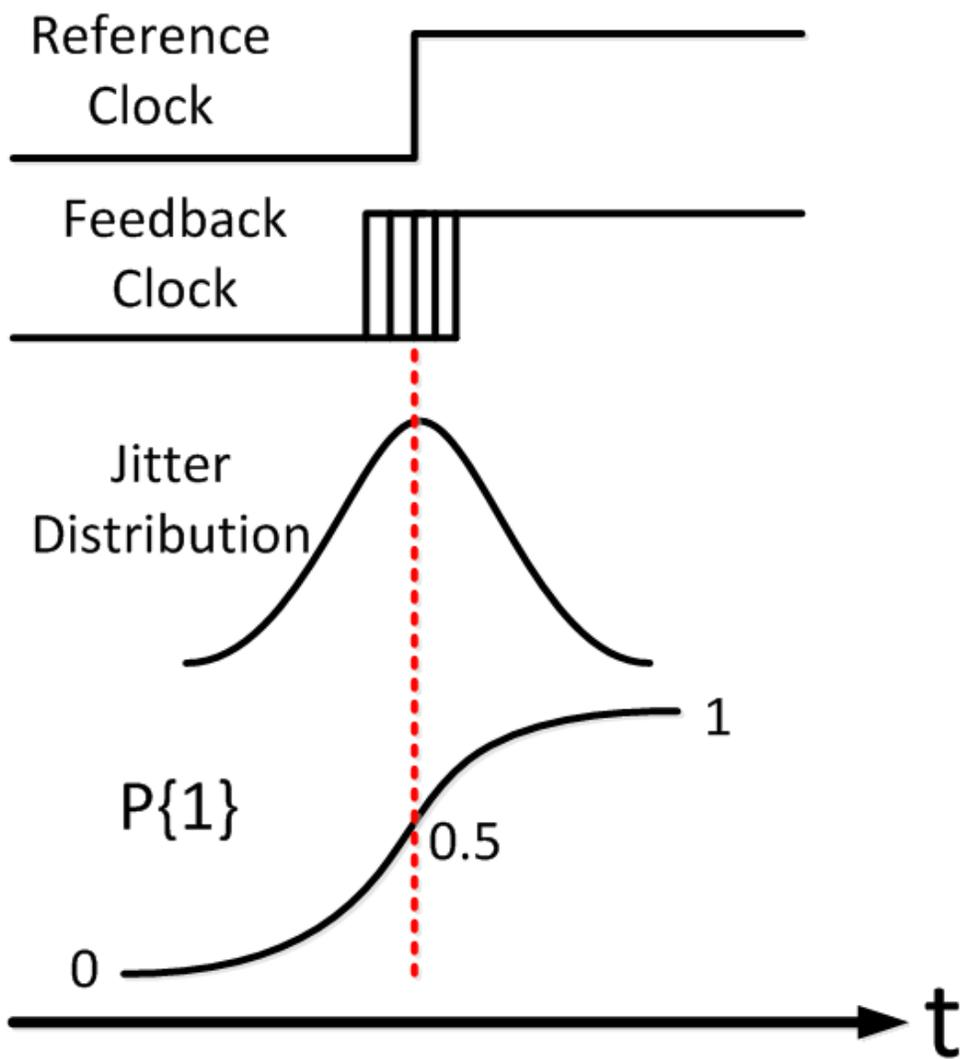
Figure 5.14: Probability Problem in Bang-Bang Phase Detection with Random Jitter Clock
