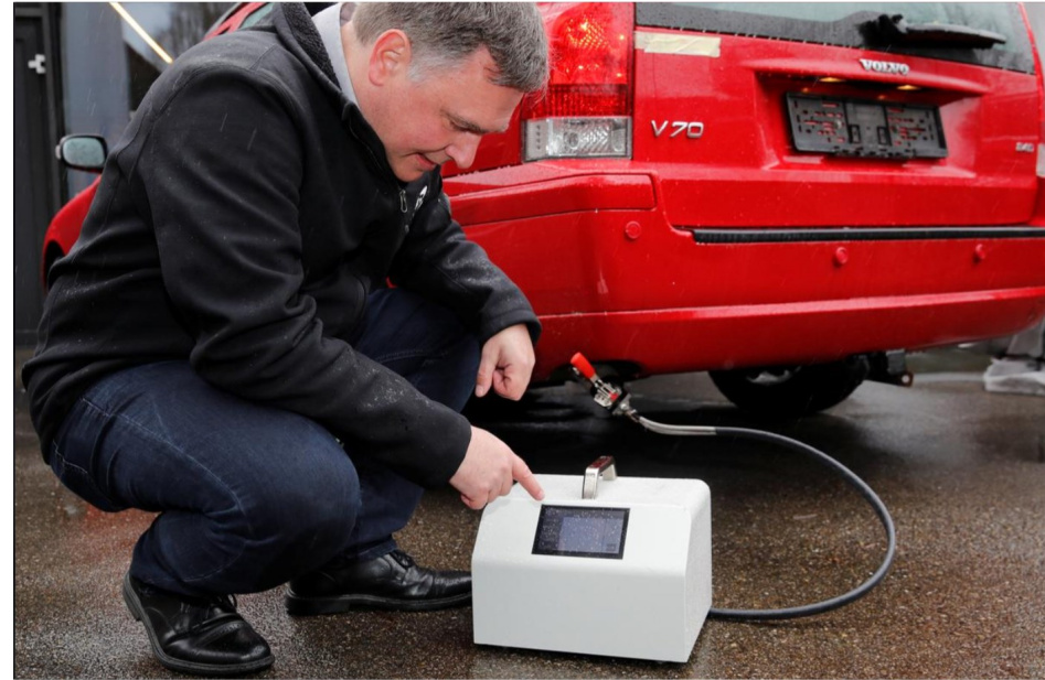
Figure 11: TSI PET being used in an emissions test
