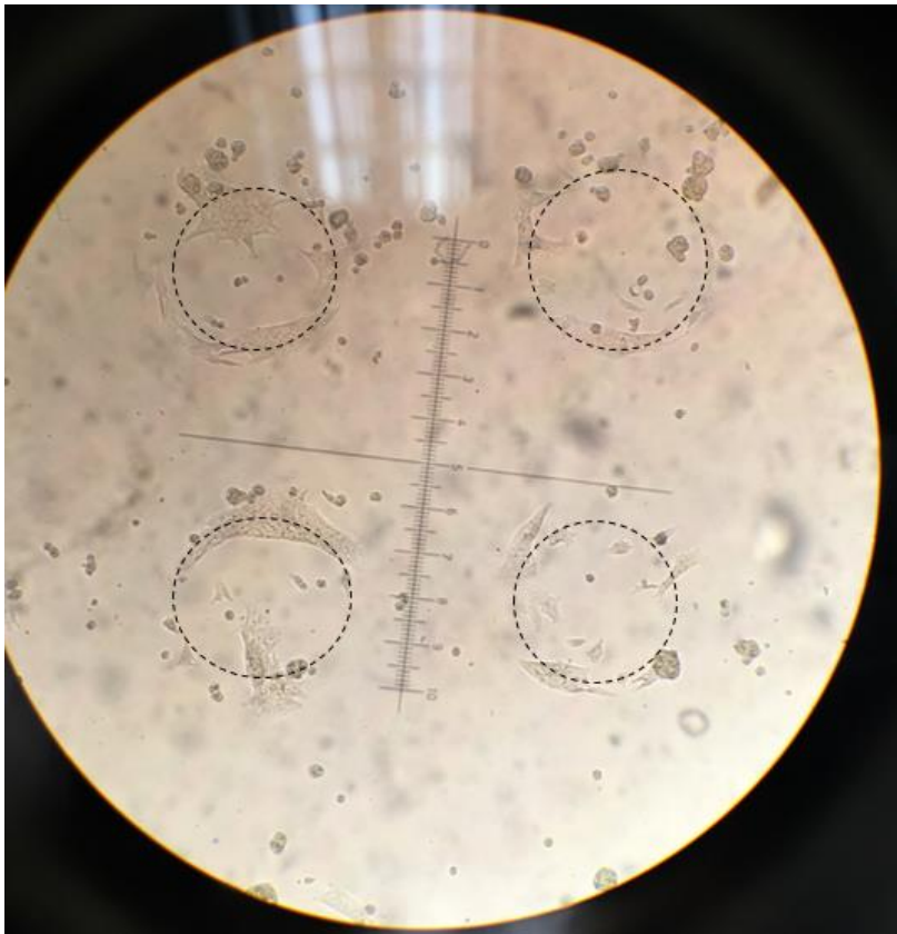
Figure 3: The initial protocol for indirect microcontact printing produced ring-like patterns when confluent circles should have been produced.
