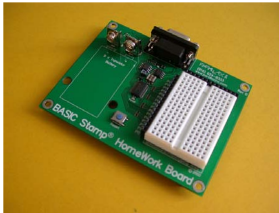
Fig. 4.8. Microcontroller evaluation board utilized in the developments. The surface mount microcontroller package is located at the center of the board (Parallax, 2003a).
