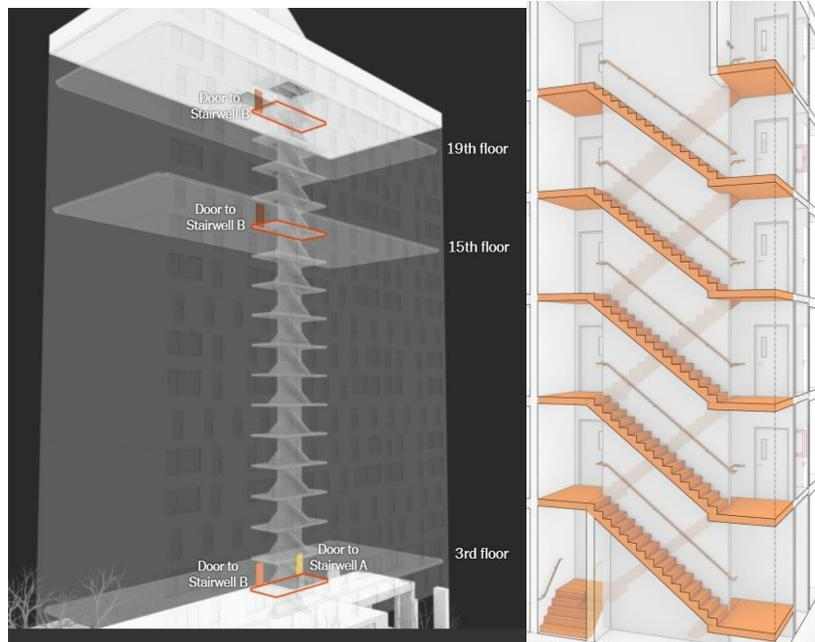
Figure 2: Scissor Stairwell Layout (Source: NYT and Speckert, nd.)
