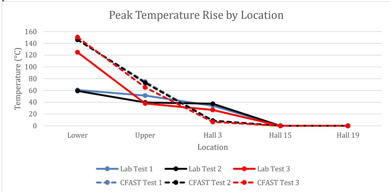
Figure 23: Peak Temperature by Location
