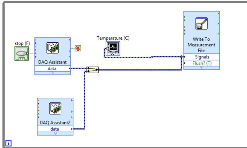
Figure 13: The LabVIEW block diagram for obtaining temperature from our thermocouples.
