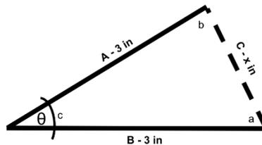
The door percentage input into CFAST was calculated at each different degree opening by taking the ratio of C to B. We used the law of sines to calculate the third side (C).
