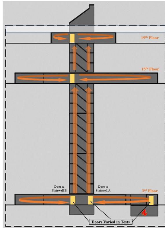
Figure 5: Key areas where smoke spread in the Bronx Apartment building
