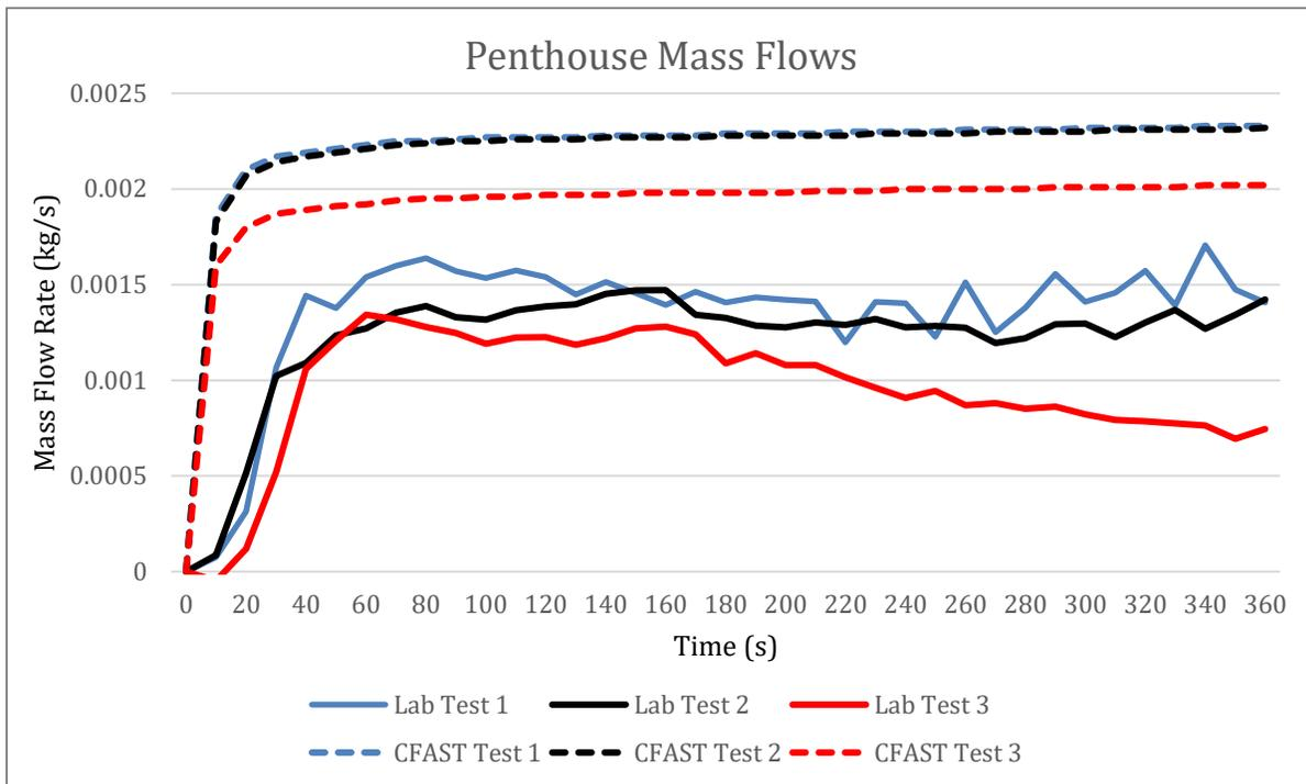
Figure 27: Mass Flow at the Penthouse
