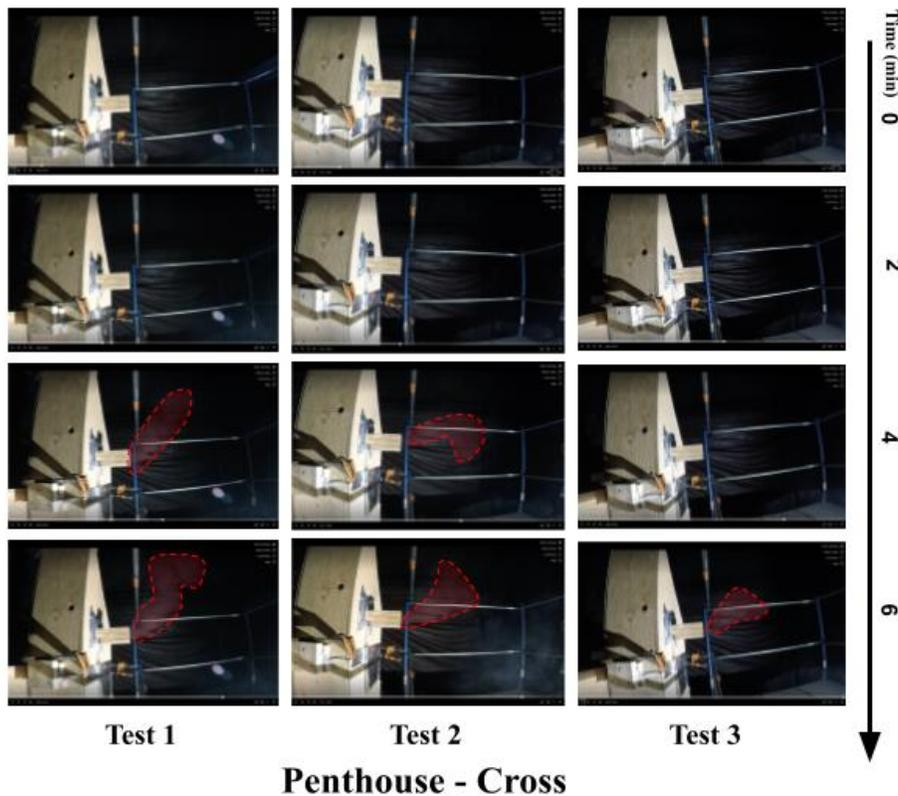
Figure 29: Penthouse Smoke Exhaust Comparison between All Tests
