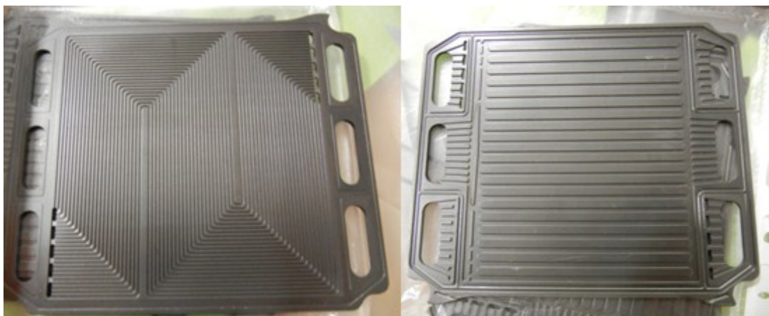
Figure 22: (left) A) Bipolar Plate reactant distribution channels and (right) B) hot water distribution channels (UBzM, 2012)
