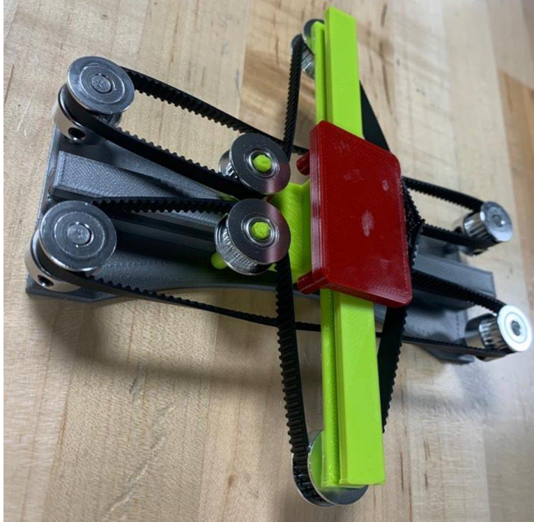
Figure 38: Inverted H-Bot assembly with pulley and belt configuration
