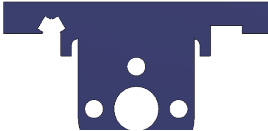
Figure 63: Print bed with cutouts for Delrin strips and Delrin pre-loads
