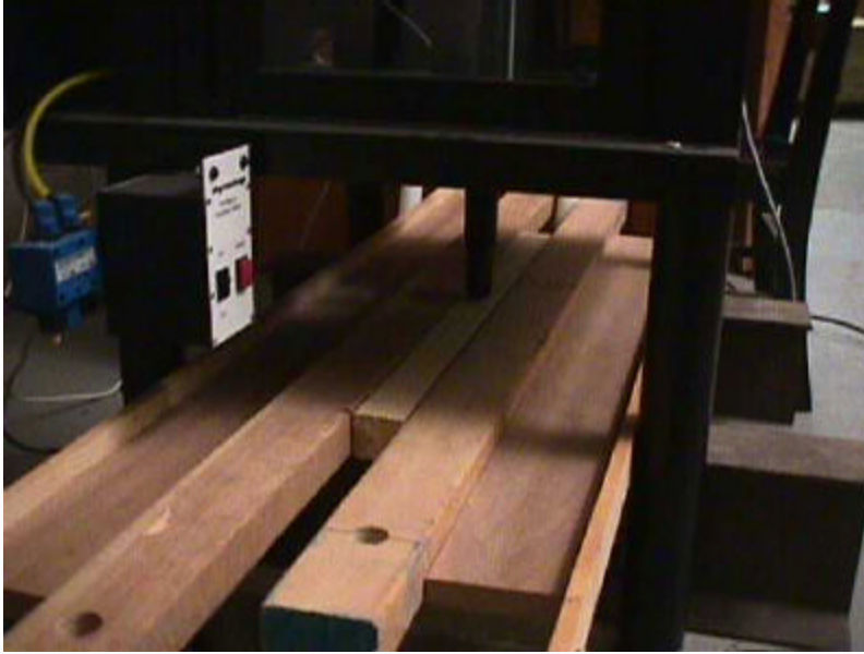
Figure 5. The wood support on each side of the specimen.
