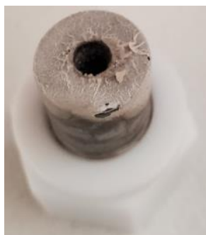
Figure 41. Dried KOH on outside of Oxygen cathode after discharge program
