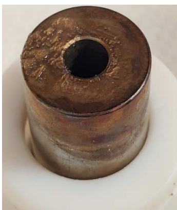
Figure 42. Gelled KOH accumulate from seeping through separators
