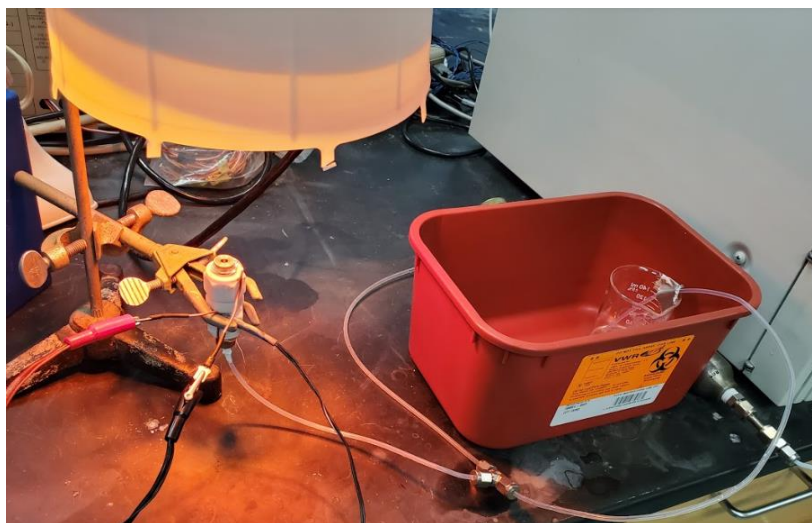
Figure 37. Nitrogen Sparge and Limited Air Flow Set-up
