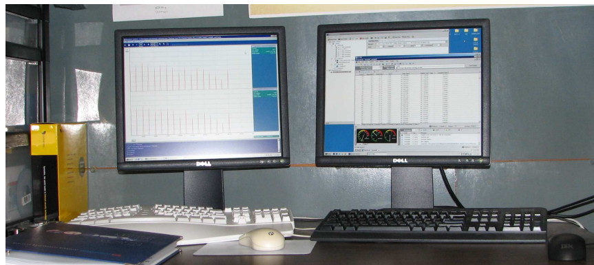
Figure 3-14 The multipath testbed control terminal; the screen on the left is for controlling the PROPSim™ C8 and the screen on the right is for controlling the Azimuth™ Systems 801W, modules, etc.
