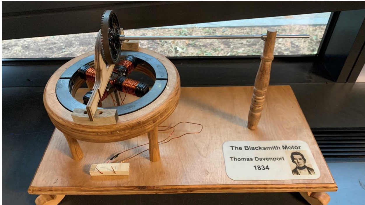
Figure 33: Image of motor with first iteration of permanent magnets. The frame is the same as in iteration 2 – only the field magnets changed. This version also features a new power supply setup.
