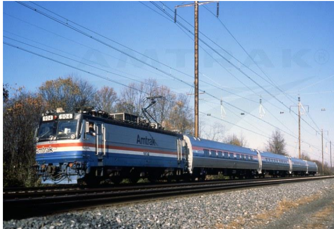
Figure 9: An Amtrak AEM-7 Pulling four cars. The AEM-7 is an electric locomotive featuring a 7000hp drivetrain with a top speed of around 125mph. The electric train was one of Davenport's imagined applications of his electric motor. ( https://history.amtrak.com/blogs/blog/digging-into-the-archives-the-aem-7-locomotive )
