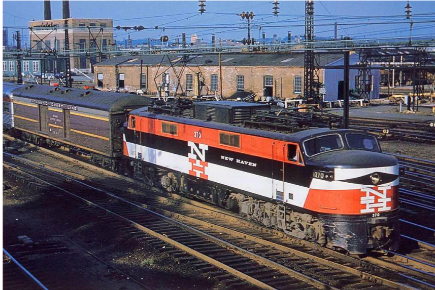
Figure 8: A New Haven EP-5 “Jet”. These electric locomotives would operate between New York and New Haven from the early 1950s through the 1970’s. At the time, the electrified line was revolutionary, and the New Haven was one of the first in its development. https://www.american-rails.com/ep5s.html
