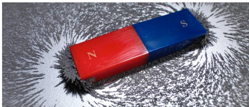
Figure 20: Example of a Permanent Magnet in the shape of a bar. Iron filings around the magnet follow the magnetic field lines.
