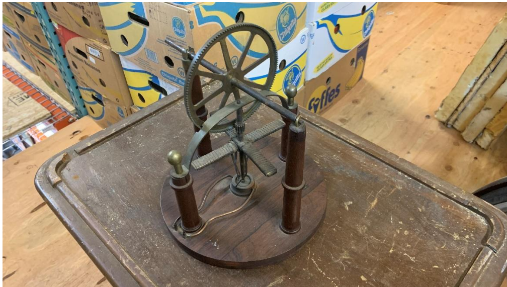
Figure 6: One of Davenport's original motors. Likely an early version based on the use of his Mercury cup commutator in at the base of the armature shaft. Not seen are the permanent field magnets which would rest on the supporting posts. For nearly 200 years old, the motor is in excellent shape. It is one of a handful known to currently exist and is currently part of a private collection.
