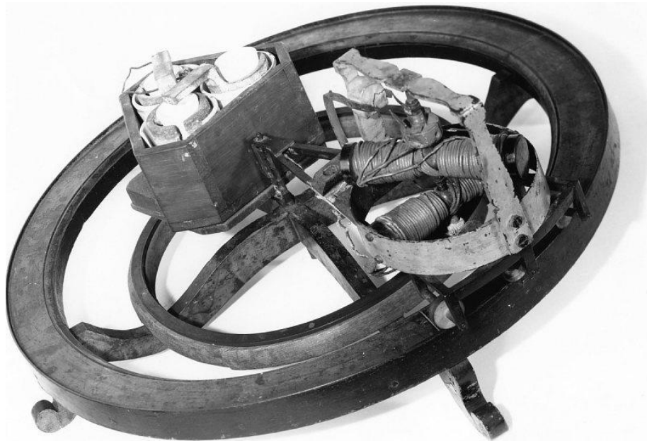
Figure 4: Image of the Davenport Model Railway. The little cart would be propelled around the circular track at “great speed” by the motor.
