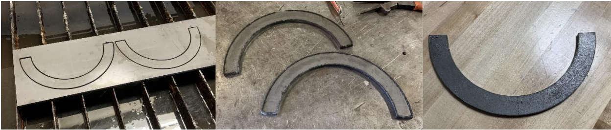
Figure 35: Image of cut semi-circles in plate and after finishing. The bur on the edge of the steel was removed by simply striking with a hammer (middle). The final product post cleaning (right)
