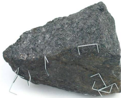
Figure 11: A piece of lodestone with staples attached. Lodestone (magnetite) has a naturally occurring magnetic field due to its high concentration of iron oxides.
