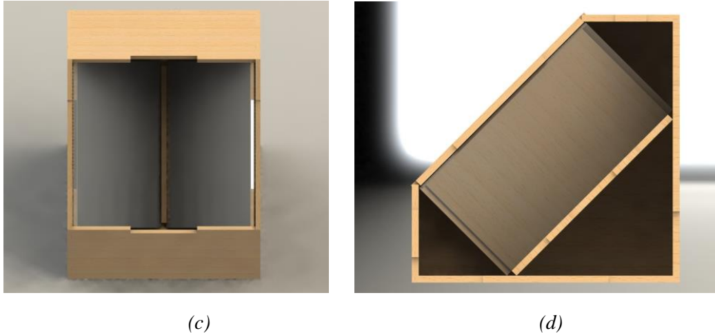
Figure 2.2 3D drawing of the mechanical structure of the foot box. (a) from the back; (b) from the front; (c) internal structure from the front; (d) internal structure from left side
